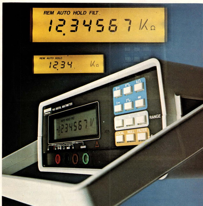
Extending scale length to 6½ digits via digital averaging, Model 7150 DMM incorporates full talker/listener IEEE-488 interfacing as a standard capability.
