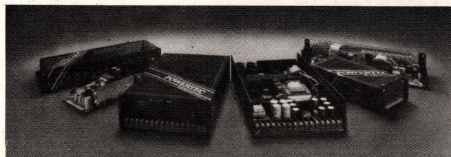
Fig 5—Featuring a fully regulated main output and optional regulation on the secondaries, Powertec's Series 19 ValuSwitcher line furnishes 50 to 300W and includes an optional EMI filter that meets VDE 0871 specifications.
