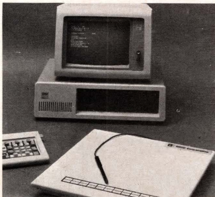
Equipped with an 11×11-in. digitizer pad and menu-driven software, the Graphic Analysis Package 1 from GTCO Corp costs $1419 and takes advantage of the processing and graphics of IBM's Personal Computer.
