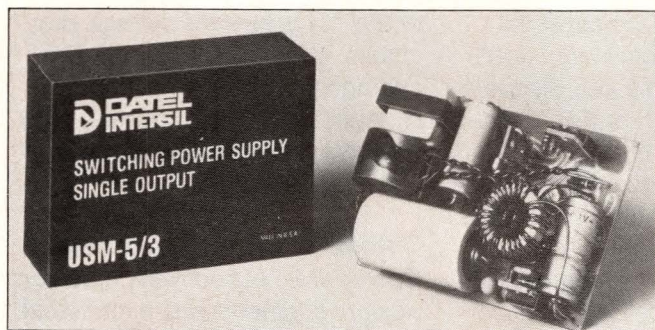
Monolithic switching regulators employ a push/pull pulse-width-modulation technique operating at 20 kHz min to ensure silent operation of Datel-Intersil's 5V, 3A Model USM-5/3. The unit accepts line voltages of 90 to 130V ac at 47 to 450 Hz and costs $119.
