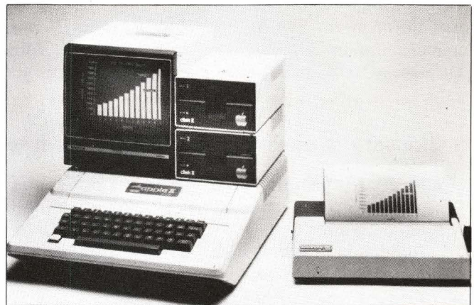
Termed the Apple Disk II housekeeper , the DOS 3.3 operating system from Apple Computer allows turnkey operation under Apple BASIC. It automatically catalogs files by name; saves, loads, runs, renames, deletes and verifies files; permits sequential and random data access; and helps make backup diskette copies.
