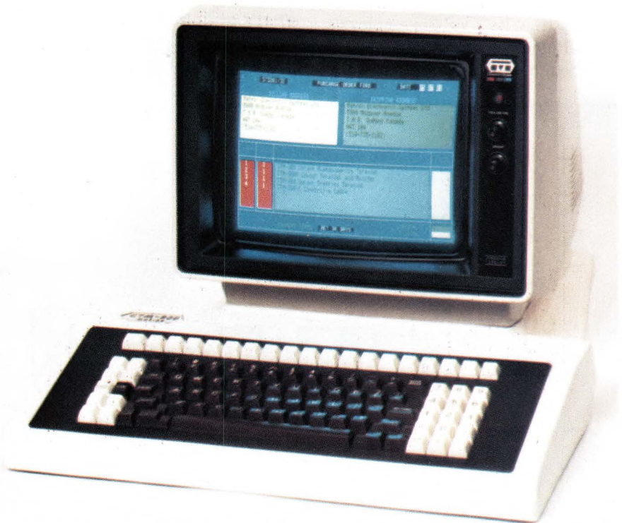
An RS-232C-interfaced ASCII terminal, the CTM-300 from Matrox Electronic Systems also features an 8-color CRT display. You can customize its functions from the host computer via a downloaded program.
