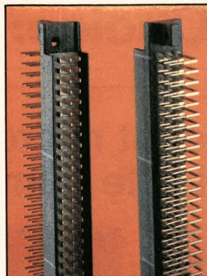
Three row VERSACON header. Available in 2-, 3-, and 4-row 0.100", 0.125", and 0.150" grid configurations.
