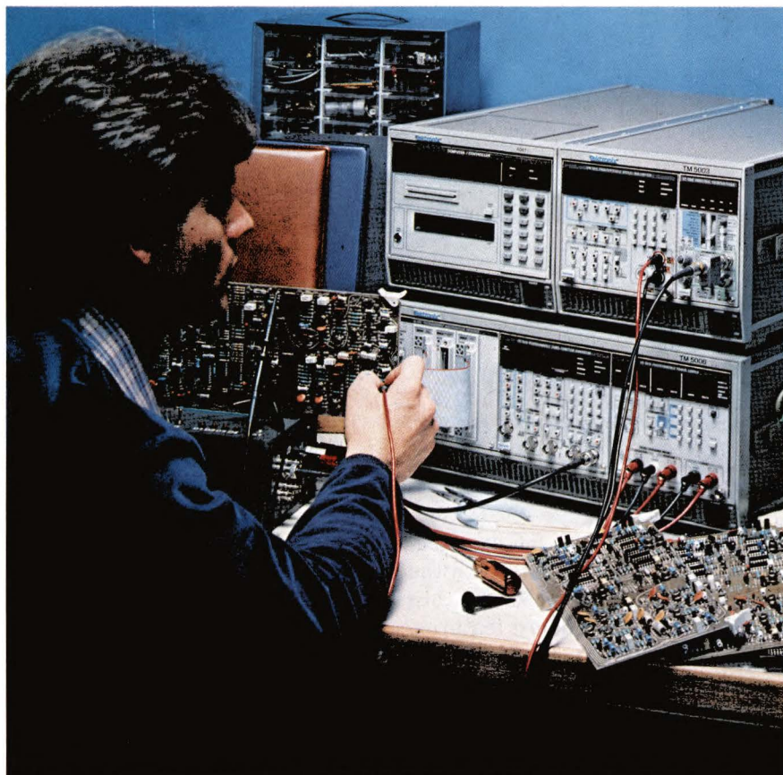
Among the various programmable plug-in instruments in Tektronix's TM 5000 Series, you'll find two counters: Models DC 5009 (135 MHz, $2200) and DC 5010 (350 MHz, $3600).
