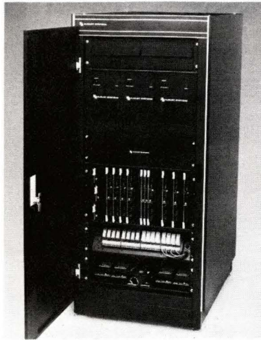
Employing advanced fault-tolerant technology to provide nonstop, error-free operation during a hardware failure, the Series 300 Can't Fail computer serves real-time control and monitoring applications where a failure could cause serious or catastrophic results.
