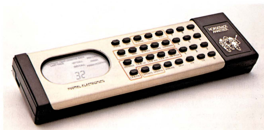
A sophisticated programmable machine requiring 31 inputs for each horse in a race, the Mattel Horse Race Analyzer includes an elaborate LCD that prompts the handicapper with the name of his next required entry.
