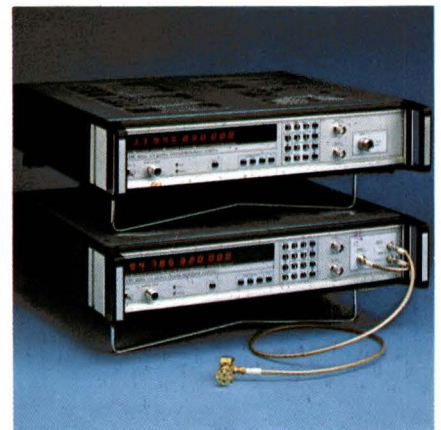
The highest frequency you can measure today with a frequency counter is 110 GHz, and you can measure it with EIP Microwave's Model 578. Models 575 and 578 feature source locking; they can control a swept source to achieve synthesizer-like performance at low cost.
