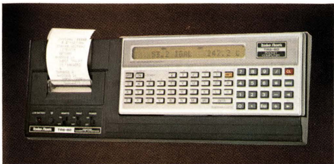
The printer cradle for the TRS-80 Pocket Computer also serves as an interface to a cassette recorder that preserves programs on tape or loads them into the machine.
