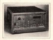
**BER INDICATOR.** Providing bit-error-rate measurements to 325 MHz, the modular BERTS-325C includes a clock source, transmitter and receiver that generate pseudorandom or fixed-word patterns for stimulating the system under test and measure the bit-by-bit errors received. BER or total errors can be measured on continuous or burst data for applications such as TDMA testing. Data and delayed-data outputs are furnished for QPSK-test applica-
