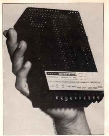
Taking advantage of the efficiencies available at higher frequencies, Abbott Transistor Labs' Model Z switcher runs at 38 kHz.
