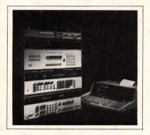
**TEST SET.** Model 8903-E85 semiautomatic transceiver test set makes in-channel tests from AM, FM and PM communication transceivers from 150 kHz to 990 MHz, either automatically under control of an HP 85F controller or manually using instrument frontpanel keyboard entry.
