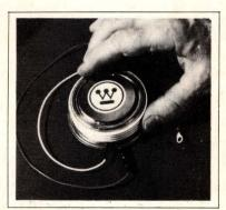
PHASE-CONTROL SCR. A phase-control thyristor that can handle up to 3500V and provide current ratings of 800 to 1200A, Model T9GO minimizes the need for series design in high-voltage circuits. Developed for motor and phase controls, VAR systems, power supplies and fusion systems, it provides guaranteed dv/dt of 300V/µsec. Forward voltage drop specs at 1.7V for the 1200A unit. Other features include gate current of 200A with soft gate control,
