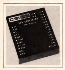
SYNCHRO CONVERTER. Employing Type II servo loops designed to follow input-shaft velocities as high as  $1800^{\circ}$ /sec (300 rpm), the 16-bit Model 168H100 synchro- or resolver-to-digital unit provides 1.3' accuracy over its full temperature range. It maintains this performance despite  $\pm 10\%$  signal- and reference-amplitude
