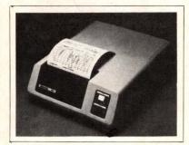
**HARD-COPY UNITS.** Models 4611 (for storage-tube displays) and 4612 (for raster-scan video sources) use a dry carbon toner and an electrostatic process to produce permanent copies on 8½×11-in. dielectric paper. The paper looks and feels like plain bond and permits pen or pencil notations.
