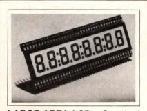
LARGE-AREA LCDs. Standard Model 740 (6-digit) and 742 (8-digit) displays feature bonded pin connectors. Both offer 0.5-in. character heights and include colons and decimal points. The displays operate over a 3 to 20V rms range and furnish low dissipation (50 µW typ for Model 740). Package sizes measure 2.75×1.2 and 3.7×1.2 in. for the 740 and 742, respectively. Connectorless versions are optional. Beckman Instruments Inc, Box 3579, Scottsdale, AZ 85257. Phone (602) 947-8371. Circle No 248
