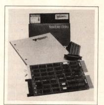
**PRINTER INTERFACE.** Model 125 single-board interface allows DEC LSI-11 systems to use any of the company's electrostatic plotters or printer/plotters, I/O multiplexers, hard-copy controllers or vector-to-raster converters. Plugging into the computer mainframe or I/O expansion chassis and operating
