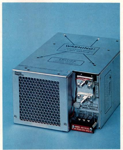
In a package that formerly provided 1000W, Model PM 2501 delivers 1500W. The 20-lb switcher comes with foldback and current limiting and furnishes a 20-msec hold-up period.
