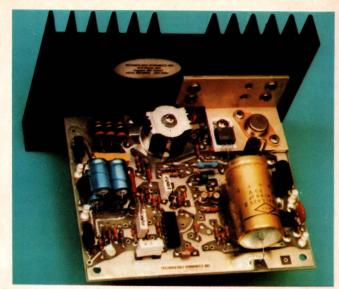
Switching regulators, such as Technology Dynamics' Model SR50P, can deliver 50W in a small package.
