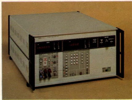
More than 80% of the Navy's needs for DVM and DMM calibration are met by a modified version of this Fluke Model 5100B.
