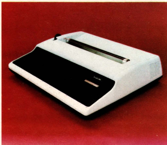
Equipped with dual 8085 \mu Ps and a 512-character receive-data buffer and achieving print rates from 30 to 120 cps, General Electric's Terminet 2000 Series printers suit desktop data-communication requirements.
