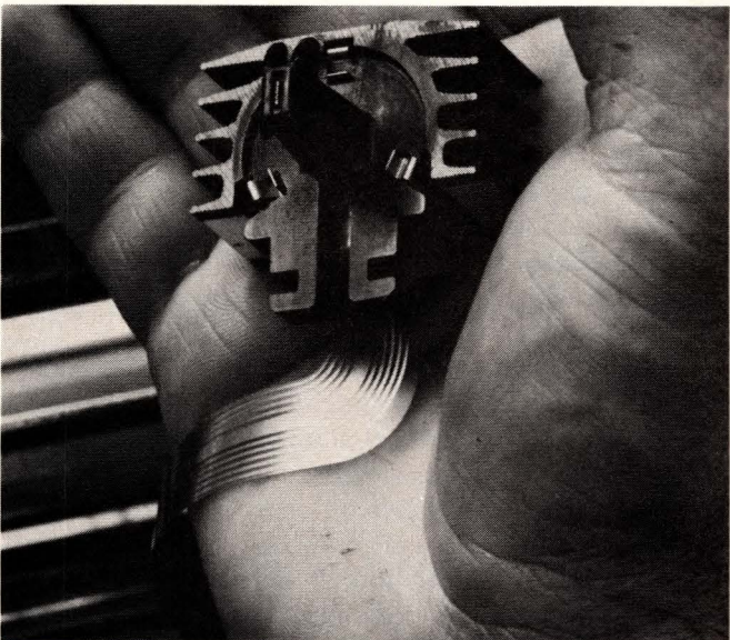
Designed as a low-cost ($28) throwaway replacement, this 9-wire single-column dot-matrix printhead is the heart of Epson's MX-80 tabletop printer.
