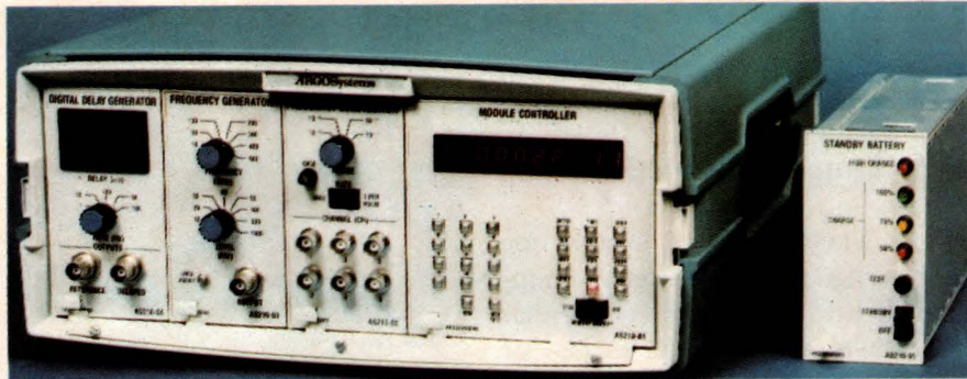
A rubidium standard is at the heart of ArgoSystems' frequency-counter calibration set. Its 10-MHz output goes to all the plug-ins in the portable mainframe.
