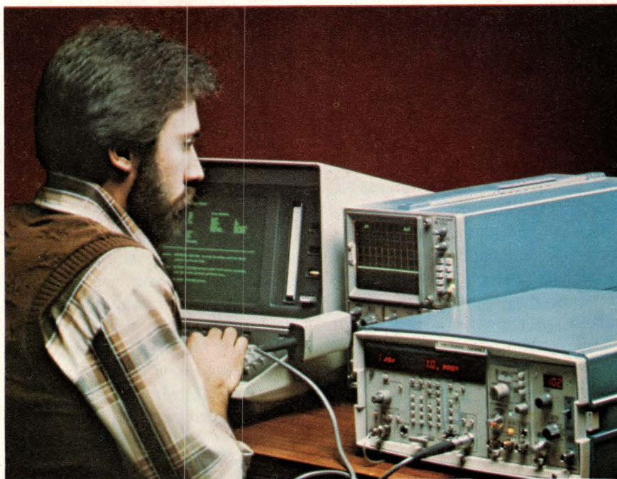
Prompting software helps you write calibration-procedure programs for Tektronix's Model CG 551AP scope calibrator.
