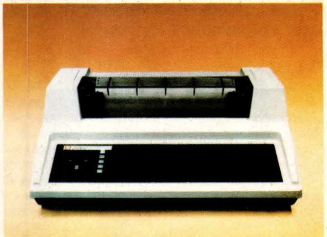
Offering such standard features as 150-cps print speed, 1280-character buffer, 132-column adjustable carriage and the ability to print as many as six copies, Texas Instruments' Omni 820 RO supports applications requiring flexibility as data-processing requirements grow.
