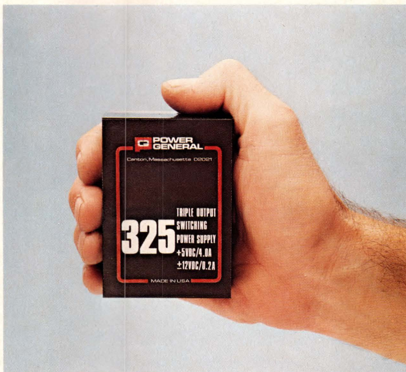
Offering a 25W rating in a 2.75×4×1.375-in. package, Model 325 delivers 5V and ±12V outputs. The off-line switcher operates on 85 to 135 or 170 to 260V ac inputs and features epoxy encapsulation.
