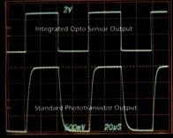
The SDP 8600 integrates a Schmitt trigger, voltage regulator, differential amplifier and photodiode onto the same substrate—replacing a complete PC board. This neat integration hasn't cost any performance. It has a propagation delay time of only 5 µs and a 50 ns rise and fall time.
