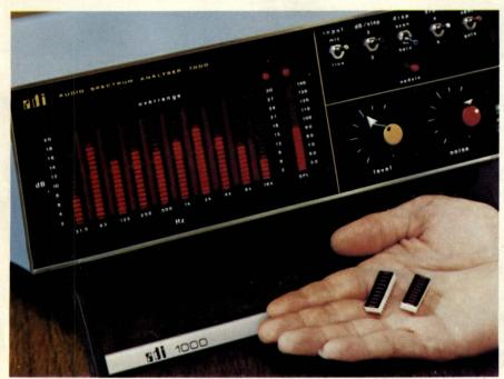
The relative intensities of spectral components in a 31.5-Hz to 16-kHz audio-frequency band correspond to the heights of the red-LED bar-graph columns in this spectrum analyzer from Audio Developments International. Each column consists of two 10-element Litronix RGB-1000 stackable modules.
