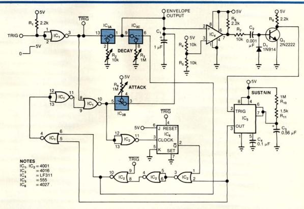
**CMOS switches** isolate the independently adjustable attack, sustain and decay times of this envelope generator. Determined by the 5V supply and the  $R_4/R_5$  ratio, the output swings between 0 and 2.5V—even for zero sustain times.
