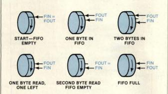
Fig 2—Two pointers indicate the next available memory location (FIN) and the last-used location (FOUT).
