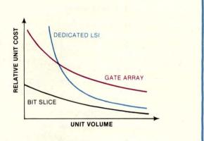
Fig 3—The relative unit cost of logic-design alternatives shows gate arrays with an advantage over dedicated LSI at lower volumes. (Source: Fairchild Semiconductor Div)
