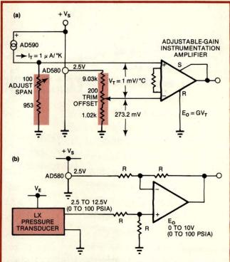
Fig 2—Range offsetting is a simple but effective method for converting measurements from degrees Kelvin to degrees Celsius (a) or translating the output of high-level transducers whose ranges are offset from zero (b).
