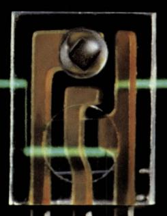
It's a logical breakthrough from Spectronics. We've designed the first opto detector IC offering compatability with TTL, CMOS and other standard logic families.
