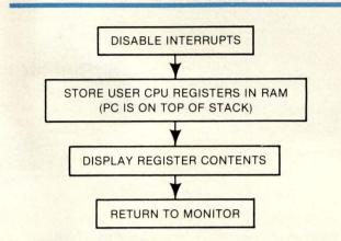
Fig 3—An interrupt-service routine stores the processor's status, displays it and returns to the system monitor.
