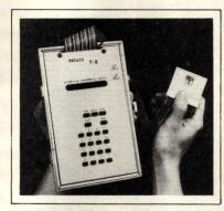
$\mu$ C ANALYZER. You can troubleshoot 6800- $\mu$ P-based systems by single stepping through development or diagnostic programs with the hand-held,  $\mu$ P-based Model T-8. The unit stores information from 63 machine cycles occurring before a user-selected break-
