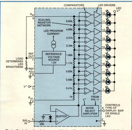
Fig 1—Basic functional elements of National Semiconductor's LM3914/15/16 dotor bar-display drivers allow the chips' outputs to drive 10 LEDs in a moving-dot mode (if pin 9 is open) or a rising-bar mode (if pin 9 is tied to V+). The ICs can also drive vacuum-fluorescent devices and LCDs.
