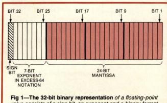
Fig 1—The 32-bit binary representation of a floating-point value consists of a sign bit, an exponent and a binary-format mantissa.
