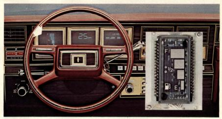
**Analog-sensor and bar-element-driver ICs** control vacuum-fluorescent (VF) display devices like the 32-bar VF fuel gauge shown in the inset and used in several 1980 Ford car models (arrow). When the tank is full, all 32 elements glow a bright green, but as fuel is used, the bars darken sequentially, from the top down.
