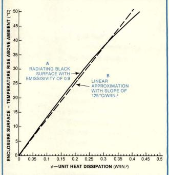
Fig 1—An enclosure's surface-temperature rise as a function of its unit power dissipation  $\phi_{\text{DISS}}$  (assuming 0.9 surface emissivity) becomes easy to compute when using curve B—a linear approximation of the actual thermodynamic curve A.
