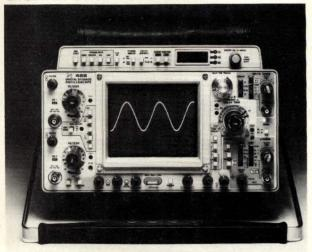
By combining a display-interpolation technique with a 25M-sample/sec, 8-bit digitizer, Model 468 achieves a 10-MHz useful storage bandwidth. Utilizing the interpolation concept, the unit requires 2.5 samples per cycle to achieve this capability.
