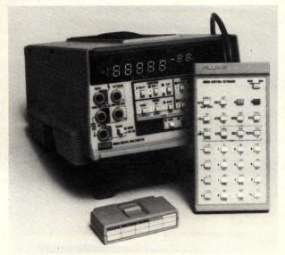
The 5½-digit Model 8860A features two  $\mu$ Ps, which control its front-panel-selectable functions and permit operation with two mutually exclusive options—IEEE-488 interface and calculator control.
