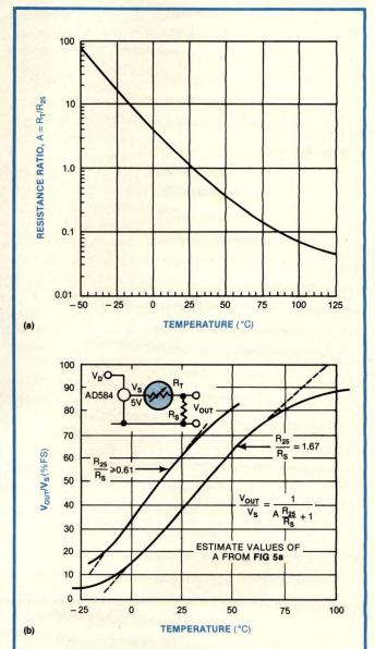
Fig 5—Although quite sensitive to temperature, thermistors are also highly nonlinear. Connecting resistors in series or parallel with a thermistor crudely linearizes device output (a) over a limited temperature range (b).
