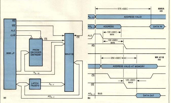
Fig 2—By substituting an MK4118 for the 2114 memory chips (a) and employing the μP's RD function as an output enable (OE), you hold the memory's output inactive (b); bus contention thus can't occur.
