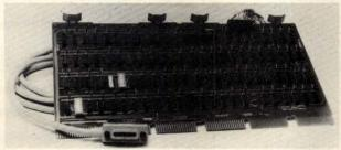
Plugging into any hex-wide SPC slot, the GPIB11-2 interface provides hardware for decoding GPIB talker, listener and controller functions and can be used in single- or multicontroller systems.
