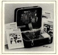
PORTABLE µP LAB. The Portable Training Lab (Course 525A) consists of 20 self-training modules (4 vols, 1650 pgs) and a complete 8080A-based hardware system. The texts cover programming fundamentals, real-timeinterrupt handling, control of programmable interfacing devices and closed-loop control-system implementation. Each module provides hands-on experiments that involve program coding and execution. \$1595. Integrated Computer Systems Inc, Box 5339, Santa Monica, CA 90405. Phone (213) 450-2060.
