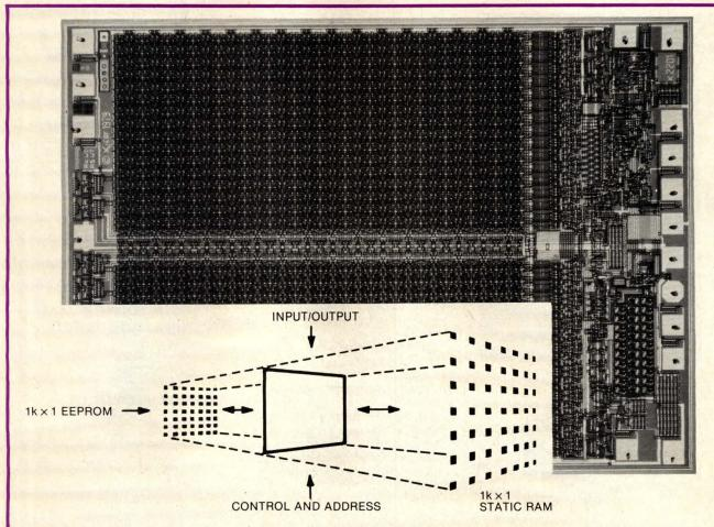
Fig 7—Requiring only one 5V supply, Xicor's X2201 nonvolatile RAM combines two independent bit-for-bit overlaid memories and employs n-channel floating-silicon-gate technology. Learn more about it at Electro/80 session 11.
