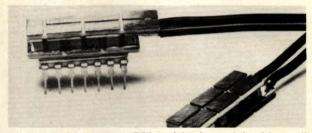
Sandwiched between a DIP and its heat sink, this small thermoelectric module can pump as much as 3.5W of heat out of the DIP.
