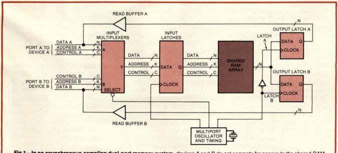
Fig 1—In an asynchronous-sampling dual-port memory system, devices A and B do not compete for access to the shared RAM array. Instead, under precise clock timing, input multiplexers and input and output latches alternately allocate memory access to ports A and B for data, address and control transactions.
