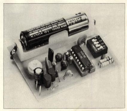
Two melodies, a door chime and a beeping alarm emerge from a 16-pin 7910 Series IC, shown here mounted in its evaluation board. The chip contains separate main-tune and accompanyment generators and several ROMs that allow it to play tunes of up to 128 notes over a wide range of tempos.
