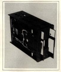
and interface compatibility with other single 5.25-in. disc drives, Model A-40 Dam provides single-side dual-density recording on 40 tracks of each diskette. Track-to-track access time of 12 msec produces a random average seek time of 170 msec. Unformatted storage capacity is 256k bytes per diskette or 512k bytes per drive. \$450. T and E Engineering, 1015 W 190th St, Gardena, CA 90248. Phone (213) 327-7657. Circle No 272
