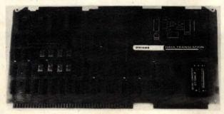
Although it's called an intelligent analog peripheral, Model DT3752 is really a  $\mu$ C-based, stand-alone, single-board analog data-acquisition system. The standard version provides 16 single-ended or eight differential-input multiplexed analog channels, a 12-bit ADC, 35-kHz throughput rate, 16k bytes of dual-port RAM, on-card DMA and serial as well as parallel I/O.
