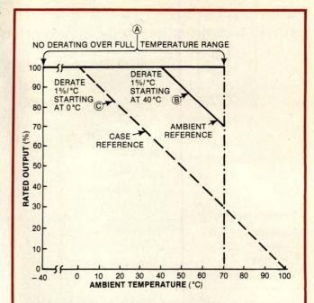
Fig 3—Power-supply temperature specs can be stated relative to ambient or case temperatures. If you assume the wrong reference, though, the supply will probably go up in smoke. A, B and C refer to supplies exhibiting three different temperature characteristics (see text).
