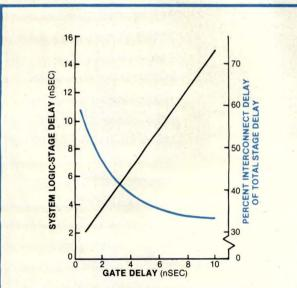
Fig 1—Shorter gate delays imply a need for fewer computer-system interconnects in order to achieve optimum performance. As Electro/80 session 22 will show, gate arrays provide one way of achieving this goal. (Source: Fairchild Semiconductor Div)
