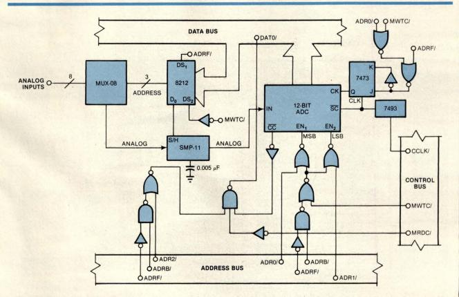
Speedy data acquisition results with this 8-channel, 12-bit system. Interfacing to an 8080 Microbus, it expands to 64 channels with the help of four MUX-16s.
