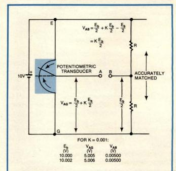
Fig 1—An offsetting bridge provides reduced sensitivity to variations in power-supply voltage. Note that even a 20% change in the fractional part of  $V_{AG}$  essentially produces no change in  $V_{AB}$ .
