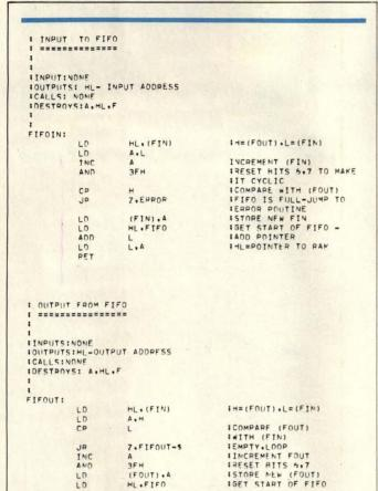
Fig 1—Using only two bytes of RAM, plus the RAM already assigned to the stack, these routines implement storage that acts like a cyclic memory space.
