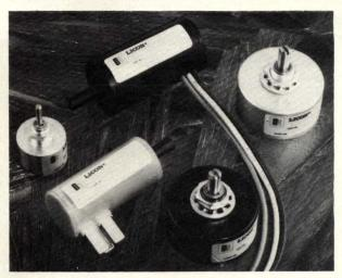
Available in linear and rotary versions, Series 33 position sensors employ two ferrite tubes wound as inductors and connected in series. Attached to each unit's input shaft, a permanent magnet linearly varies the core's differential inductance in direct relation to shaft position. When excited with an ac signal, the sensors output an ac voltage linear and proportional to position.
