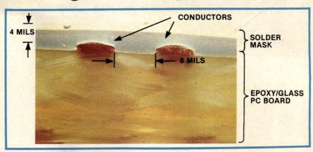
If improperly applied, dry-film solder masks leave voids between closely spaced conductors on the surface of a pc board. These voids can trap moisture and impurities, thereby creating leakage paths. This cross-sectional view illustrates the proper application of such a mask; the 4-mil-thick mask (blue-tinted layer) completely fills the 6-mil-wide space between conductors on the surface of an epoxy/glass board. Note also the glass-fiber weaving inside the board (Photo courtesy Dynachem Corp)
