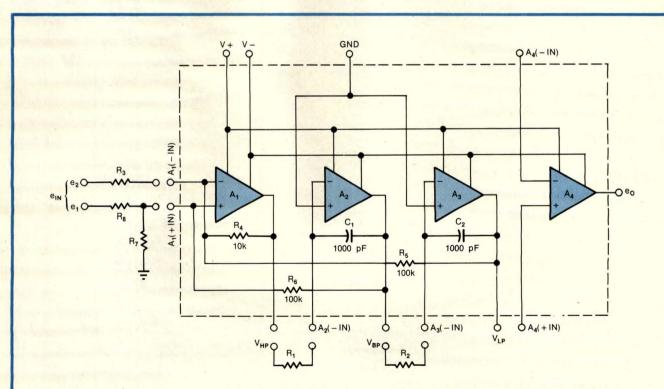
Fig 1—The universal active filter used in this article's design example, General Instrument's ACF7092C is similar to most other IJAFs.
