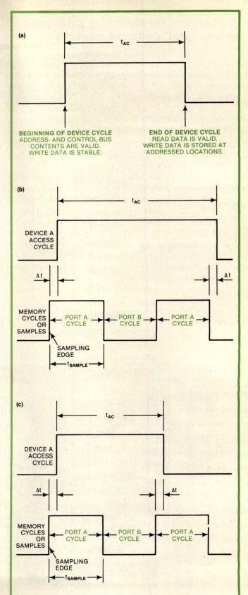
Fig 2—Clock timing for an asynchronous-sampling dual-port memory involves three steps: establishing memory access as a simple Start/End sequence, t<sub>AC</sub> (a), squeezing two port-A cycles into device A's Read cycle to guarantee a complete asynchronous memory cycle (b) and requiring only one sampling-clock leading edge for device A's Write cycle, because the input latches allow memory Write cycles to complete independently of the attached device (c).
