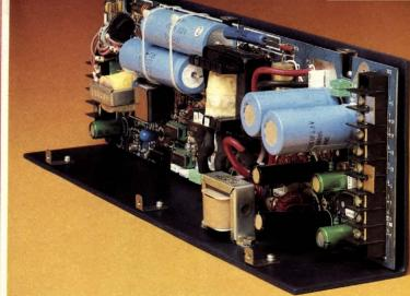
The SWS 250T Series switching regulated DC power supplies offer high efficiency with maximum reliability and performance plus multiple output versatility.
