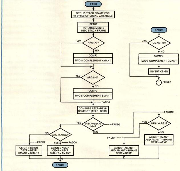
Fig 5—FADD performs floating-point addition of two 32-bit arguments.
