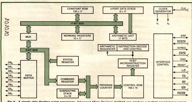
Fig 6—A single-chip floating-point processor, Advanced Micro Devices' Am9512 can produce a tenfold speed improvement compared with its 8080A-μP software counterpart. Electro/80 session 14 will examine current developments in such devices.
