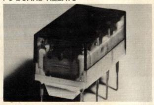
Sealed against wave soldering and cleaning-solvent damage, RD Series DIP-sized relays offer a wide selection of coil-voltage and contact configurations. Insulation resistance specs at  $100\text{-}M\Omega$  min, and dielectric strength between contact and coil or opposite-polarity contacts equals 1 kV ac.
