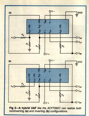
$$G_{(LP)} = \frac{G_{LP} \omega_n^2}{s^2 + \left(\frac{\omega_n}{Q}\right) s + \omega_n^2}$$
