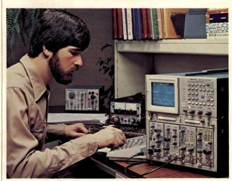
Digital storage, programmability and an IEEE-488 interface combine with 400-MHz analog performance in Tektronix's 7854.
