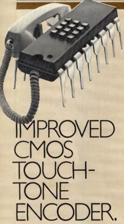
popular CMOS 7206 touch tone encoder. The new ICM7206C combines both oscillator mute and single contact keyboard functions on one chip—and avoids spurious side tones. The 2-of-8 sine wave touch tone encoder features fast oscillator startup (5ms), extemely low distortion (<5%) and low voltage operation (down to 3V). The ICM7206C works with either 3x4 or 4x4 key formats for minimum cost keyboard design. It's intended for telephones, numeric data entry and the like. Check 21.
