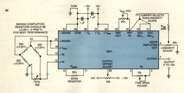
utilize the output of a bridge preamplifier to modulate a bridge's excitation. An external adjustment circuit applied to the 2B31 bridge/signal conditioner provides a degree of over- or undercorrection to partially compensate for the nonlinearity of the device (such as an RTD) as well as the bridge.
