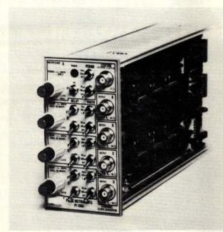
channels provide pulse widths variable from 10 nsec to 1 msec. Driving a terminated  $50\Omega$  line, the 2V-min output pulses exhibit rise and fall times of less than 7 nsec. \$790.
