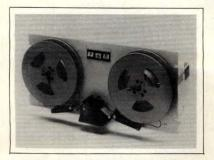
PAPER-TAPE READER. Model RR7155 has 200-cps asynchronous or synchronous read speed and 400-cps tape-positioning mode for rewinding on program cueing. Stepper-motor controlled, the 5.5-in.-high unit uses only one moving part, offers stop-on-character capability at all speeds and mounts on a 19-in. rack. An optional add-on fanfold tank assembly is available; MTBF specs at 16,000 to 20,000 hrs. \$657 (OEM qty). Remex, Box C-19533, Irvine, CA 92713. Phone (714) 557-6860. Circle No 271
