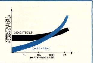
Fig 4—The cost of LSI procurement (including start-up) is lower for gate arrays than for dedicated LSI at lower volumes. (Source: Fairchild Semiconductor Div)
