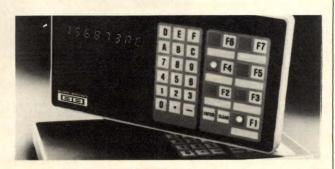
buffered input permits data or message verification before transmission to the processor at 110 or 300 baud. One DB-25 connector handles the power and I/O lines. \$249 for hexadecimal- or numeric-keyboard version.
