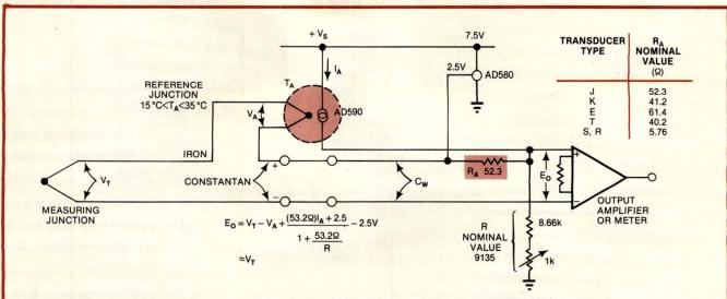
Fig 3—Cold-junction compensation provides a thermocouple reference in applications where using an ice bath for the reference junction is inconvenient. Through changes in the value of R<sub>Λ</sub>, the circuit accommodates a variety of thermocouple types.
