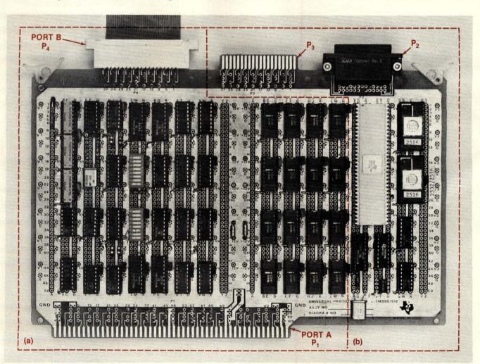
Fig 3—An asynchronous-sampling 8k-byte dual-port memory card (designed in this case for a Texas Instruments TM 990 computer system) serves varied applications: as a stand-alone asynchronous-sampling memory with ports at  $P_1$  and  $P_4$  (a) and as a multiprocessor system with an on-board peripheral processor interacting with an off-board backplane CPU (b).
