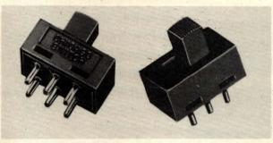
Featuring 2-piece bodies, Series 124 slide switches can be wave soldered without contaminating their contacts. Only the lower base inserts into the pc board and is wave soldered and cleaned; the units' top half is then hand-snapped on.
