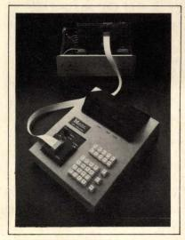
PROM EMULATOR. The ROSI ROMsimulation personality module allows program evaluation before ROM programming when used with the IM1010 PROM-programming system. The module features a 4k×8-bit RAM, which permits emulation of one to four PROMs and allows correspondence between PROM and RAM addresses. The module features standard RAM access time of 300 nsec; faster times are also available. \$595. International Microsystems Inc. 11554 C Ave, Auburn, CA 95603. Phone (916) 885-7262. Circle No 348
