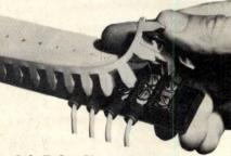
Safe-Ti Caps™ protect connections against spills, dirt and accidental short circuits from dropped tools.
