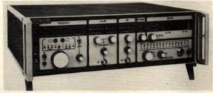
Spanning 300 kHz to 650 MHz, the Model 460 synthesized signal generator combines a -140-dBc/Hz noise-floor figure with stability and accuracy specs of  $\pm 1 \times 10^{-8}/24$  hrs.
