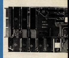
SINGLE BOARD COMPUTER \$99.50 with 6800 MI 6850 serial I/O, 2 6820 parallel I/O (32 line 512 RAM, socket for 2708, 2716, EROM. Interfamodules for industrial control, data acquisiti lab instrumentation, on 44 pin 4½" × 6½" PCE RAM, ROM, CMOS RAM/battery, A/D, D Driver/Sensor, Serial I/O, Parallel I/O, Count Timer, IEEE 488 GPIB, floppy controller. \*O (500 piece) price WINTEK Corp.—Phone (317) 7 8428 1801 South Street, Lafayette, IN 47904
