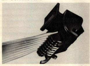
Employing an insulation-displacement contact scheme, Midas Series zero-insertion-force connectors provide a disconnectable interface with pc-board interior surfaces—without the need for an on-board mating unit. Their 4-slot design provides eight separate contact points with each lead, eliminating the need for wire stripping and soldering.
