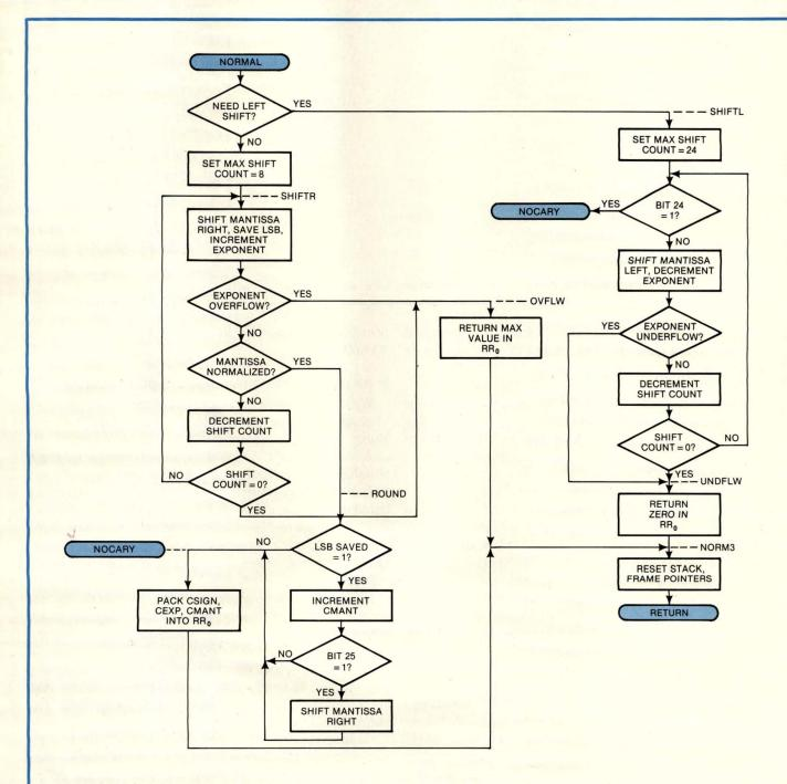
Fig 4—The NORMAL subroutine finishes the floating-point processing by normalizing the result and packing it into RR<sub>0</sub>.
