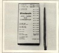
14-BIT ADC. Providing four selectable input ranges of  $\pm 10$ ,  $\pm 5$ , 0 to +5 and 0 to +10V, ADC-14-QM offers conversion time of 50 μsec and differential linearity of  $\pm \frac{1}{2}$  LSB max over the temperature range of 0 to  $70^{\circ}$ C. The stable unit furnishes differential nonlinearity and offset TCs of  $<\pm 5$  ppm/°C and measures  $2\times 4\times 0.4$  in. Power dissipation specs at 2.5W. \$186 (25). Intech, 282 Brokaw Rd, Santa Clara, CA 95050. Phone (408) 244-0500.
