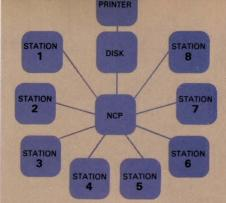
2300 Series multi-station networks share disk and printer with up to eight stations. Each station is universal and may be ordered with the software and/or hardware capabilities required.
