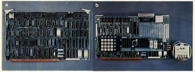
A low-cost means of providing  $\mu$ P-technology updates, Motorola's MEK6809D4 evaluation module (a) can function in a stand-alone mode or in concert with the MEK68KPD display/keyboard/wire-wrapping board (b).
