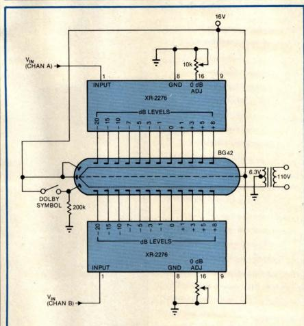
Fig 5—Twin-channel audio-level indication results from using two Exar 2276 12-element VF bar-graph drivers. The output of each 2276 illuminates half of a dual 12-bar display (Futaba BG42 or NEC 2B1745). The 12 elements span a range of -8 to +20 dB; the 10-kΩ pots adjust the 0-dB reference levels for both channels.
