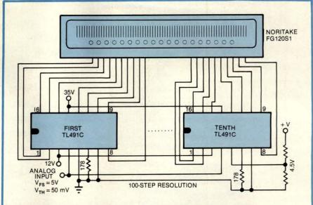
**Fig 3—100-step resolution** of an analog input quantity results when you drive a Noritake 100-bar vacuum-fluorescent display with cascaded Texas Instruments 10-step analog detector/drivers. For a 5V full-scale input, each lighted bar represents a 50-mV increment.
