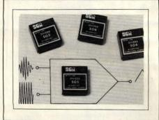
**2-QUADRANT DIVIDERS.** For interfacing with  $\mu P$ -based systems, Models 503 through 506 0.5-in.³ microhybrid modules include a transconductance dividing element, a stable reference and an output amplifier with specified accuracy, internally trimmed for feedthrough, output zero and gain. Transfer function is 10X/Y, and dividing accuracy (at 25°C) ranges from 1.0 to 0.1%, including the effects of offset voltage, feedthrough,
