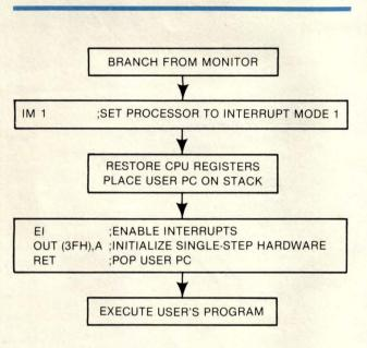
Fig 2—A single-step subroutine sets the processor to Interrupt mode, enables interrupts, initializes the associated hardware and returns the processor to the user program.
