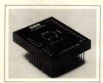
D/S CONVERTER. A 14-bit 400-Hz unit, DSC-644 is a pin-for-pin replacement for the industry-standard 400-Hz EDSC-H and -L. The 3.125×2.625×0.52-in., 5.5-oz module meets or exceeds MIL-STD-202E and features a typical output-scale-factor variation of 0.05% and a current-limiting output stage that is short-circuit proof. Accurate to ±4", the
