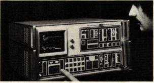
Featuring a full 70-dB dynamic range and touch-control front-panel operation, Model SD345 FFT signal analyzer provides 400-line spectral analysis to 100 kHz. Options include IEEE-488/RS-232 I/O interfaces, ½- and full-octave acoustic data analysis and digital spectrum expansion to 100×.
