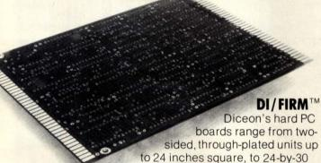
inch multilayer laminates with as many as 12 circuit layers, including back panels.
