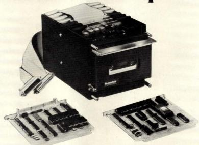
The M80 is a general purpose Z80™ based computer combined with a rugged, high-speed digital cassette drive in a compact, panel mounting module. Modem and terminal RS232C and TTY current-loop serial ports are provided for easy interfacing. A 2K PROM is programmed to implement completely interrupt driven control of the recorder and communications functions. A 1K RAM provides data buffering which allows the M80 to handle continuous streams of data up to 9600 BAUD.
