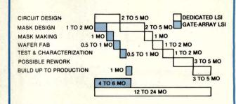
Fig 2—Gate arrays provide significant development-time advantages compared with conventional LSI. (Source: Fairchild Semiconductor Div)
