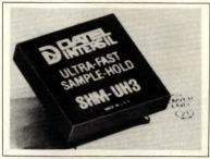
SAMPLE/HOLD. For use with ultrafast A/D converters with up to 10-bit resolution, SHM-UH3 features 30-nsec acquisition time and 30-psec aperture uncertainty time. It samples a 20-MHz, 10V p-p sinusoid to 8-bit accuracy (½-LSB uncertainty); it can also sample at up to 10 MHz while making full-scale acquisitions. Sample-mode bandwidth is 45 MHz, and output slew rate equals 500V/µsec.
