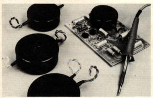
Employing toroidal cores, devices in this family of 50/60-Hz power transformers manufactured by Avel-Lindberg Ltd are about 50% smaller and lighter than equivalently rated units. Because there's no air gap, reluctance losses are low—important in "instant-on" applications—and electrically induced hum or noise is eight times lower than that exhibited by stacked, laminated transformers.
