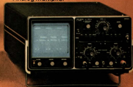
PM3233 10MHz Dual Beam Scope
