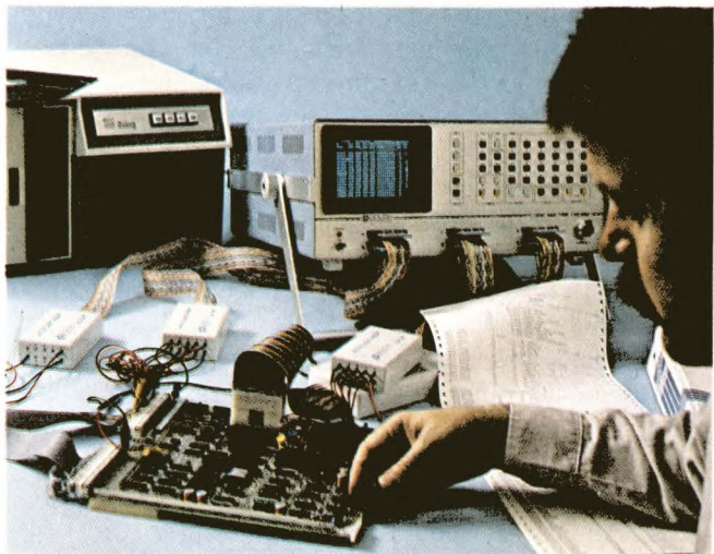
If your bus stops, trace the trouble with a logic analyzer like Gould/Biomation's K-100D. The analyzer itself is controllable via the bus for use in test systems.
