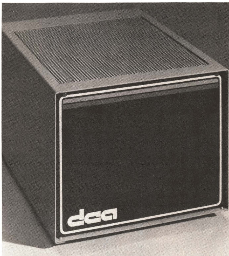
Modem-sharing features in Digital Communications Associates' System 105 allow two or more units to use a single trunk-line modem, thereby reducing system costs.
