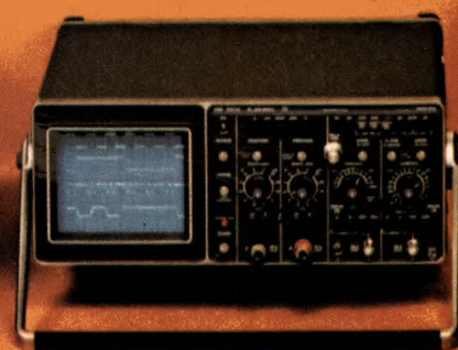
PM3214 25MHz Delayed Time Base Scope
