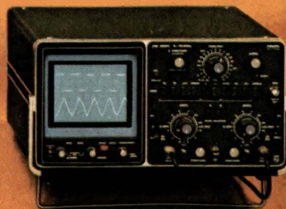
PM3234 10MHz Dual Beam Storage Scope
