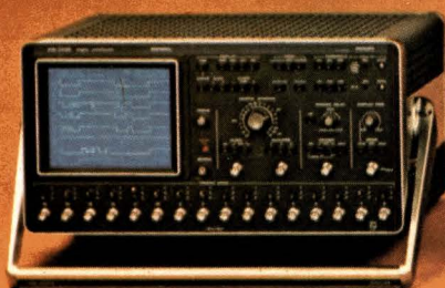
PM3500 100MHz 16 Channel Logic Analyzer
