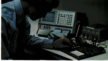
Adapter boxes ease the switch from 8- to 16-bit systems. While Biomation's K100-D has only 16 lines, a 32-channel adapter for it is available.
