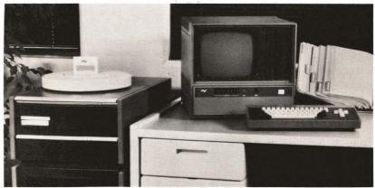
Providing increased performance and program capacity compared with its predecessors, the Intellec Series II Model 240 development system comes with a cartridge disc that decreases system response time.
