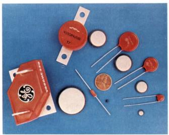
Transients from 8 to 1800V can be suppressed with metal-oxide variable resistors (MOVs) like General Electric's, shown here before and after encapsulation. The white areas on the MOV discs are the contacts. Larger sizes pass more breakdown current when maintaining the voltage across them and the protected circuit at safe levels.
