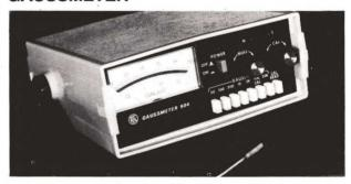
Model 904 measures magnetic flux in the range between 30G and 30 kG, achieving 3% FS accuracy. LED lamps adjacent to its analog meter indicate field polarity, and an analog output voltage corresponding to the flux density of either dc or ac fields is available at the rear panel.
