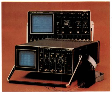
**Trigger probes** extend the usefulness of 16-channel analyzers like Philips' PM 3500. This instrument handles up to 56 trigger channels in 8-bit increments.
