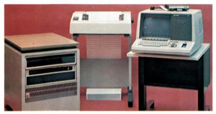
Multiuser capability makes the HP64000's use of high-performance peripherals (such as its 20M-byte disc) economically feasible, thus easing the development task.
