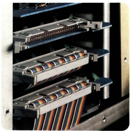
Scotchflex headers (.100" x .100" grid series) now include built-in retainer/ejector latches that snap up to lock sockets firmly in place and snap down to disconnect them quickly and easily. Latches hold tightly against vibration and shock,
