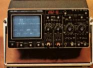
PM3263 100MHz Microprocessor-Equipped Scope with Digital Delay
