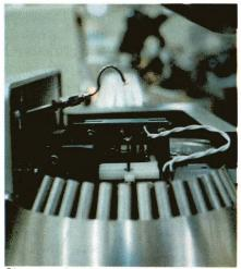
Siemens- developed proprietary die tester. Tests and sorts according to specifications.
