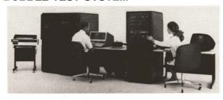
The Model 5585 magnetic-bubble-memory test system handles up to 65M-bit devices and accommodates serial, major/minor-loop, block-replicate and odd/even memory architectures.
