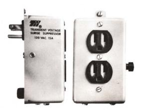
Designed to provide positive protection from lightning, switching transients and overvoltage, plug-in Models 427 and 428 operate automatically and are self-restoring. Each self-contained device plugs into a  $117V\pm10\%/15A$  single-phase wall socket that accepts NEMA 5-15-type 3-prong connectors.
