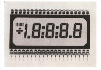
Measuring  $2\times1.2$  in. overall, the 4½-digit Model FE0206 comes in transmissive, reflective or transflective modes and with -10 to  $+55^{\circ}$ C or -5 to  $+80^{\circ}$ C materials; you can specify either DIP-pin or pinless connections.
