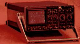
PM3265 150MHz Scope with 100MHz Analog Multiplier
