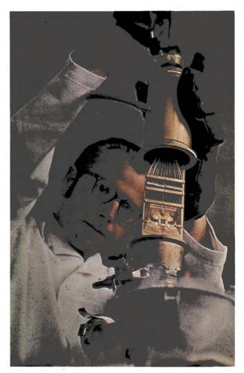
**Lowered into a liquid-helium bath,** a Josephson memory device's metal junctions become superconducting. Each memory cell in this 2k-bit IBM chip stores a single quantum of magnetic flux—an energy level of less than 10<sup>-18</sup>J.
