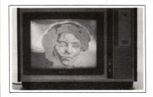
VIDEO DIGITIZER. Under program control, the FG-01 quantizes a video source to form a 256×256-element image of either 4, 6 or 8 bits per pixel. This board then loads the image data into the manufacturer's RGB-256 videorefresh board. Once digitized, the live image can be frozen on command, allowing full computer access. Less than \$800. Matrox Electronic Systems Ltd, 5800 Andover Ave, Montreal, QUE H4T 1H4, Canada. Phone (514) 735-1182.
