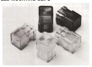
Because of their construction, which features molded Fresnel rings and striated lines on the viewing surface, Series 1933 square-lens clips for T-1¼ LED lamps provide even illumination. Their cellulose-acetate-butyrate bodies are available in amber, clear, green, red or yellow.
