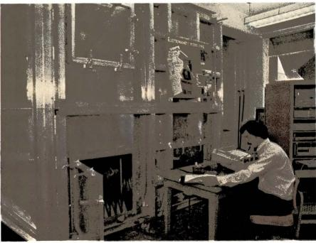
The susceptibility of electronic equipment to electromagnetic interference can be measured with a transverse electromagnetic (TEM) cell like this 3m-cross-section unit. The cell's input connector is at the tip of the pyramid-shaped section on the left.
