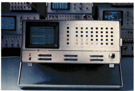
Even 16-bit processors don't have too many lines for Dolch/Kontron's LAM4850 logic analyzer to handle. It accommodates 48 inputs at clock rates of up to 50 MHz.
