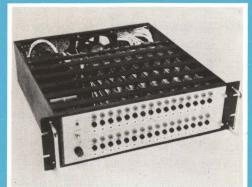
NEW LOW LEVEL INSTRUMENTATION AMPLIFIER SUBSYSTEMS specially designed high performance units can interface directly with PDI's 6000 & 7000 subsystems. Performance characteristics: high gains to 500; accuracy: 0.01%; linearity: 0.005%; very low gain; offset temp. coeff. & 2 pole Butterworth filter option. Std. 19" rack mount chassis with max. of 32 chan-Phoenix Data, Inc., 3384 W. Osborn, Phoenix, AZ 85017. PH 602/278-8528 TWX 910-951-1364
