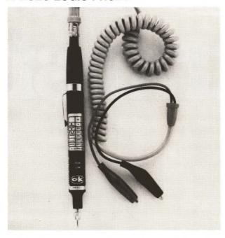
Although it's inexpensive, Model PRB-1 detects pulses with durations as short as 10 nsec and provides frequency response to 50 MHz. Pulse stretching to 50 nsec (plus and minus) is automatic.
