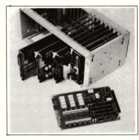
I/O TERMINAL. The SE100 measures, digitizes, isolates and transmits industrial-process data to computers, terminals and modems, as well as completing control loops to isolated DACs and switch closures. Featuring remote self calibration, automatic cable-break protection and complete optical isolation, it handles a variety of sensor and data interfaces. From \$1490. San Diego Instrument Laboratory, 7969 Engineer Rd, San Diego, CA 92111. Phone (714) 292-0646.
