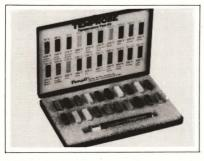
**TEMPERATURE TEST KIT.** Although only pocket sized, the Temprobe kit contains 20 temperature-indicating crayons that cover 125 to  $800^{\circ}F$  (52 to  $427^{\circ}C$ ). Each crayon melts at a specific temperature, guaranteed within  $\pm 1\%$ . A special metal holder/marker makes application easy. \$10. **Tempil**, Hamilton Blvd, South Plainfield, NJ 07080. Phone (201) 757-8300. **Circle No 300**
