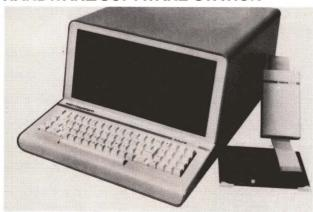
The AMDS-AST provides you with all necessary tools for  $8080,\,8085,\,6800,\,6802$  or Z80  $\mu P$ -based product design and testing. A CPU, universal logic analyzer, CRT and keyboard are all integrated into this compact station, which has a built-in high-speed network interface for sharing disc and printer sources.
