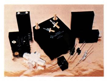
Voltage spikes and surges that can destroy semiconductors and microprocessors are clamped to safe levels by special avalanche breakdown diodes such as these TransZorbs from General Semiconductor Industries.
