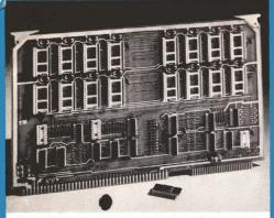
SBC 80 Compatible 32K PROM board. The PROM-32 accepts sixteen 2716 E-PROMs. All IC's are socketed. The base addresses of the memory fall on 16K boundaries and are settable to 0000, 4000, 8000, and C000 Hex. Any 2K memory block may be deserlected. This feature allows other boards to use the deselected address blocks. Best of all is our 3 yr warranty! \$250 (Qty. 1-9). Stock. Electronic Solutions, Inc., 7969 Engineer Rd., San Diego, CA 92111. (714) 292-0242.
