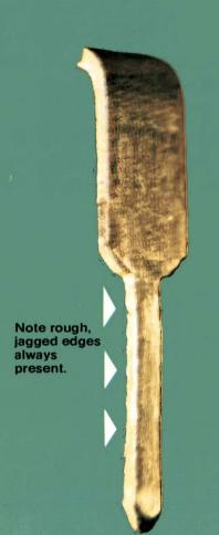
Your IC lead frames look like this at 30X enlargement (unretouched). Because they are punched out of metal, the edges are rough, jagged and irregular. In contrast, the flat sides of the lead frame are smooth, even and perfectly plated.
