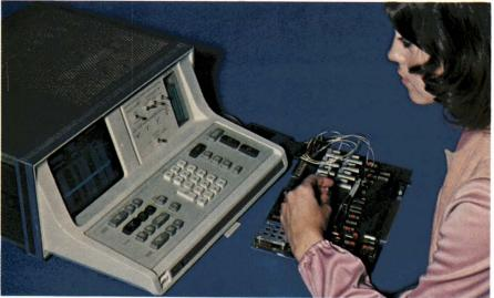
Logic analyzers are flexible enough to change input-channel assignments. On Hewlett-Packard's 1611A, you can swap address, data and other lines to configure 36 input channels—more than enough to accommodate 16-bit-µP systems.
