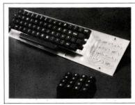
KEYBOARDS. Because of their crossbar contact design, Sabrecoil keyboards incorporate only three parts for each switch position. The 1-piece frame that houses all switch parts provides ease of mounting and deflection resistance for the entire assembly.
