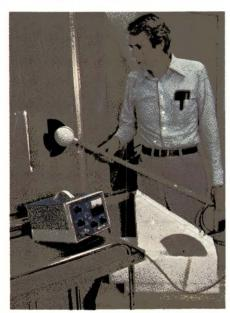
An isotropic antenna developed at the National Bureau of Standards, Boulder, CO, is small and sensitive enough to measure the electromagnetic fields generated near signal sources. Its metering circuitry is housed in the blue box.
