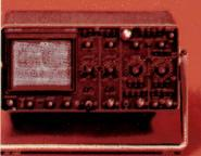
PM3262 100MHz Dual Trace Universal Scope with 3 Channel Display and Alternate Time Base
