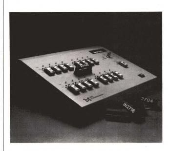
The IM2020 programmer aims at fault-proof operation by nontechnical personnel. It provides single-key operation of all modes, automatically checking PROMs and performing self diagnosis before operations commence.
