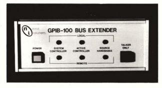
The GPIB-100 has RS-422-compatible line drivers and receivers that allow you to connect instruments separated by up to 300m, instead of the 4m allowed by the IEEE-488 bus. It also expands the maximum number of system components from 15 to 28 units.
