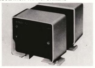
Various models of Stabiline IT isolation transformers protect  $\mu Ps,$  medical equipment, computers, industrial controls, communications equipment, processors and other sensitive loads from electrical noise on power lines. Ranging in power rating from 0.5 to 5 kVA, they offer  $1000\text{-}M\Omega$  insulation resistance, 2500V-rms dielectric (primary to secondary), 0.005-pF maximum interwinding capacitance and 126 dB of common-mode attenuation.
