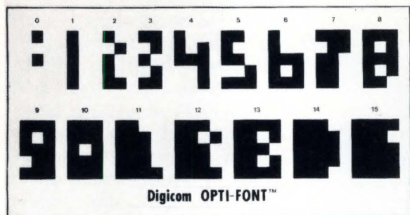
Fig. 1—Basic to the Direct Digital Graphics technique is the Opti-Font (left), a proprietary group of 16 optically weighted characters. Generated by the Digicoder, the characters literally create "pictures by the numbers", thus presenting digital data in graphic form. Characters are composed of dots on a 4 \times 5 matrix. Shown to the right is the Model D2
