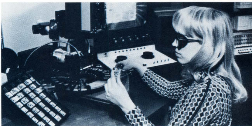
Better stabilities can be achieved with laser-trimmed thin-film resistors thanks to a Western Electric study. Here, a thin-film circuit is readied for active trimming via a Nd:YAG laser.
