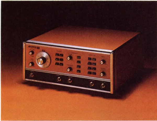
This function generator has a lot to offer. It can provide sine, square, triangle, pulse, ramp and sync waveforms over a frequency range of 0.005 Hz to 5 MHz. It also includes trigger, gate, variable dc, variable offset and VCF features for $395. (Ailtech)
