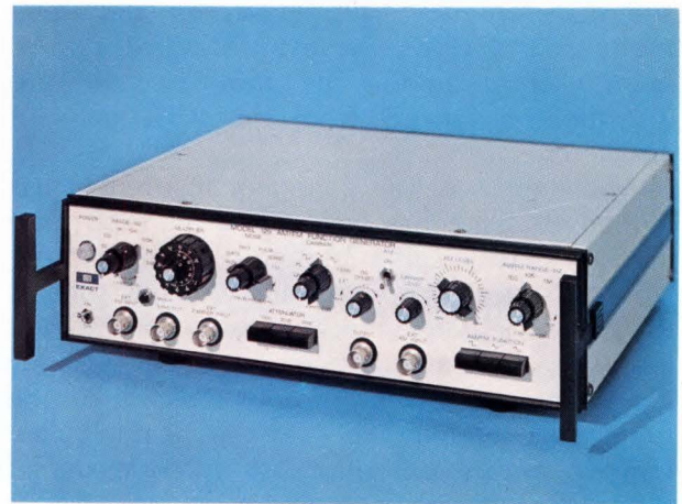
Model 129 is really two generators in one. The main generator offers VCF and has sine, square, triangle, \pm square, \pm pulse, \pm sine and sync waveforms over 0.1 Hz to 5 MHz. The AM/FM generator produces sine, square and triangle waveforms over 1 Hz to 1 MHz, has simultaneous AM and FM and can also be used to gate and trigger the main generator for toneburst and pulse operation. Total cost is $895. (Exact)
