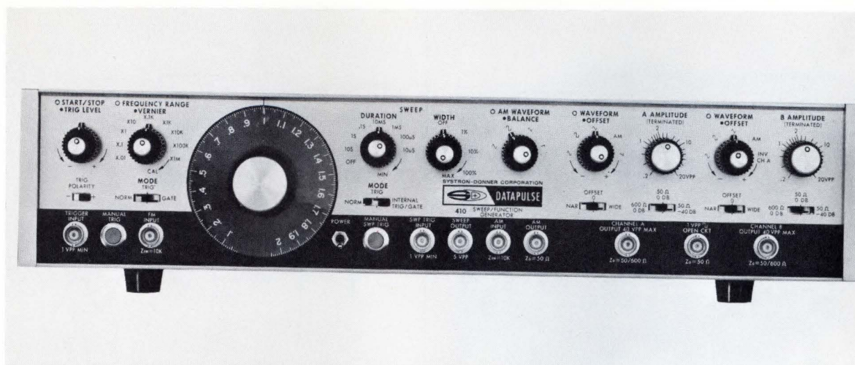
Model 410 is loaded with features. These include a 1000:1 sweep ratio, external triggering of both the main and sweep generators, FM and AM with 4-quadrant multiplication and a pair of 40V p-p (into an open circuit) output amplifiers with independent dc offset and waveform selection. The $995 generator features sine, square, triangle, pulse, sine squared and sawtooth waveforms over 0.0002 Hz to 2 MHz. ( Systron-Donner )
