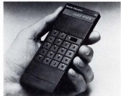
Duty-cycling the power supplied to the LSI/MOS chip allows this calculator to be very light (2-1/2 oz) and slim (3/8-in. thick).
