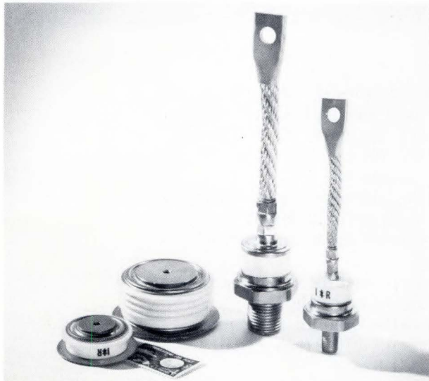
Fig. 1—Typical fast-recovery rectifier diodes have ratings of 100 and 250A for stud mounted types and 400 and 650A for hockey-pucks. Recovery times are typically less than two \mu sec.
