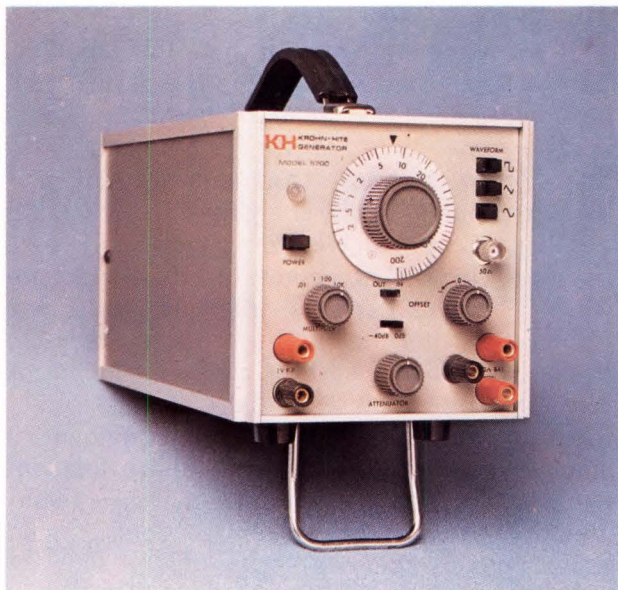
Low-cost function generators like this one offer a high performance/price ratio. The Model 5700 costs only $295 but offers sine, square and triangle waveforms over 0.002 Hz to 2 MHz, a 1000:1 tuning-dial ratio, auxiliary square waves, an output attenuator, dc offset control and two outputs—a 600 \Omega balanced output with 30V p-p into an open circuit and a 50 \Omega single ended output with 15V p-p into an open circuit. (Krohn-Hite)
