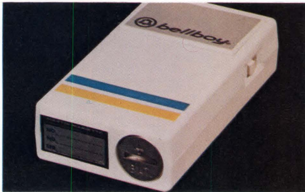
Micro sized paging system , made possible by reduced battery requirements of CMOS, is a joint project of RCA and Martin Marietta. It is already in use under the "Bellboy" trade name by five Bell System companies.
