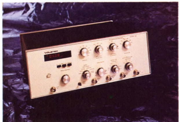
A digital readout for both frequency and amplitude is featured in Model 147. Covering a frequency range of 0.0005 Hz to 10 MHz, the 3-1/2-digit display instrument costing $1295 produces sine, square, triangle, positive and negative pulse, sawtooth, ramp and sync outputs. (Wavetek)
