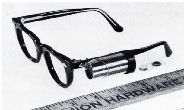
Blind seeing aid uses a miniature camera and tactile stimulation to aid the blind to locate, recognize and retrieve objects; read graphs, meters and oscilloscopes and also to distinguish colors. The camera was developed by the Smith-Kettlewell Institute for Visual Sciences and the 32 x 32-element self-scanning photodiode matrix was developed by Reticon Corp.
