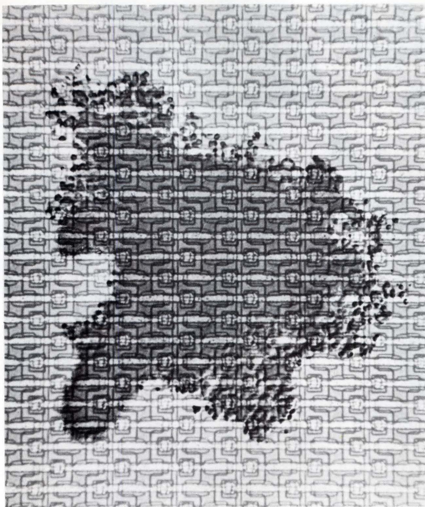
Fig. 3—8k-bit memory chip size reference, shows an amoeba (dark area), a one cell organism which is as large as 40 of the one-transistor memory cells in IBM's new device.
