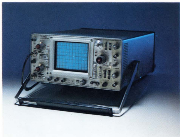
Fig. 6—The largest bandwidth and most sensitive oscilloscopes to operate from rechargeable batteries are the Models 465 and 475 from Tektronix, Inc. Model 465 is rated for 100 MHz at 5 mV/div. and the 475 shown here, operates up to 200 MHz with a sensitivity of 2 mV/div. They are slated to replace the popular 453A/454A oscilloscopes.
