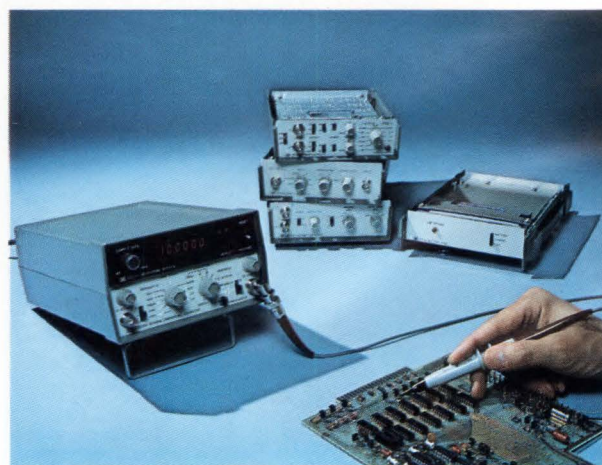
Fig. 8—The plug-on approach is used in Hewlett-Packard's 5300A electronic counter which allows the addition of either 10, 50 or 100-MHz modules as the need arises for maximum versatility and non-obsolescence. The system weighs only 3-1/3 lbs and operates from rechargeable Ni-Cd batteries (middle module).
