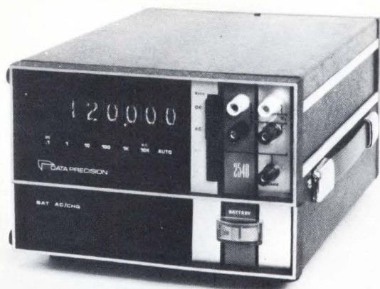
Fig. 5—The only 5-1/2-digit multimeter that operates from a battery (rechargeable lead oxide) is Data Precision's Model 2540 which dissipates only 12W of power. The meter incorporates three new major circuit advances—Triphasic conversion, Ratiohmic resistance and Isopolar reference—to cut the instrument's cost and enhance its performance.
