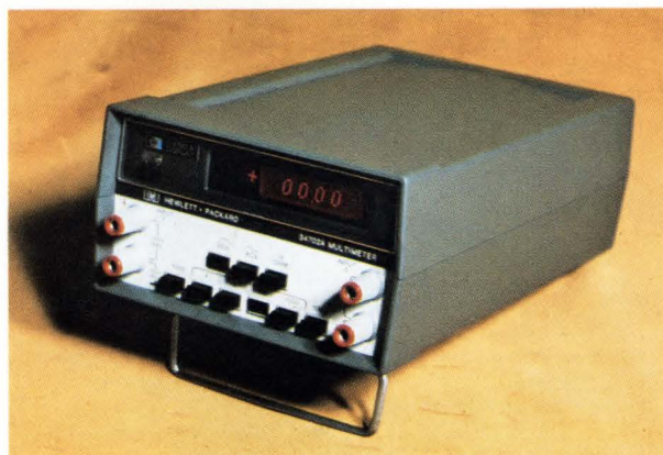
Fig. 10—Thanks to plug-on modules , Hewlett-Packard's Model 3470 digital measuring system can be configured as either a 4-digit multimeter or a 4-digit voltmeter, with the appropriate selection of the bottom module. A plug-on rechargeable Ni-Cd module can also be added to the system to allow for battery operation.
