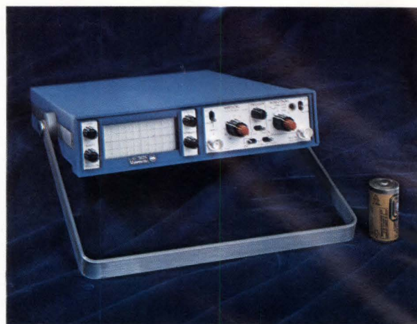
Fig. 7—A 20-MHz oscilloscope that fits into a briefcase is Vu-Data Corp.'s PS-900 unit. It offers 10-mV/div. sensitivity and weighs only 7 lbs (including batteries). A choice of Ni-Cd, alkaline or carbon zinc "C" cells are available for power. An internal recharge circuit is provided to cut-off batteries when fully recharged, so they can be placed in a recharge mode indefinitely without any damage.
