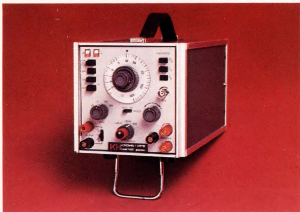
Fig. 11 — The latest portable function generator, the Krohn-Hite Model 5600, provides sine, square and triangle waveforms from 0.002 Hz to 2 MHz. It will operate on battery power for approximately 5 hours.
