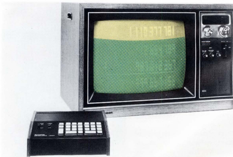
Contents of this novel calculator can be read on the screen of any ordinary television set.
