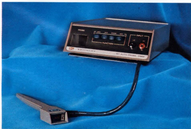
Fig. 2—Incorporating a LED-display probe with a push-to-read switch, Keithley's Model 167 Auto-Probe digital multimeter reaches new heights in portability. Operating on a set of six alkaline batteries, this fast-warmup unit has a dc-to-dc converter that shuts off whenever the batteries drop below a predetermined voltage level to guard against erroneous measurements.
