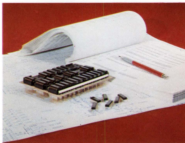
Fig. 2—Industry standards are the basis of the rapid growth of CAM. Starting with the almost universal acceptance of the DIP IC package, there is now a wide range of DIP support hardware that goes all the way up to the backplane level. This hardware standardization has in turn encouraged the development of expensive but labor-saving N/C machines for automatic handling of these standard parts. And these machines are what encourage the historic graphic language of engineering design to be translated into numeric form and handled by the computers.
