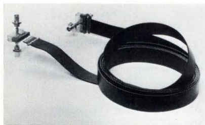
Fig. 1—Lowest flat flexible cable in crosstalk yet. Designated "Black Magic," it offers better than 5% crosstalk (both far-end and near-end), making it ideal for high-speed-computer interconnections. Note the ease of termination into a multi-conductor PC board with 0.05-in. spacings between conductors. The connectors shown are mounted in adapters for test purposes.
