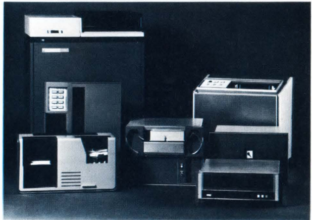
Fig. 5 Line printers, fixed and moving-head discs, tape transports and paper tape and card equipment are typical of standard peripheral equipment used with minicomputers.
