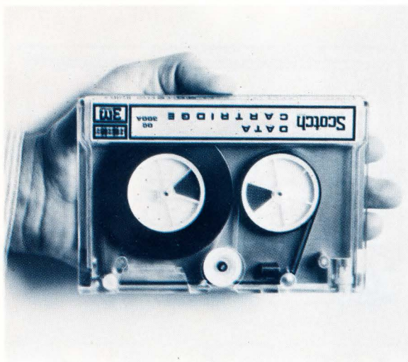
Fig. 3—The 3M cartridge that can really move tape at high speeds. 3M says their unusual drive-band arrangement will permit reliable read/write operation at 90 ips and searching at 180 ips! Note that it is practically a complete mechanical deck
