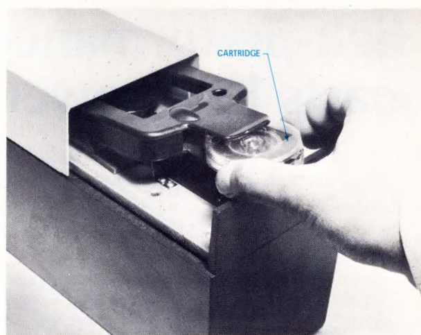
Fig. 5—Cogar's little heart-shaped cartridge contains just one of the tape reels. A tricky threading system automatically pulls the tape to the take-up reel that is permanently on the transport. (See photo at left)
