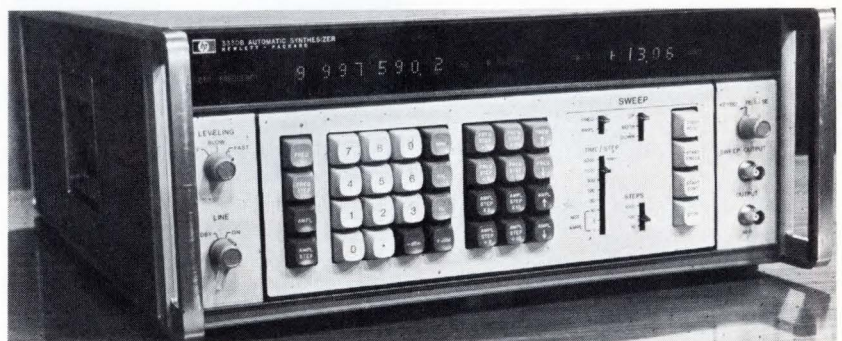
Using built-in ROMs, Hewlett-Packard's Model 3330B synthesizer allows complete amplitude and frequency programming from an upward-tiltable keyboard on the front panel. The instrument ranges over 0.1 Hz to 13 MHz at a constant resolution of 0.1 Hz.
