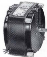
Type K Motors: Permanent-split capacitor instrument motors. Normal slip, high slip and synchronous windings. Stock ratings to 2.4 Oz-in. Only 2.405" square.
