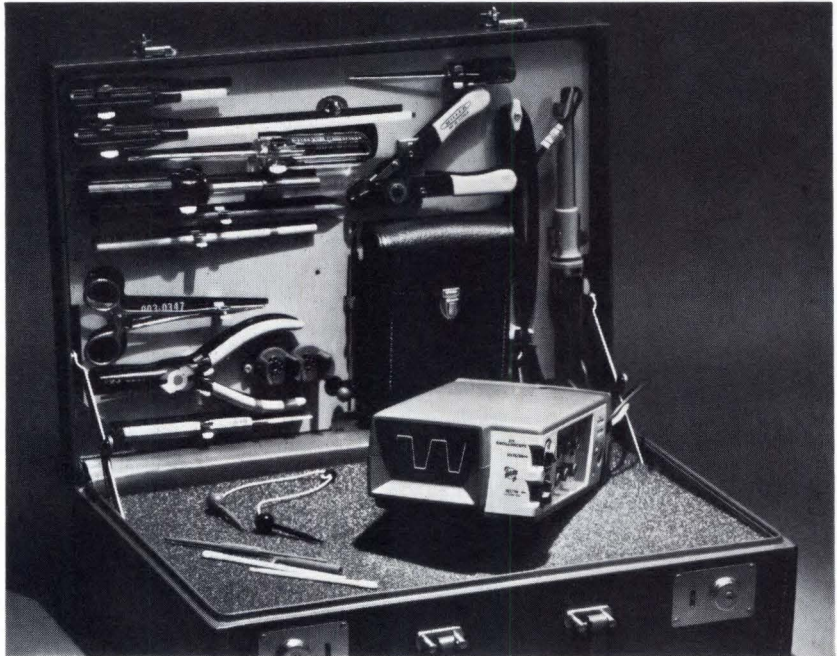
Tektronix Model 211 has taken the lead in reducing size and weight. This $545 unit weighs 3 lbs and has a 5-MHz bandwidth.
