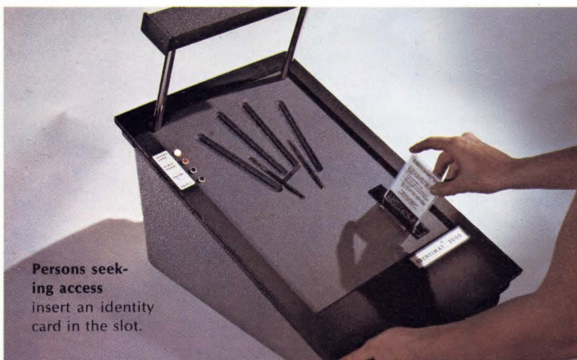
Placing their hand on the machine initiates an optical scan which is used for comparison with information coded on the card. Acceptance or rejection is indicated by panel lights.
