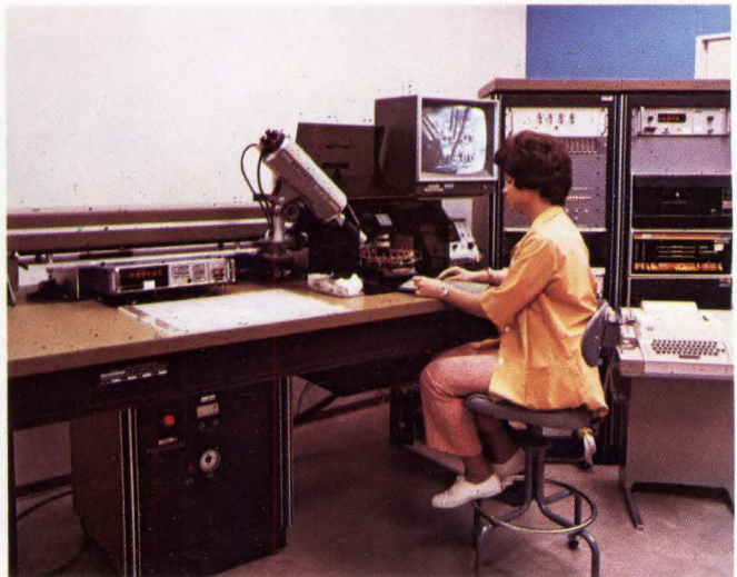
Entire laser/computer resistor trimming system. Laser safety shield normally is in down position, to protect operator from laser light. In photo, protective cover is raised, with laser off. "Teletype", to right, inputs operator instructions to system. Manual control box can be used to operate laser, stage motors, etc., and also contains emergency shutdown button. Left rack cabinet contains controls, interconnection matrices, power supplies and a programmable bridge.
