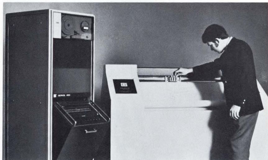
Drum plotter, Model 462 —claimed to be the fastest, largest and most accurate of its type available—consists of the Series 400 control (L) and Model 62 drum plotter (R).
