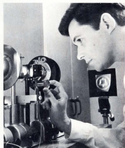
Bell Labs.' scientist adjusts focus on image of Bell System symbol projected from feric (ferroelectric picture device) onto small screen.
