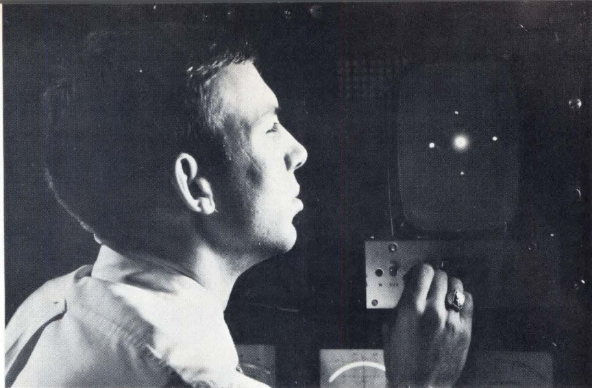
X-ray diffraction pattern of a pentaerythritol crystal is produced "live" on TV monitor by a camera tube that is similar to the one used for "Picturephone" service.
