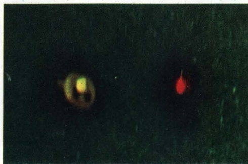
Fig. 1 — LED light output. The red Monsanto GaAsP (right) is operating at about 1.5V and 10mA. The yellow General Electric SiC (left) is operating at about 5V and 100 mA. The GaAsP is running cool but the SiC is running hot. The GaAsP is a passivated die covered by a dropped-on epoxy lens that magnifies its chip spot size. The SiC is just a bare, unpassivated chip on a header.
