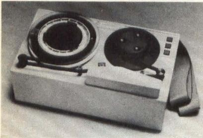
Holding up to 900' of magnetic tape, this 9-track reel-to-reel storage system (Reel-Core 7) stores up to 33 Mbytes of information on its 7" reel. Recording at 1600 and 3200 bpi, the Reel-Core 7 has tape speeds of 25 and 50 inches/sec, and can copy data at a maximum rate of 80,000 cps. It also has built-in diagnostics for self-testing and comes with its own PC-compatible board and software. Price is \$4,495. **Lancore Technologies** Westlake, CA **Circle 174**
