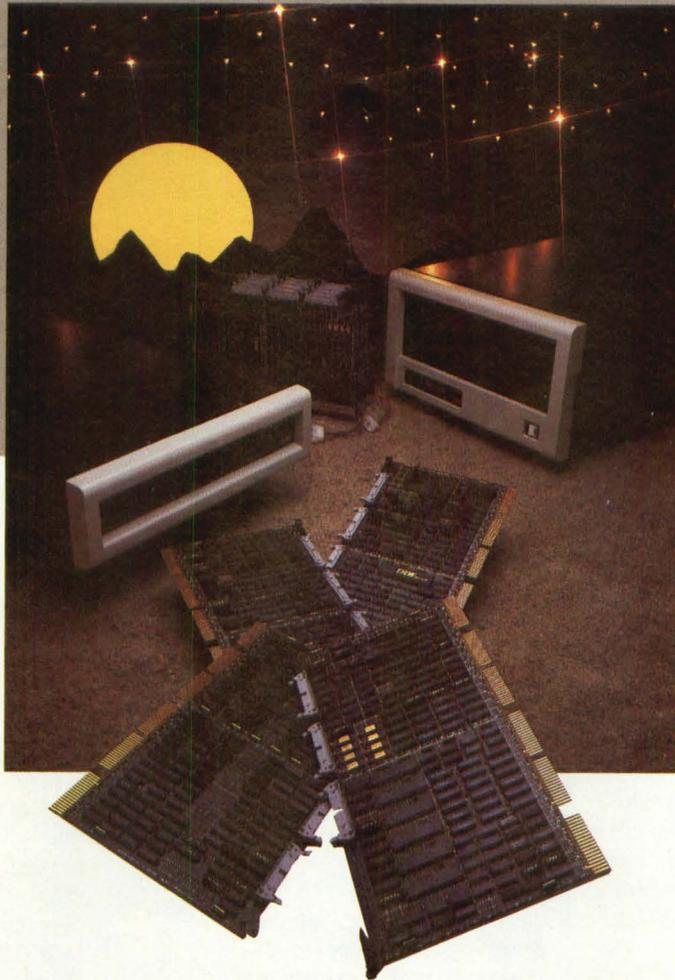
Mini-MAP makes it practical to apply array processing to general-purpose scientific and engineering computing.
