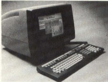
Designed for use with the firm's 932 Supermicro family, as well as with other UNIX-based systems, this color display terminal, the ColorScan 90, allows simultaneous display of up to eight active tasks, each with vertical and horizontal scrolling. Eight background and eight foreground colors display data in 64 combinations. The 12" nonglare screen presents characters and images in 80- or 132-columns. Price is \$1,995. **Data-media**, Nashua, NH **Circle 170**
