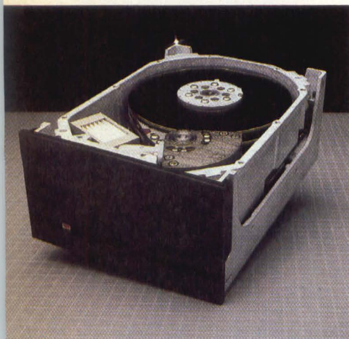
Figure 3: The 1350 Series of drives from Micropolis uses the ESDI, with data separation on the drive.
