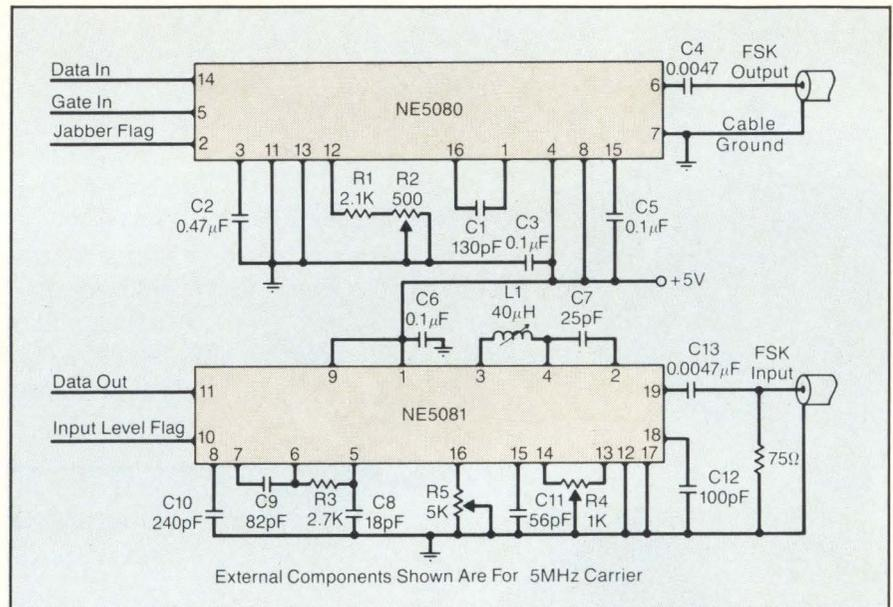
Figure 1: Connection of the NE 5080 and 5081 as a DC to 2 Mbaud full-duplex modem.
