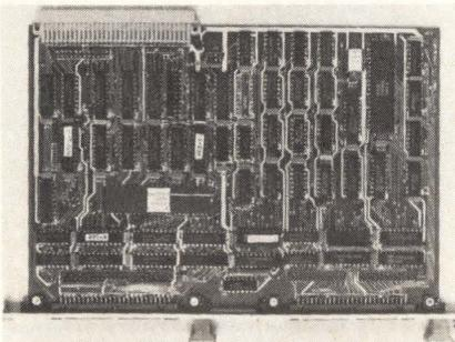
The IoVME-402 is a VME Bus Master which interfaces the VME bus to most 9-track tape drives and has SCSI interface, dual RS-232 I/O ports and vectored interrupts. The interface has an AM9516-based dual channel DMA controller. All DMA functions are programmable and chain loadable including: 24-bit addresses, 16-bit transfer counts, 8- or 16-bit data transfers and byte to word funneling. Price is \$1,850. **Io Incorporated**, Tucson, AZ **Write 192**
