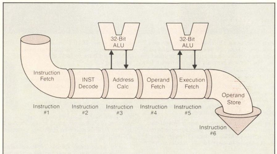
Figure 5: This instruction pipeline will be used in Zilog's new Z80,000 32-bit microprocessor (to be introduced in February 1985). Keeping a pipeline full is critical to exploiting its usefulness.
