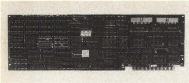
Figure 2, above: Sky Computer's TMS320 based co-processor.
