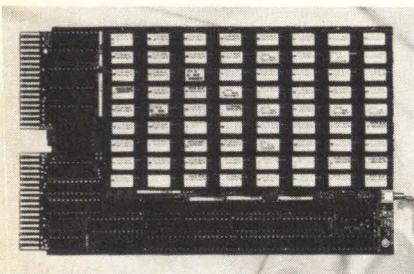
The Pincom 23SX is a 2Mbyte dual wide card for Q-Bus systems. The 23SX uses 64K or 256K of RAM and has block mode, CSR parity, and standard 22-bit addressing. Other features are socketed RAMs, On-line/Off-line switch, LED Run/Error indicator and additional RAM. **Standard Memories**, Santa Ana, CA **Write 182**
