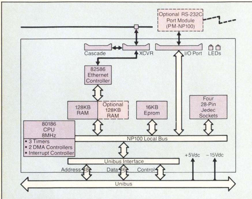
Figure 2: Interlan's NP100 board for Unibus systems, as well as those for other buses and Excelan's 200 series boards, provide Ethernet protocols on board in EPROM. With the power of an 80186 processor and 128 or 256K RAM, host systems are offloaded of communications processing.
