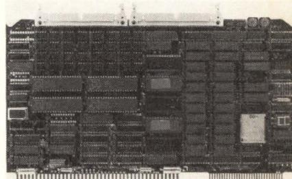
The Am96/3500 is an eight-channel serial communications controller board, featuring an 80186 CPU. The Am96/3500 can operate as a slave controller or a bus master. The Am96/3500 has eight independently programmable serial channels based on the Z8530 serial communications controllers and is compatible with RS-232C and RS-423 protocols. The SCCs can be programmed to handle all asynchronous and synchronous formats. Price is \$2,795. **Advanced Micro Devices**, Sunnyvale, CA **Write 214**
