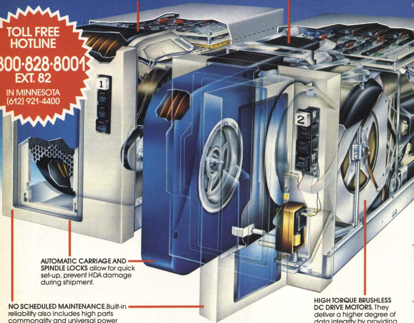
**AUTOMATIC CARRIAGE AND SPINDLE LOCKS** allow for quick set-up, prevent HDA damage during shipment.
