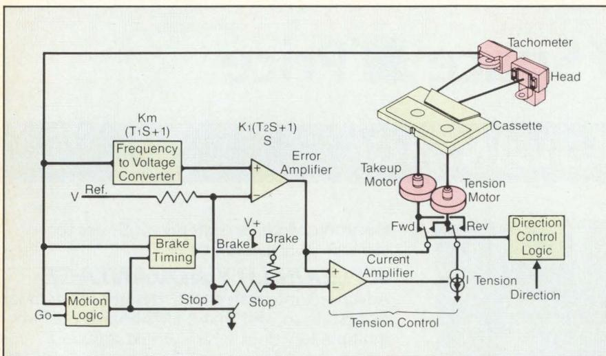
Figure 1: Only four moving parts comprise the design of the drives; tension is electronically controlled.
