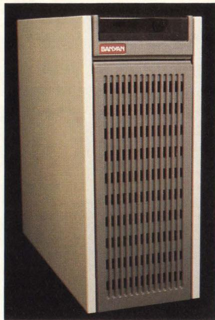
Figure 1: The Banyan Network Server is based on a 32-bit virtual memory processor.
