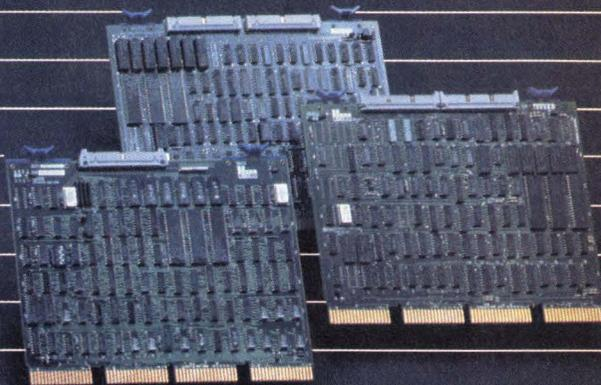
1/2" TAPE—CONTROLLER/COUPLER PERTEC I/O
