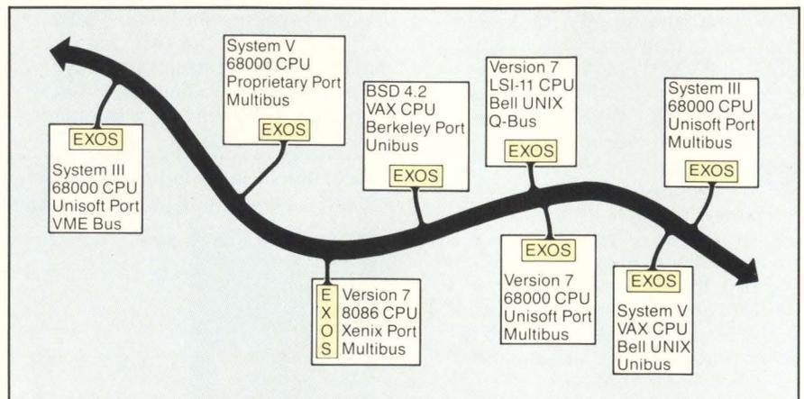
Figure 1: An example of UNIX systems on Excelan's Ethernet using Series 200 front-end processors and their 8010 IP/TCP protocols; file transport, remote copy, login, shell, and electronic mail are available to all users.
