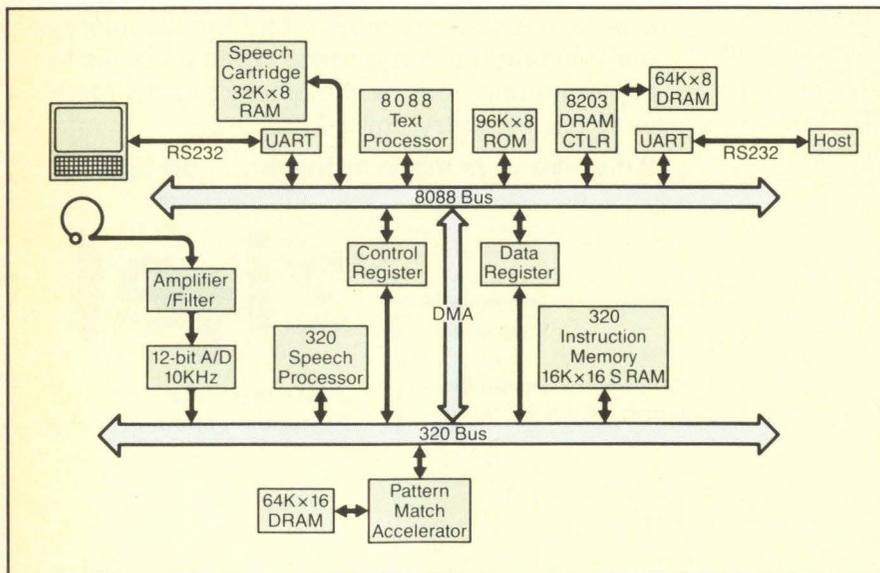
Figure 3: The Verbex Series 4000 block diagram.
