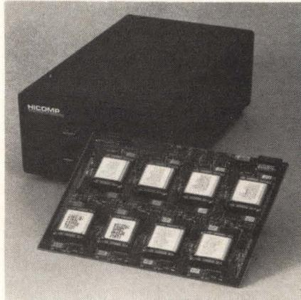
The Bubble Drive is a bubble memory storage board for the IBM PC. It provides either 256 Kbytes for 512 Kbytes of non-volatile, mass storage on a single card which plugs into the PC's I/O slot. It functions as a floppy disk and is fully compatible with PC-DOS 1.1 and 2.0. Standard features include write-protect, boot-enable and a self-installing feature which installs the Bubble Drive software after power-up. Price is \$995-\$1,495. **Hicomp**, Richmond, WA **Write 185**
