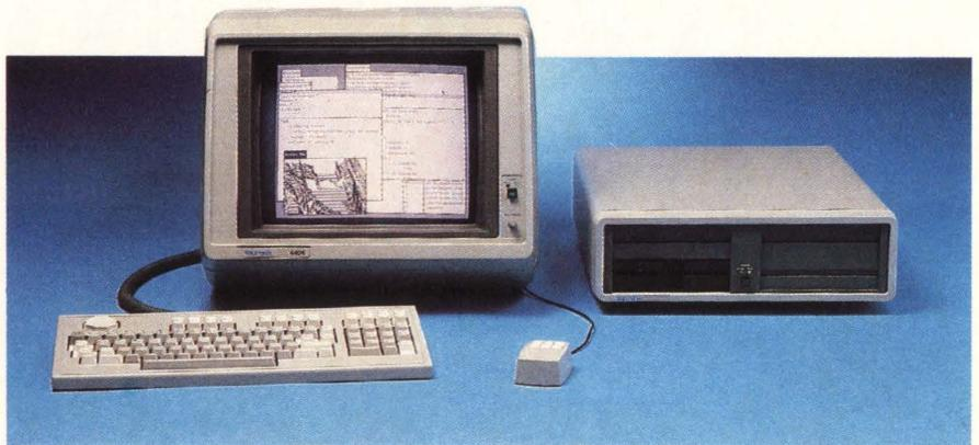
The standard Tektronix 4404 Artificial Intelligence System, listed at \$14,950 (U.S. only), features a monochrome bit-mapped display; keyboard; mouse; 32-bit microprocessor with virtual memory management; hardware floating point; 1 Mbyte RAM; and a 20-Mbyte hard disk with a single 5¼" floppy disk. The system comes with the Smalltalk-80 (a trademark of Xerox Corporation) language, an interactive, graphics-oriented exploratory programming language.
