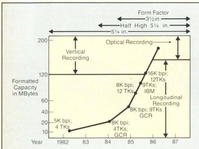
Figure 3: Capacity of digital cassettes has room to grow; by using vertical or optical recording technology, Winchester capacities are rivaled.
