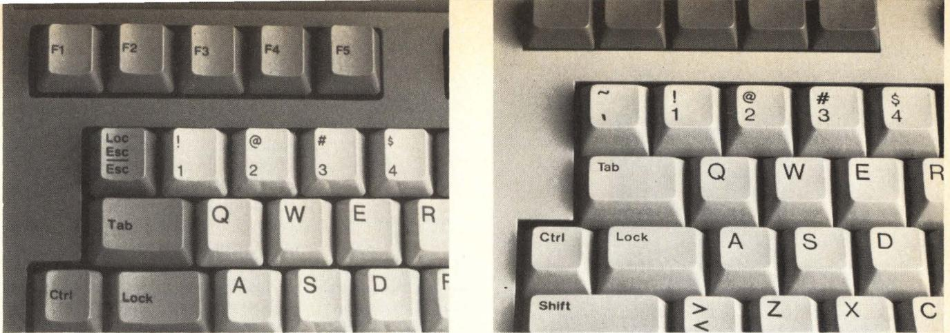
Figure 4: DEC (left) changed the position of the escape key on the newer VT-220 series. Televideo (right), opting for user familiarity with the VT-100 series, decided to retain the escape key position of the VT-100 on their 922, rather than fully emulate the VT-220.
