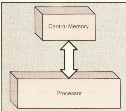
Figure 1: The link between the processor and central memory of a von Neumann computer is known as the von Neumann bottleneck.
