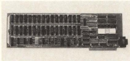
The Chromagraphic I is a color graphic display adapter for IBM compatible personal computers. It provides a 16 color 640 × 408 pixel display at a 60 Hz, flicker free refresh rate. The Chromagraphic I contains an on-board GDC which has been enhanced to draw all color planes simultaneously and to provide replacement and rubberband modes of operation as well as a simplified software interface. A direct drive video port is provided. Price is \$800. **Chromagic**, Milpitas, CA **Write 198**
