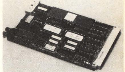
The Gesmpu-4A is a microcomputer board built around the MC68000 16-bit microprocessor. The microprocessor operating at an 8MHz clock rate. Clock frequency is generated by an onboard crystal oscillator. The board has four JEDEC sockets to accommodate 128 Kbytes of EPROM and 16 Kbytes of static RAM. The Gesmpu-4A has a triple 16-bit timer and an RS-232-C serial interface with fully programmable baud rate. Price is \$475. **Gespac**, Mesa, AZ **Write 224**
