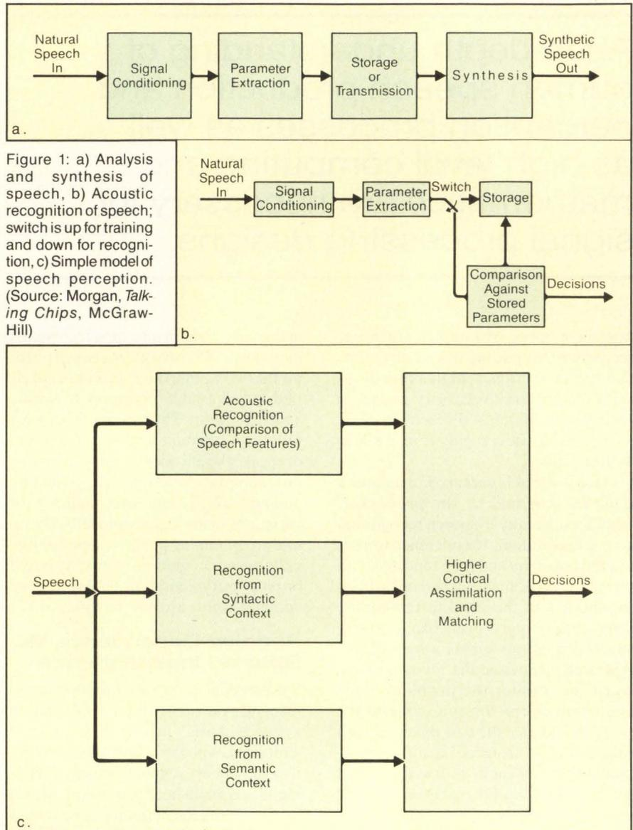
Figure 1: a) Analysis and synthesis of speech, b) Acoustic recognition of speech; switch is up for training and down for recognition, c) Simple model of speech perception. (Source: Morgan, *Talking Chips*, McGraw-Hill)
