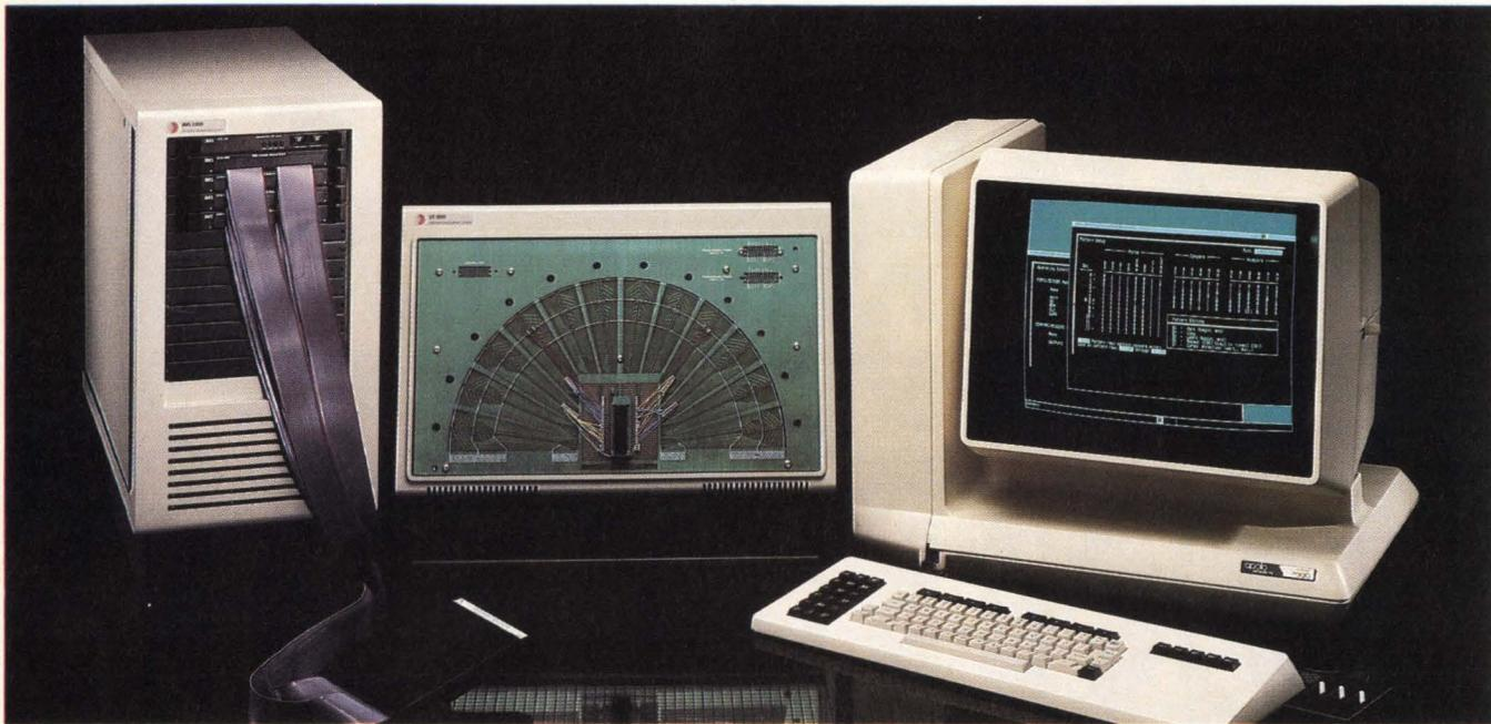
The Logic Master test system interfaces to both engineering workstations and computers. ICs can be functionally tested at speeds up to 40 MHz.
