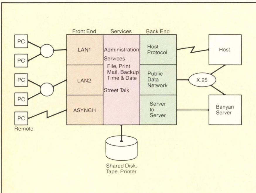
Figure 2: Illustration shows the three functional elements of the network server, which incorporates the three bus structures.
