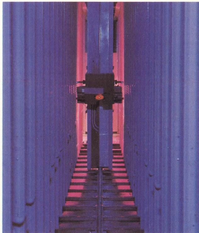
Figure 1: Increased use of automation is improving throughput and quality at many Winchester disk drive manufacturing facilities, and helping to keep more manufacturing plants on-shore. Above, a Litton ToteStacker system moves nearly completed Winchester through a series of final tests at Priam's new automated manufacturing facility in San Jose, CA.
