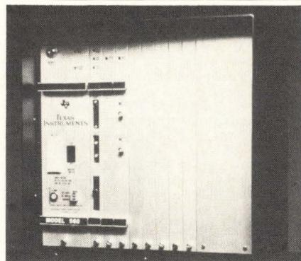
including digital, analog, intelligent, and TIWAY I/O modules. The Models 560 and 565 CPU card(s) can also be programmed via the VPU200 video programming unit. **Texas Instruments**, Dallas, TX
