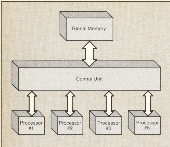
Figure 2: In theory, using multiprocessor von Neumann computers to exploit parallelism seems viable. In practice, however, synchronizing the processors and sharing data becomes very difficult.
