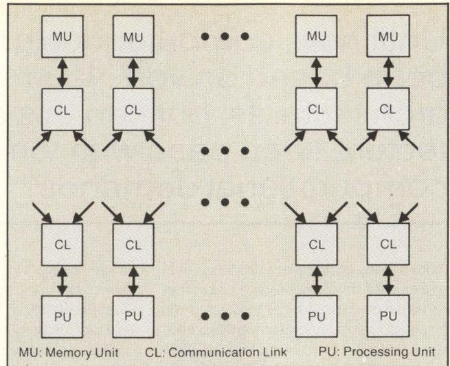
Figure 3: In a scalable multiprocessor system, memory units and processors can be added by simply plugging them together. Increased memory latency, however, is one of the problems with scalable von Neumann machines.
