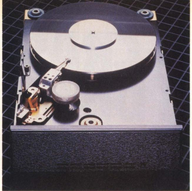
Figure 3: Manufacturers of half-height, 20-Mbyte Winchesters are hoping that IBM's announcement of a 20-Mbyte drive in their PC-AT will create a big market for their drives, just as IBM's PC-XT created a huge demand for 10-Mbyte Winchesters. Cogito's PT925, shown here, is designed for portable applications, and features Whitney-style mini-slider heads, thin film media, and 12-watt power consumption.
