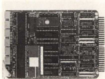
The ZT8806 is an 8088-based processor board for automation applications. MAX mode operation allows the addition of the 8087 Numeric Data Processor using Intel's iSBC 337 piggyback processor option. Five 28-pin byte-wide JEDEC memory sockets provide space for up to 64 Kbytes of PROM and 32 Kbytes of static RAM. The I/O capabilities include one serial port, 5 counter/timers, two 8-bit parallel I/O ports, and an interrupt controller. Price is \$465. **Ziatech**, San Luis Obispo, CA **Write 210**
