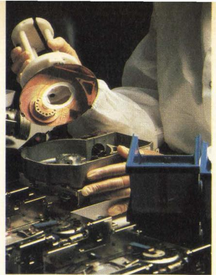
Figure 5: Despite the growing demand for thin film media, iron oxide disks, like this one being installed into a Seagate 5 1/4" Winchester, are still the most popular media for rigid disk drives in all size categories. (Photo courtesy Seagate Technology.)
