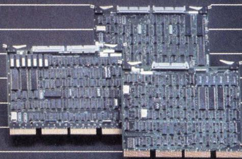
1/2" TAPE—CONTROLLER/COUPLER PERTEC I/O
