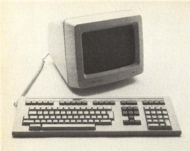
Figure 6: The DEC VT-220 text-only terminal is the newest successor to the VT-100, which is easily the most emulated terminal in the industry.
