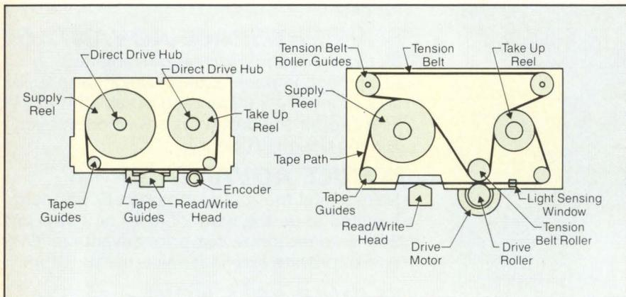
Figure 2: The D/CAS cassette is only 4" x 2 1/2" x 7/16", compared to 6" x 4" x 11/16" for a standard tape cartridge.
