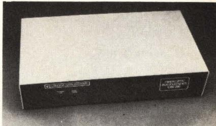
The CBE-202 Fiber Optic Interprocessor Link comprises a parallel-to-serial multiplexer and a Bus Interface Module (BIM) which plugs into DEC PDP and VAX backplanes. A duplex fiber optic cable links the two multiplexers. The link operates at 250 kilowords/sec and can be as long as 2 kilometers. The Bus Interface Modules are software compatible with the DEC DR11-B or DR11-W modules. Price is \$4,500. **Canoga Data Systems**, Canoga Park, CA **Write 177**
