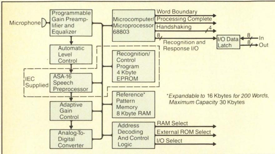
Figure 2: Interstate Voice Products' VRC100-2 simplified block diagram.
