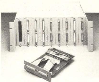
mount chassis which supports eight plug-in I/O modules. Up to eight chassis may
