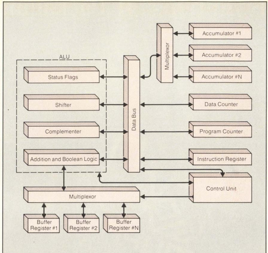
Figure 4: Multiple buffer registers and accumulators enable the processor to concurrently perform several tasks.
