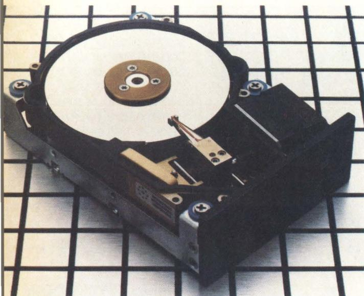
Figure 2: A big future is forecast for small, sub-4" Winchesters, especially those that prove to be reliable in harsh environments. This Microscience drive features plated media, closed-loop positioning and linear actuator to maintain data integrity under adverse conditions.
