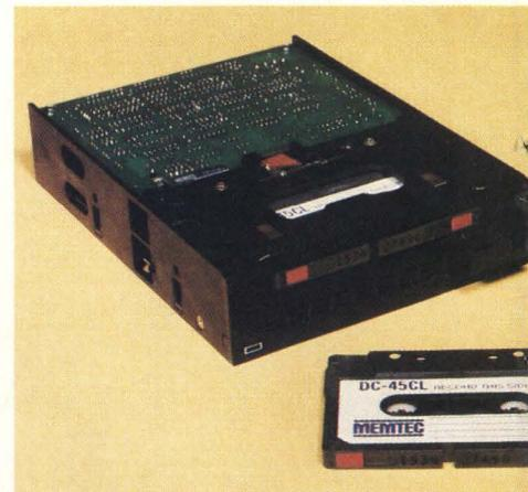
Memtec's Companion 400 half-height series uses compact cassette recording media for 10, 20 or 40 Mbytes of storage.
