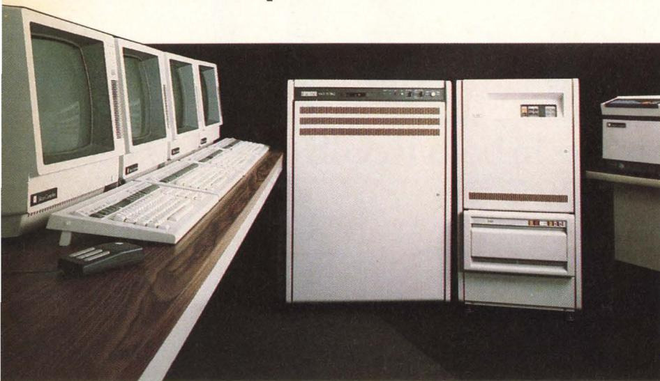
The Genesil Silicon Development System is made up of a VAX 11/750-based turnkey system running under UNIX, supporting up to four users and offering user I/O options.
