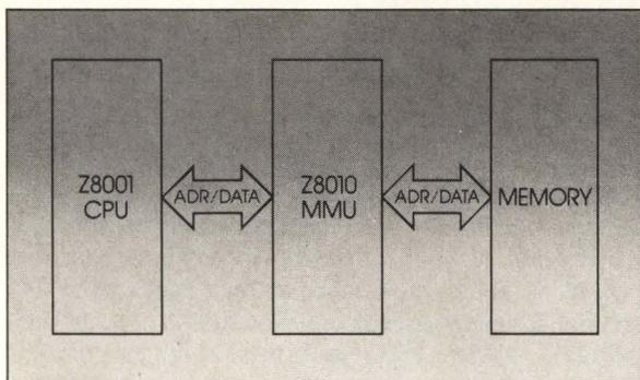
Zilog's configuration system prevents the Blue Sky Phenomenon by inserting a chip called the Z8010 Memory Management unit between the processor and memory.
