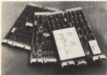
The 1114AD is a Q-Bus compatible 1114AD board which has 8 software programmable ranges from 10mV full scale to 10V full scale. The 1114AD has unrestricted mixing of high and low level signals plus 12-bit resolution. For fixed and changing I/O environments, the 1114AD has software selection by channel of thermocouple type, RTD, load cell and strain gauge inputs. Companion boards provide expansion to 128 channels with 250V common mode protection. **Adac**, Woburn, MA **Write 213**
