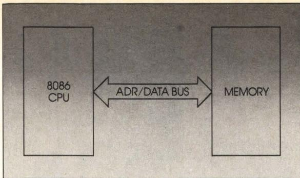
A typical Intel 8086-to-8088 configuration, the lack of memory checking hardware—the memory to the processor. The processor can change any area in its memory at will, without regard to the consequences. The result: illegal operations cannot be detected before damage has occurred; and any damage to the program and data cannot be undone.
