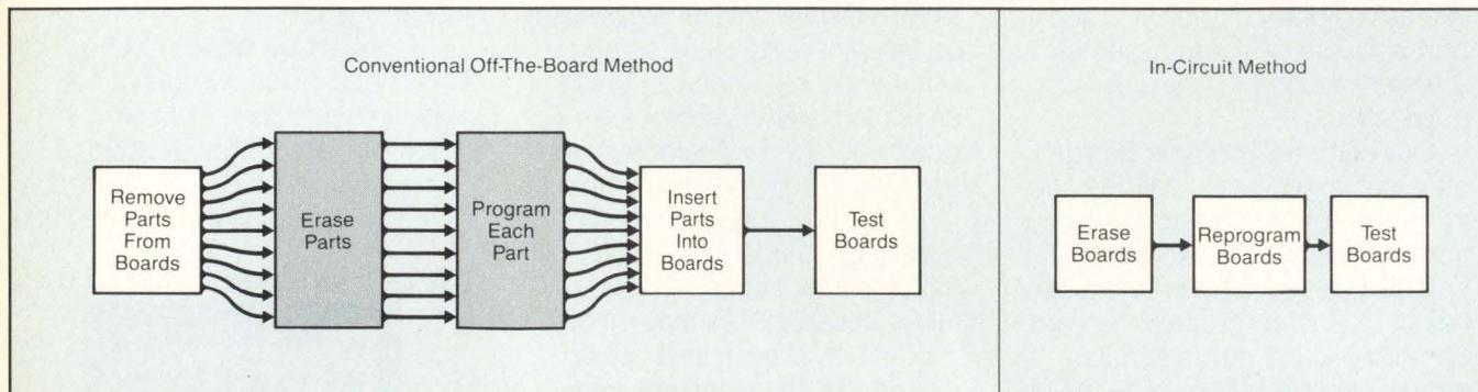
Figure 3: Reprogramming memory boards, comparing off-the-board method to in-circuit method.
