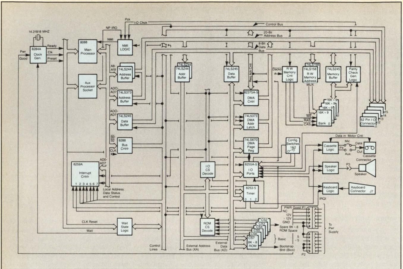
Figure 4: System board diagram of the IBM PC. The board can support either 16K to 64K or 64K to 256K of RAM.
