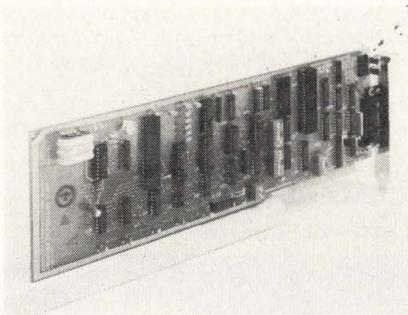
The Advanced Communication Controller allows communication with other computer systems using different protocols. The board allows communication rates of 19.2 K and optional features include, an IBM-PC compatible printer interface, and a real time clock. Design features include multiple protocol support, DMA interface and interrupts, intelligent communications controller chip (Z80 SIO), and a parallel port option. **Frontier Technologies Corp.**, Milwaukee, WI **Write 201**
