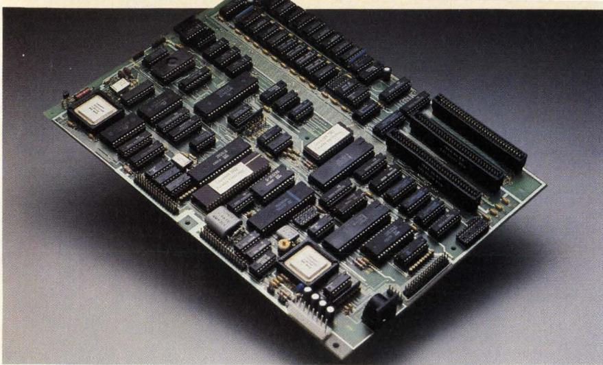
Figure 9: The FE6413 is a single board computer from Faraday Electronics compatible with the IBM PC which has either a floppy disk or monochrome display controller option.
