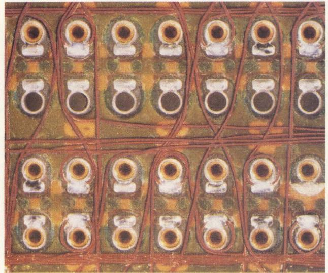
boro, MA). The concept bridges the gap between wire wrap and multilayer printed circuit boards. Computer storage of design information used in conjunction with premanufactured board modules allows new designs to be started in wire wrap for prototyping and converted directly to Unilayer 11 wiring for production requirements, thus eliminating the cost and time normally associated with production redesigns.
