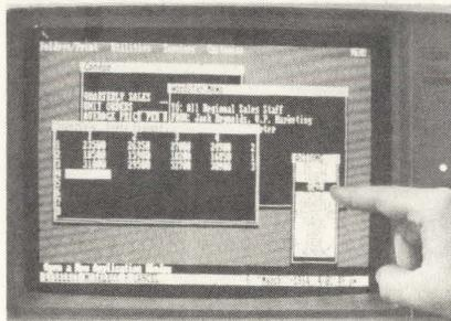
The Point-I Color Kit includes a 13" diagonal touch screen, intelligent controller and an RS-232C serial interface. The screen, available for the IBM PC color monitor is fully programmable and supported by software development tools. With the screen, users can select from menus, position the cursor and create and manipulate graphics by touching the IBM Color Monitor with a fingertip. Price in OEM quantities is \$650. **MicroTouch**, Woburn, MA **Write 178**
