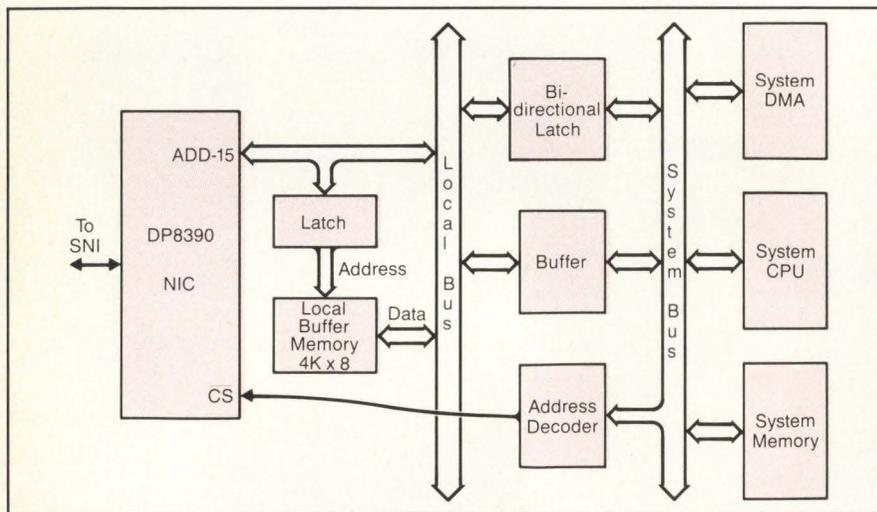
Figure 1: A few low cost external components is all that is needed to interface the NIC to the host system with local memory. Even the control signals for the buffers and the latches shown are provided by the NIC. A direct interface to the system bus (without a local memory) requires even fewer components.
