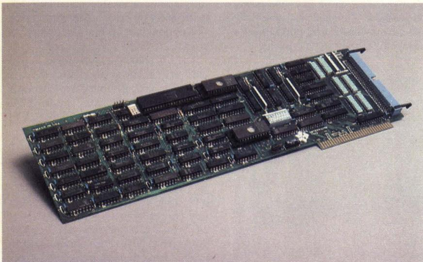
Figure 5: Interphase Corp.'s Maverick SMD PC-80 is a rigid disk controller which allows the PC to support the SMD interface.
