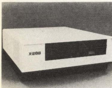
The X-286 is a desktop supermicro-computer which implements the XENIX operating system on Intel's 80286 processor. The basic configuration supports five users which is
