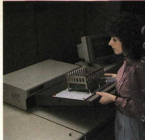
The new generation of in-circuit programmers makes changes between programmable boards as easy as changing adapter bases. (Photo courtesy Data I/O).
