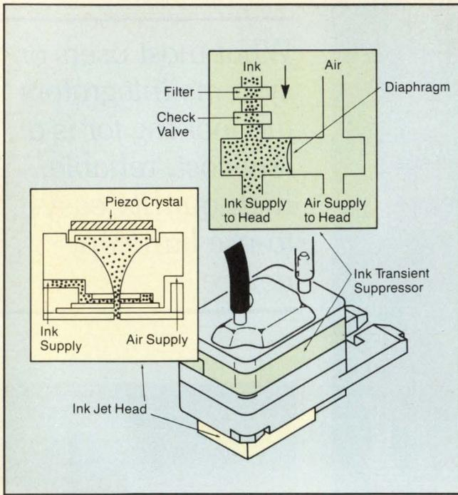
Figure 4: The ink transient suppressor from Tektronix uses a five micron mesh filter to trap bubbles and particles that may have worked their way into the ink system. A one-way valve prevents ink from flowing away from the ink jet heads, and a flexible diaphragm, exposed to air on one side and ink on the other, suppresses shock when the copier is jolted and moved.
