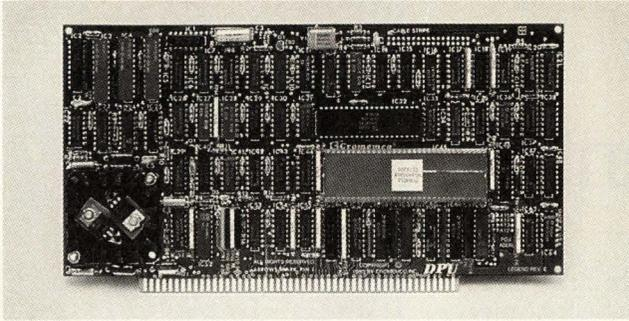
Cromemco's dual processor card features a 68000 and a Z80.
