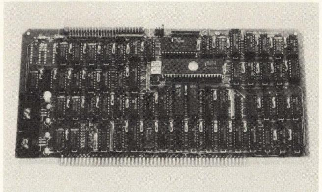
Adaptec's Intelligent host adapter, the AHA-1510, supports the S-100 bus.
