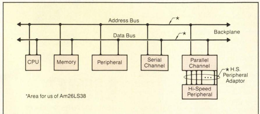
Figure 2: Am26LS38 utility in a processor complex.
