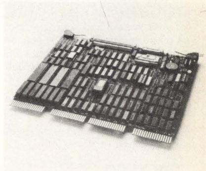
The Model DQ215 Winchester disk controller interfaces two 8" and/or 14" SMD I/O compatible drives to LSI-II thru 11/73 and MICRO/PDP-II computers. The quad module operates when it is plugged into one Q-Bus slot and connected to drive(s) by flat cables. The controller has universal formatting, 56-bit ECC, 22-bit addressing for 4 Mbyte data access and is compatible with RT-II, RSX-II and RSTS operating systems. Price in quantities of 50 is \$1,150. **Dilog, Garden Grove, CA** **Write 206**
