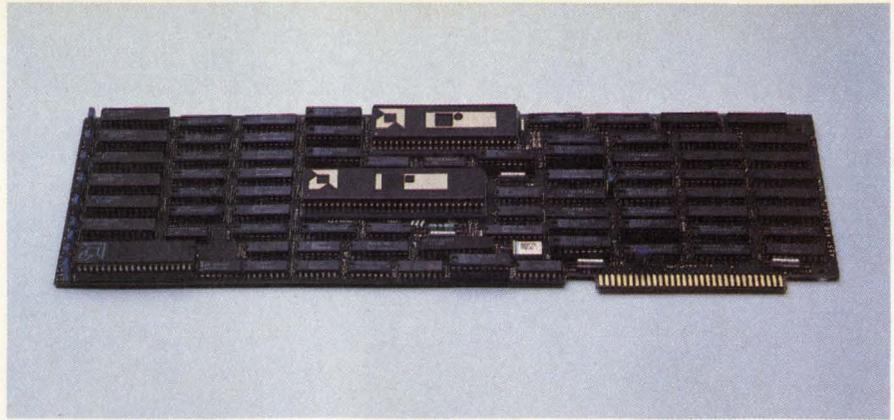
Figure 7: Utilizing a 16-bit AM29516 eight MHz parallel multiplier, the Marinco APB-3024 PC adds array processor functions to the IBM PC.
