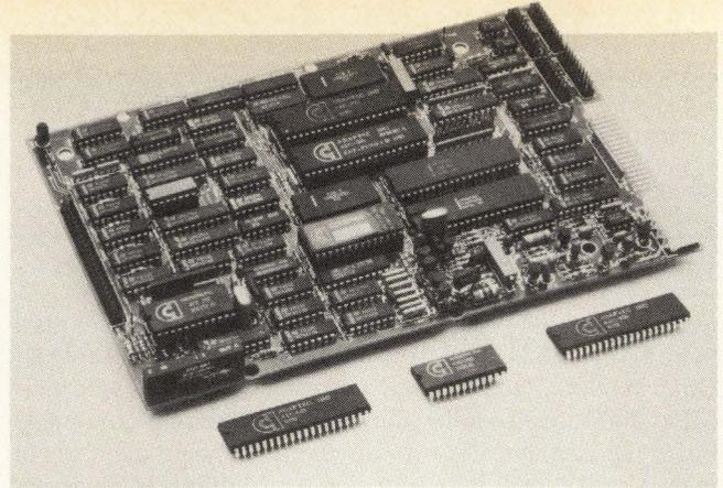
Adaptec's ACB-550 5 1/4" Winchester disk controller with SASI/ANSI SCSI support.
