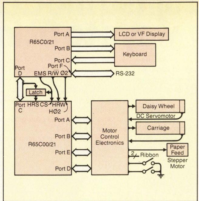
Figure 2 (above): Typewriter/Telecommunications system with dual processor host and peripheral controller.
