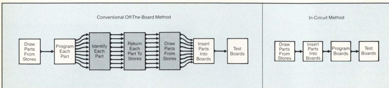
Figure 2: Comparing the manufacturing steps required for the off-the-board and in-circuit programming methods.
