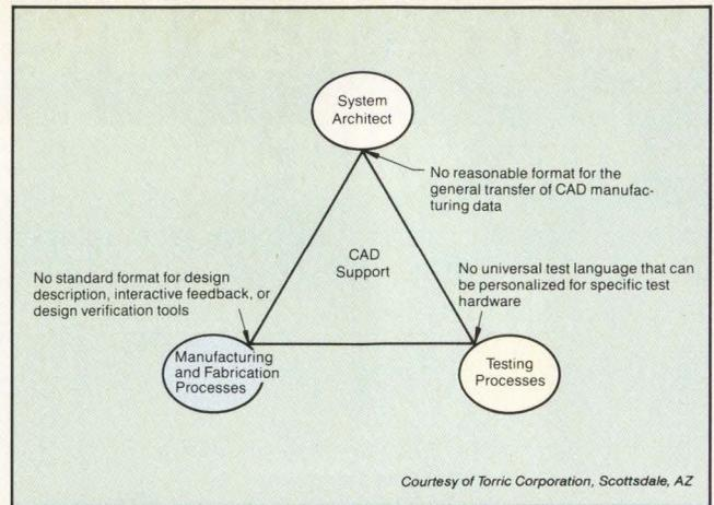
Figure 4: Three interfaces in the design environment that are presently lacking in definition.
