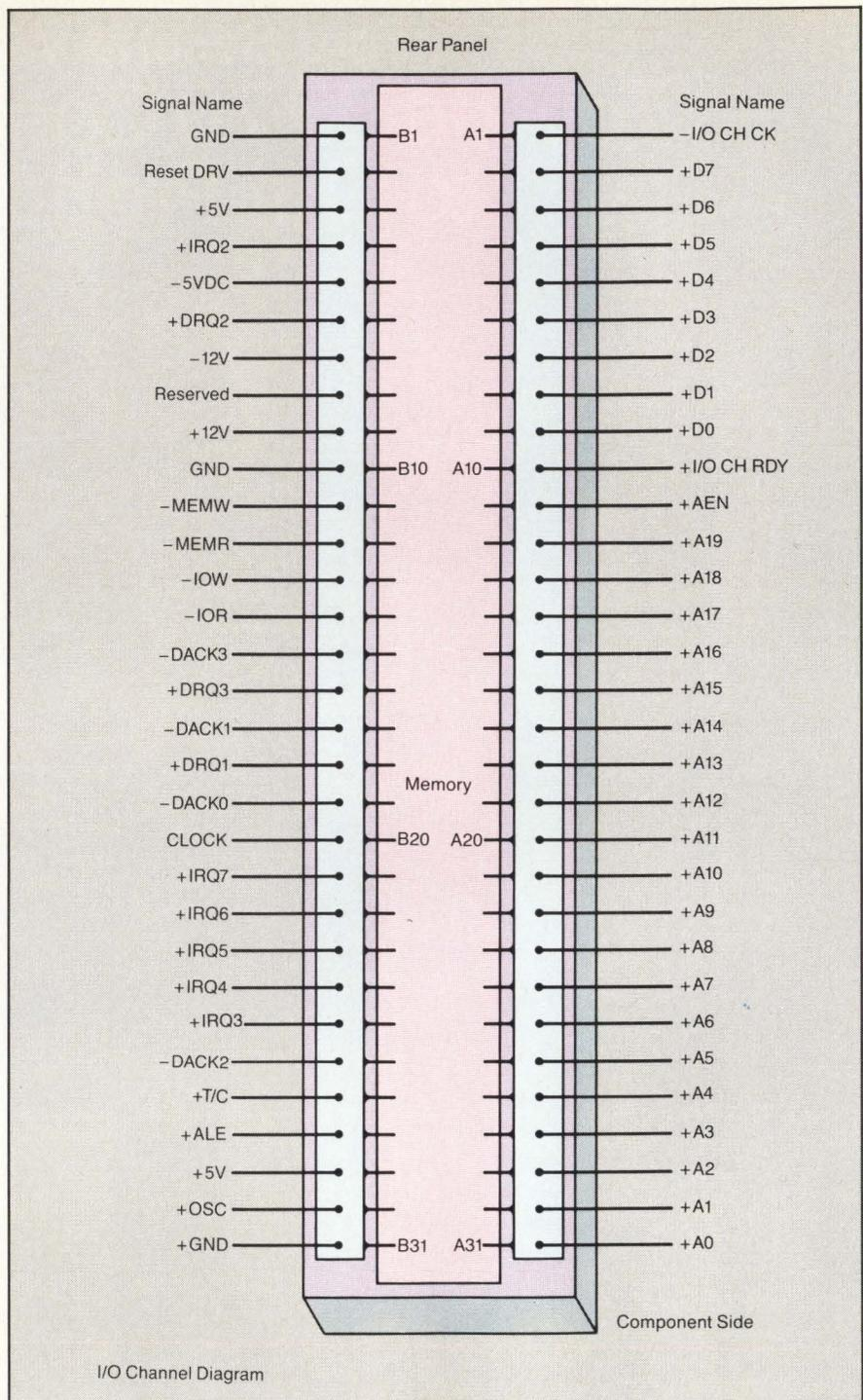
Figure 6: Diagram of the I/O channel which is an extension of the 8088 microprocessor bus. The I/O channel is bused across the system's five I/O slots.
