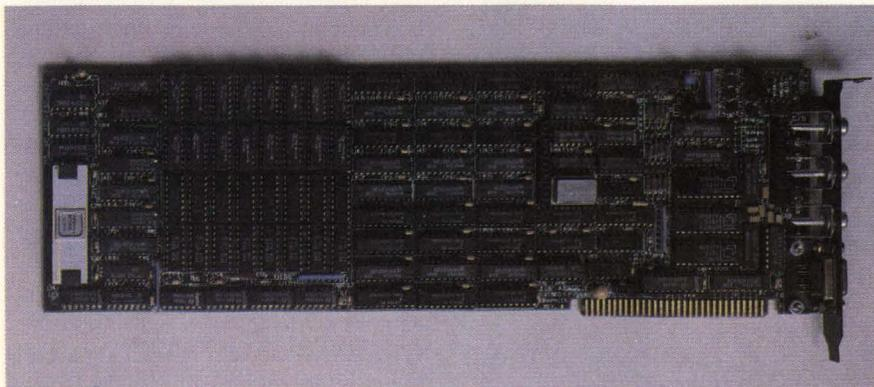
Figure 3: Featuring the NEC 7220 chip and 128K of memory, the IDEAgraph color graphics board from IDEAssociates allows the PC or XT to be used in CAD/CAM applications.
