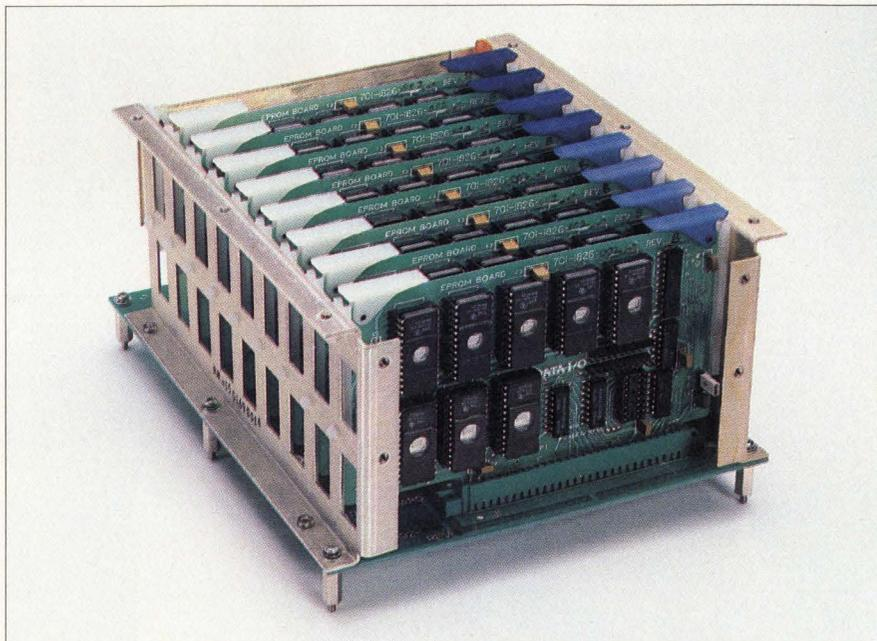
Figure 1: Data I/O's interface fixture holds up to eight circuit boards for simultaneous programming.
