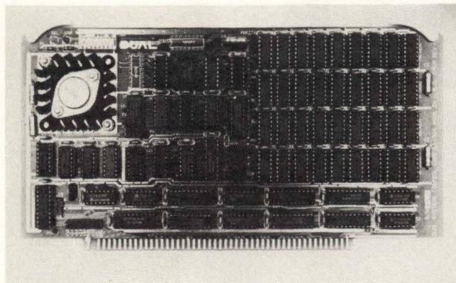
Dual Systems (Berkeley, CA) 1 Mbyte RAM board makes use of 256 Kbit devices. Access time is 220 ns.
