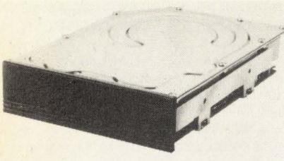
The MR522 5 1/4" Winchester disk drive has 25.50 Mbytes of unformatted capacity, 6.37 Mbytes per surface and 10,416 bytes per track. The MR522 has an industry-standard transfer rate, recording format and controller interface requirements, and consumes 18 watts of power. The drive has two platters, four data surfaces and four magnetic data heads. Price is \$875 in OEM quantities. **Mitsubishi**, Torrance, CA **Write 171**
