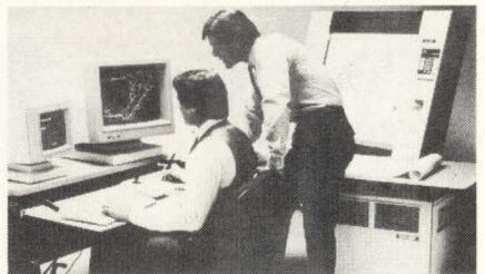
The System 25 is a CAD system with a 32-bit central processing unit, distributed processing and a modular building approach that enables system expansion. The system can be organized into single-user, stand-alone, multiuser or mainframe-based configurations. The main design station consists of two displays, a 12" alphanumeric screen and a monochrome or color graphics screen. Price is \$65,000. **Calcomp**, Anaheim, CA **Write 146**
