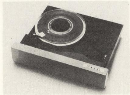
The PCT-1000 is an IBM-format compatible 9-track streaming tape drive, that provides backup of 138 Mbytes for Winchester hard disks, read/write access to archival data banks, and intercomputer data interchange. The PCT-1000 can handle formats including 800 NRZI, IBM and ANSI; 1600 cpi PE, IBM and ANSI; and dual-density, 3200/1600 cpi. Price is \$2,256. **IBEX Computer Corp.**, North Hollywood, CA **Write 176**
