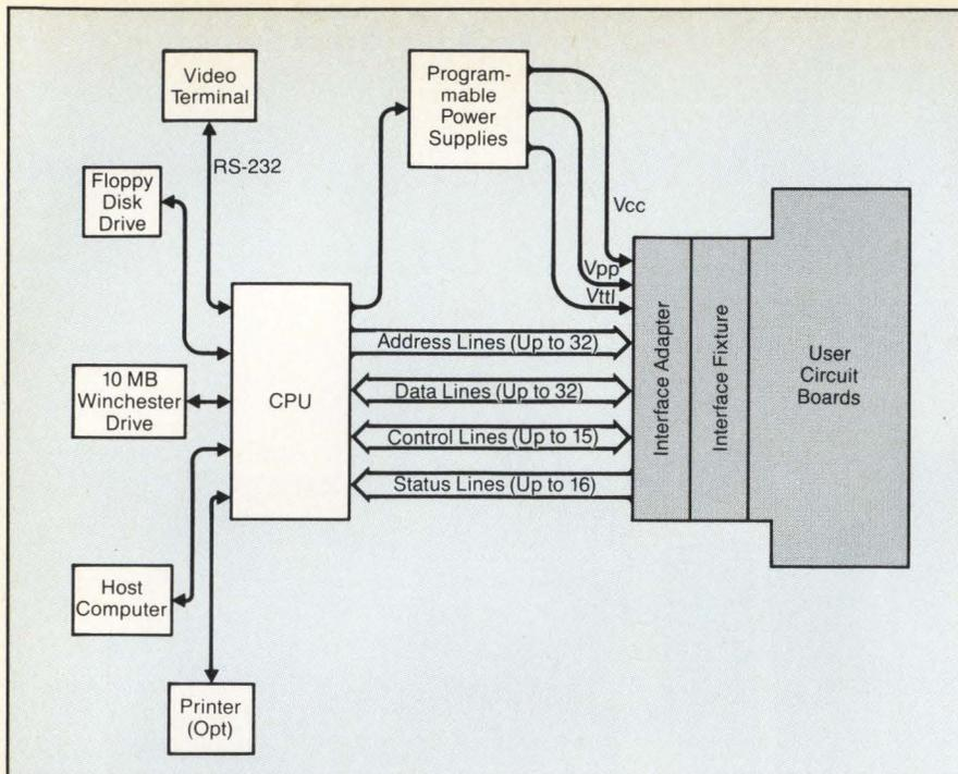
Figure 4: Block diagram illustrates the internal structure of the in-circuit programming system.
