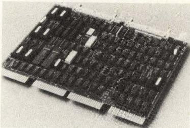
The TC13 tape coupler connects industry-standard 1/2" tape drives to DEC PDP-11 and VAX-11 systems. Tape data rates of 781 Kbyte cps are
