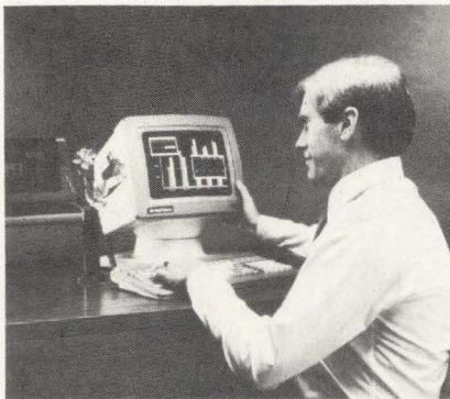
The 925E terminal provides 925 compatibility. The 925E meets DIN standards, has a tilt and swivel screen, a buffered printer port and 16 function keys that can be shifted to 32. An optional graphics board is available. Price is \$795. **TeleVideo Systems, Sunnyvale, CA. Write 175**
