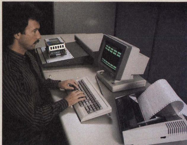
Figure 1: The Data I/O Model 156A In-Circuit Programming System.
