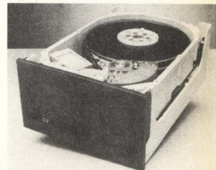
Models 1353, 1354, and 1355 are Winchester disk drives with capacities of 85, 127, and 170 Mbytes, respectively. The series is compatible with drive controllers available from major controller firms and average access times are less than 30 msec. Prices, respectively, are \$1,469, \$1,669, and \$1,837 in OEM quantities. Evaluation units will ship in the fourth quarter of the year. **Micropolis Corp.**, Chatsworth, CA
