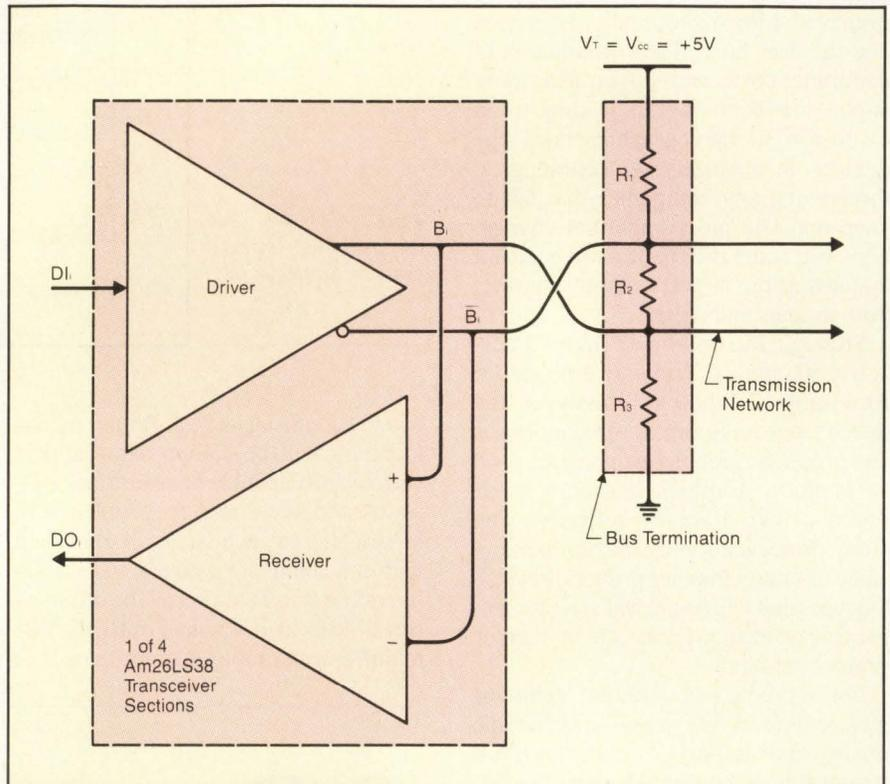
Figure 1: System connection diagram.
