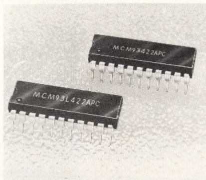
The MCM93422A and MCM93L422A are 1024-bit bipolar RAMs with access times of 35ns and 45ns, respectively. The parts have a power dissipation of 0.26 mW/bit and provide 3-state outputs to drive bus-organized systems and/or highly capacitive loads. The series is TTL compatible and is offered in JEDEC standard 22-pin, 400 mil wide plastic or ceramic packages. Price in quantities of 100 is \$9.50 (plastic), and \$10.76 (ceramic). **Motorola, Phoenix, AZ** **Write 188**
