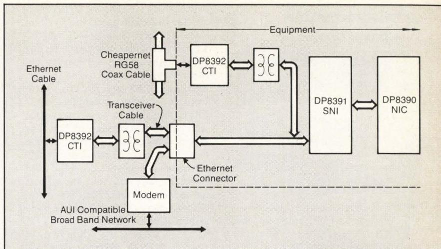
Figure 2: By incorporating the CTI along with the other two chips within the data terminal equipment, the user can be provided with the option of using either the Cheapernet or the Ethernet or the Broadband network.
