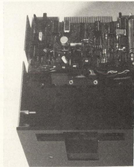
Tape drives to the D/CAS standards, like the Memtec Companion 500 Series, fit into a standard 5¼" form factor and hold 10 or 20 Mbytes.
