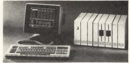
The B25 desktop microcomputer system supports clusters of up to 32 B20 and B25 workstations. The basic system includes a central processor with 256K RAM, 12" display, keyboard and a dual floppy disk storage module. A 10-million byte floppy/hard disk peripheral is available as an option. The system can also be expanded to 40 Mbytes. Price is \$4,000. **Burroughs Corp.**, Detroit, MI **Write 138**
