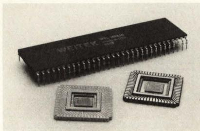
Available on leadless chip carriers and 64-pin DIPS for even lower power-consumption and broader interfacing alternatives, the new chips undergo an exhaustive proprietary burn-in process that assures reliable performance.
