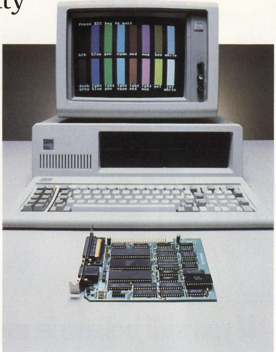
Figure 1: The Hercules color card from Hercules Computer fits into one of the IBM XT's short expansion slots.
