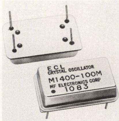
These Crystal Clock Oscillators are for commercial or industrial applications and are available in frequencies of 10 to 125 MHz. The metal package is hermetically sealed by resistance weld, with a glass-to-metal seal connector which may be soldered or plugged into a socket. The oscillators have monolithic ECL 10,000 outputs and come in fourteen models that cover .0025% thru 1.0%. **MF Electronics, New Rochelle, NY** **Write 200**
