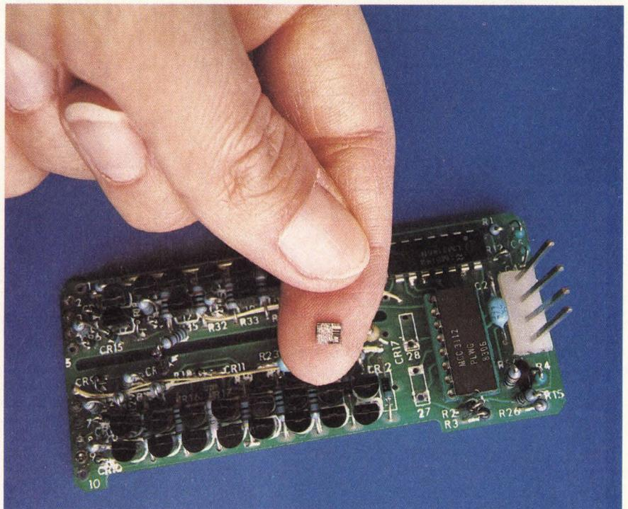
*The many functions now performed by discrete devices, logic circuitry and relays are combined on a single chip.*
