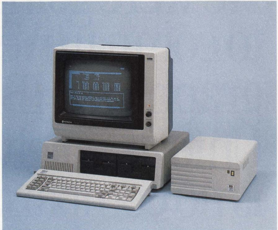
Winchester disk StorageMaster™ subsystems from Control Data provide 18 or 30 Mbytes of storage to the IBM PC.
