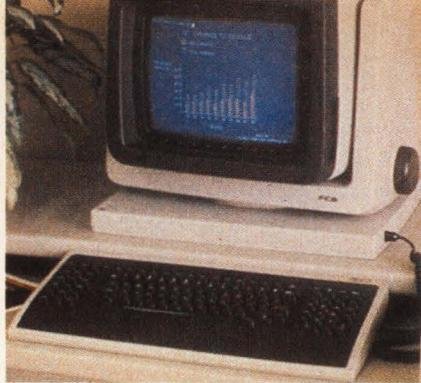
The Florida Computer Graphics Beacon terminal line was one of the first to incorporate both 16/32 bit processors and second generation bit slice devices.
