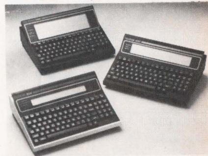
The T-4000 and T-5000 are two portable computers which are battery-operated and have 256 Kbyte non-volatile bubble memories. The T-4000 has an 8-line x 80 character LCD and weighs nine pounds. The T-5000 has a 16 line x 80 character LCD and weighs ten pounds. Both models fit into a briefcase and have alphanumeric keyboards
