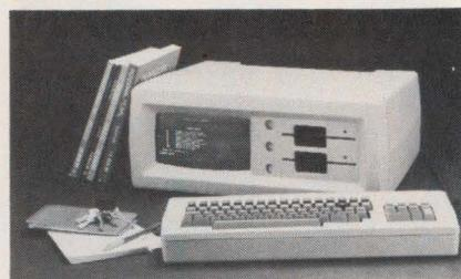
The MD3 is a CP/M-based portable computer which includes two floppy disk drives and eight software packages. Features of the MD3 include 64 Kbytes of RAM, two double-sided, double-density, 5.25" floppy disk drives (400 Kbytes each), a 5 x 9" monitor with an 80-character by 24-line display, two ports, a detachable keyboard, and character-map graphics. **Morrow**, San Leandro, CA **Write 138**
