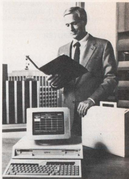
The Apricot is an 8086-based IBM-compatible 16-bit microcomputer. It has 256 Kbytes of main memory, three operating systems (MS-DOS, CP/M-86 and concurrent CP/M-86) and 3.5" Sony MicroDrives, each with 315 Kbytes of storage. The Apricot also includes an integral calculator and bundled executive software. An 80-character MicroScreen is built into the keyboard and displays two 40-character lines. Price is \$2,495., **ACT**, Santa Clara, CA **Write 132**
