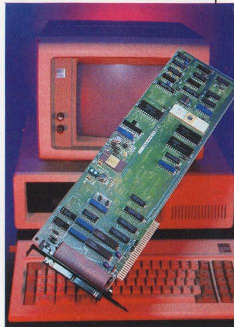
*Figure 1: The DT2808 brings low cost analog and digital I/O functions to the IBM PC. This single board peripheral fits in one of the host computer's expansion slots.*
