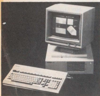
The T300 Computing System includes a 192K computer with Intel 8088 microprocessor, 640K 5-1/4" floppy disk drive and a 12" green screen display. The system includes a 10 Mbyte hard disk, a memory expansion to 512K, a clock/calendar, and a 16 color palette. The 12" monochrome display has a resolution of 640 x 500 and the same feature is included on the optional 14" color display. Price is \$2,495. **Toshiba**, Tustin, CA **Write 136**
