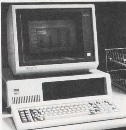
The Color IV is a high-resolution color monitor compatible with the IBM Personal Computer and DEC Rainbow computers. It is available in two versions with either RGB analog or digital input. The monitor, using a separate interface, will display 16 colors and will accept the RS 170A, RGB signal of the DEC Rainbow. The monitor has 720 x 420 resolution and a .31mm dot pitch CRT. The unit has a 96 x 24 character display. Price is \$995. **Amdek Corp.** Elk Grove Village, IL **Write 128**
