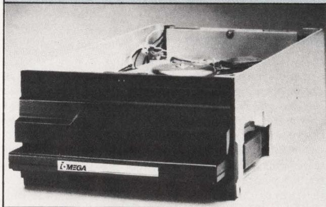
Figure 5: In addition to their standard Alpha-10 8" flexible disk drive, storing 10 Mbytes on a cartridge, Iomega now builds a 10.5 Mbyte version compatible with DEC's RL02.
