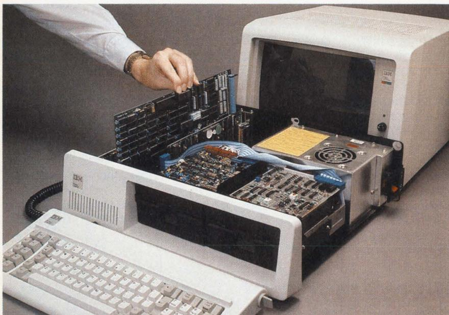
*The first SMD rigid disk interface controller board for the PC is Interphase's Maverick SMD PC-80, shown here being inserted into an IBM system.*
