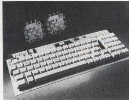
The KS-200E keyboard is designed with patented twin bifurcated contacts and has a rated life of 50 million cycles. The KS-200E is available with tactile or linear feel. Keys have a .120" stroke and typical bounce is less than one msec, with a five msec bounce over the switch life. The KS-200E is available as discrete switches or arrays assembled with or without keycaps, or assembled and soldered to a PC board with or without electronic encoding. **Stackpole Components**, Farmville, VA.
