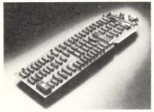
The Color/Graphics Monitor Adapter Board provides color display and graphics capabilities output for the Eagle PC, Eagle 1600 Se-
