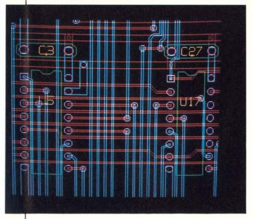
Figure 2: A Zoom closeup of a completed routing scheme.
