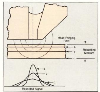
Figure 3: Thin-film (a): less head fringing and a higher-amplitude recorded signal than thicker media (b, c). (Courtesy Evotek).
