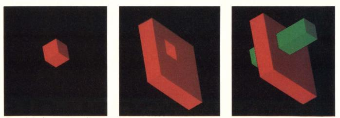
Figure 4: Boolean operations allow users of SM systems to manipulate geometric shapes quickly. An intersection of plane and block is performed to perforate the plane, or to create the volume of the intersection in this example.
