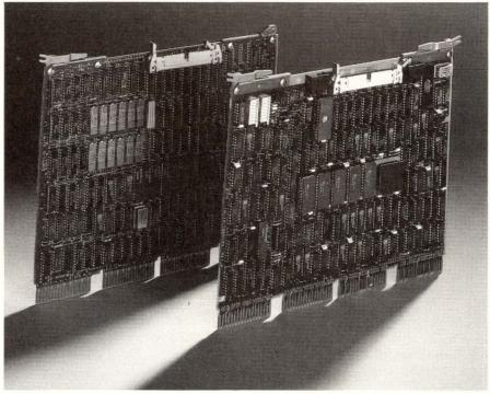
These two boards constitute the CPU of Digital Equipment Corp.'s MicroVAX-1.
