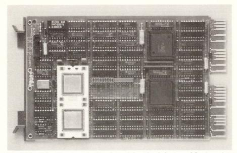
The 11/73 will be offered as a dual height module and includes integral floating point instructions.
