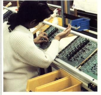
Worker assembling minute pieces of PABX (private branch exchange) circuit boards. Circuit boards, the mainstay of the system, can be programmed to handle thousands of calls each hour.
