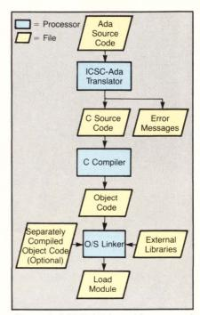
Figure 1: ICSC-ADA enables users of Gould CONCEPT/32 computers to learn ADA and develop ADA programs to satisfy emerging requirements of military and scientific computer applications.
