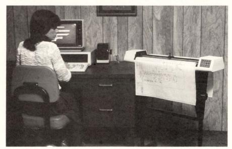
Figure 2: The Houston Instruments DMP-41 drum type pen plotters can accommodate large size papers.
