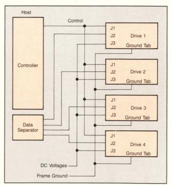
Figure 12: This diagram depicts a typical four-drive ST412HP system. Note that unlike the ESDI, the data separator is not on the drive.
