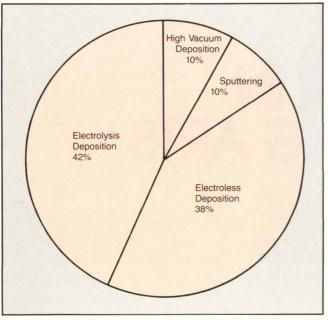
Figure 2: According to a survey conducted by Memorex, 29 companies manufacture thin-film media, using four processes.
