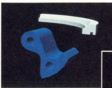
▲ Figure 5: Techniques of software editing include operations of revolution shown in white and extrusion in blue. Both types of operations allow 2D planar outlines to be translated across space to quickly generate solid parts.
