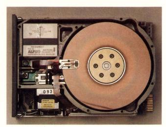
Figure 8: The positioning system on Seagate's 12.76-Mbyte ST412 uses a split-band actuator and a stepper motor for an average access time of 85 msecs.
