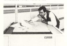
The Versatec electrostatic remote plotting system emulates HASP and 3780 workstations, and supports binary synchronous communications protocols under DEC VAX/VMS, RSX-11M/M-Plus or RT-11 operating sytems. It includes a remote plotting controller, random element processor, and electrostatic plotting software. The random element processor handles plot data ordering and rasterization and the disk-based processors support remote color plotting. Price is \$6,500. Versatec, Santa Clara, CA Write 160
