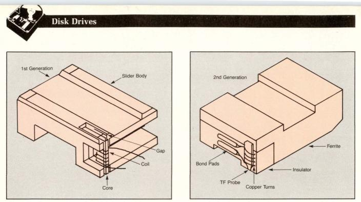
Figure 7: The vertical-recording R/W head at left is a narrow-gap composite head manufactured using conventional techniques. The "probe-style" head at right can be made using thin-film processes. (Courtesy Applied Magnetics).
