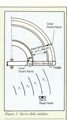
relationship of bit sync information. Because the dual-frequency method uses a relative amplitude difference of f1 and f2 frequencies, servo head azimuth alignment is not critical, thus reducing production costs and service requirements.
