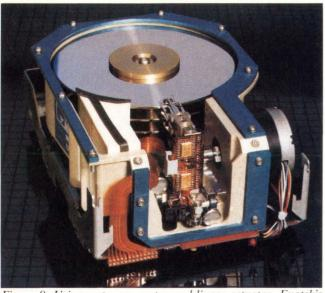
Figure 9: Using a stepper motor and linear actuator, Evotek's 5000 series drive provides an average access time of 49 msecs.
