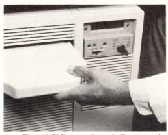
The 11/725 uses Digital Equipment's own 26 Mbyte fixed/26 Mbyte removable technology.
