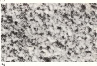
Figure 1: Although ferrite and thin-film disks look equally smooth to the naked eye, these 40,000X electromicrographs reveal that thin-film media (b) is smoother and more uniform than particulate iron oxide media (a). (Photos Courtesy Memorex).
