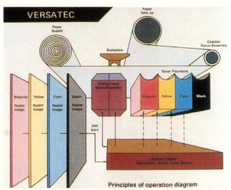
Figure 4: Versatec's color electrostatic plotter—principle of operation.
