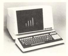
The GO-140 is an integrated alphanumeric/ graphics terminal which emulates the DEC VT100 and Tektronix 4010 series of terminals. Its alphanumeric features include 24 lines of 80 or 132 characters, selectable sta-
