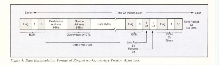
The ring interface operates in two modes: listen and transmit. In the listen mode, the interface checks if the receiving bits form a token. Once the token is tranformed into BOM, the ring interface switches to transmit mode. Since the change over from listen mode to transmit mode happens in 1-bit time, the ring interface is usually supported by a buffer to store a few packets of information.
