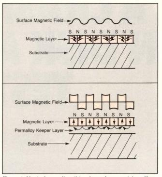
Figure 4: Vertical recording (b) reduces demagnetizing effects caused by adjacent poles of like charge, and produces a sharper surface magnetic field than conventional horizontal recording (a). (Courtesy Vertimag).
