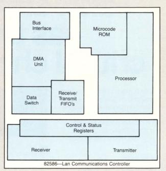
Figure 2: 82586—VLSI Local Area Network Communications Controller from Intel.
