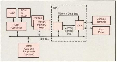
Figure 2: Schematic drawing of the Micro-VAX1 which illustrates its two-board Qbus configuration. (Figure courtesy Digital Equipment Corp.)
