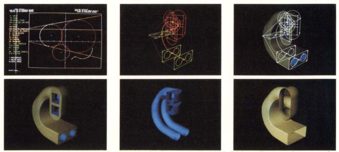
Figure 3: Creation of a manifold design on SDRC's IDEAS supported by Lexidata's Solidview. The system demonstrates the problem of parametric input in terms of time required, and the technique's flexibility in the creation of complex designs. Another advantage of SM in general is shown by the ability to define internal views once geometry is input.
