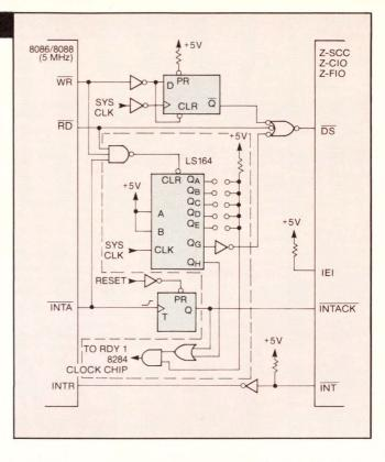
suppliers. Zilog's Z-Bus peripherals are designed with the flexibility to interface to most multiplexed address/data bus structures.
