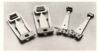
Figure 5: The heads shown from Applied Magnetics are, from left: Standard, full-size monolithic ferrite slider on the Winchester suspension; full-size composite slider on Winchester suspension; mini-monolithic ferrite slider on Whitney suspension; and a mini-composite slider on the Whitney suspension.
