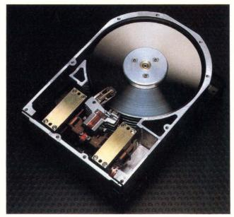
Figure 10: Priam's 500 series features a linear voice coil actuator delivering an average access time of 32 msecs.
