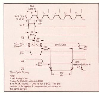
Figure 3: Read and Write cycle timing.
