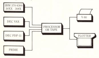
377X/SNA, 3780, HASP or bisync protocols under IBM OS, VS, VM/CMS, DEC VAX/VMS, RSX-11M/M-Plus & RT-11, PRIME PRIMOS, and other popular operating systems. exclusive compression algorithms. Some completely eliminate host computer overhead for plot processing.
