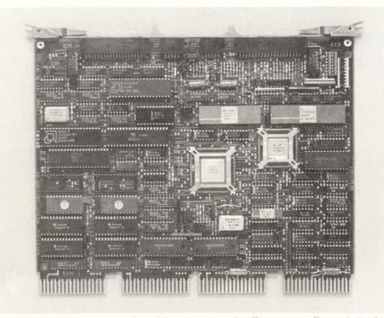
The KXT11-C I/O processor board functions as an intelligent controller optimized to handle communication processing.
