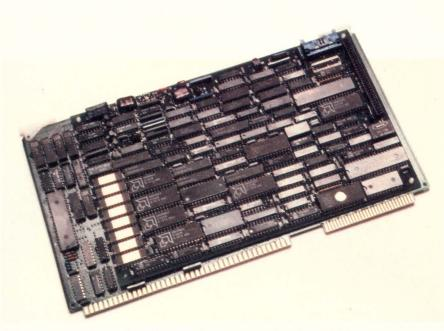
Ethernet Controller for Multibus based processors-Interlan NI 3010.
