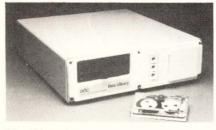
The disk back-up system from ADIC has interface adapters for most systems and buses including SASI, QIC-02, S-100, Multibus and GPIB. The system utilizes a 16 track  $\frac{1}{4''}$  data cartridge. Each track has 4096 addressagble blocks with 1024 bytes of data. The sytem features a 600 ft cartridge, error correction routine, and on board microprocessor control. Adic, Kirland, WA Write 163
