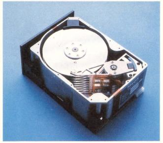
Figure 11: With a rotary voice coil positioning system, Maxtor's XT-4000 provides an average access time of 30 msecs.
