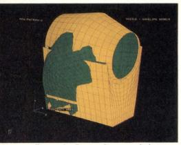
Figure 2: Patran-G, one of the most widely available finite element modelers, demonstrates the use of SM for interferences in this shot where the internal construction of the combustion chamber in green overlaps with its housing in yellow.
