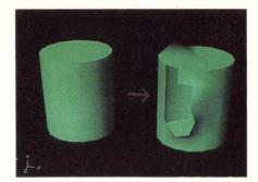
Above: Editing functions performed by SDRC's IDEAS modeling package 2D equivalent functions such as stretching and warping as well as functions unique to SM: blending, thickening, and bending. Other tasks unique to SM include surface operations such as tweaks for deformation.
