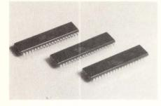
The HD6321 is a CMOS version of the NMOS parallel I/O peripheral interface adapter. Characteristics include two sets of 8-bit parallel data ports, four interrupt inputs, and handshake control. It is packaged in a 40-pin DIP and has a 10 mA current consumption during operation, and 500 A during standby. Hitachi, San Jose, CA Write 198
