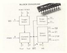
The MC3471P is a monolithic integrated Write Controller/Head Driver designed to interface the data and control signals and the heads for Tunnel or Straddle-erase floppy disk systems. Features include write current switching, track compensation, and on-chip erase delays. Price in quantities of 100-999 is \$4.25. Motorola, Phoenix, AZ Write 194
