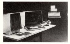
The Model 21/10 is a single station data procesing system that features 256 Kbytes of memory, SDLC communications, and an 80 cps printer. The system has 5 to 15 Mbytes of fixed disk storage and double-density diskettes with 1 Mbyte capacity. The 21/10 also supports 40, 45 and 120 cps printers. Price is \$6,000. to \$20,000. Mowhawk Data Sciences, Parisippany, NJ Write 138
