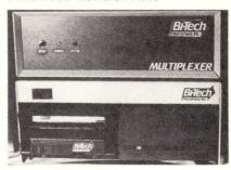
When combined with a hard disk subsystem, this multiplexer enables users to share a hard disk with four computers without the need for additional hard disk drives. The Multiplexer is a parallel transfer device with transfer speeds of 5 Mbit/sec and is compatible with most  $5\frac{1}{2}$ " fixed and removable hard drives. **B.T. Enterprises**, Bohemia, NY
