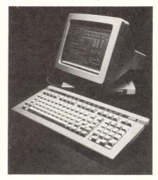
The WY-50 and WY-75 are smart editing alpha-numeric terminals which feature 14" screens with selectable 80 or 132 column widths. The terminals include nonvolatile memory which enables terminal parameters such as cursor type, transmission speed and operating mode, to be entered from the detached keyboard. Prices are \$695. (WY-50) and \$795. (WY-75). **Wyse Technology**, San Jose, CA **Write 134**
