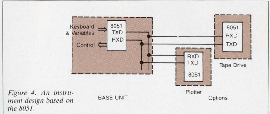
Figure 4: An instrument design based on the 8051.
