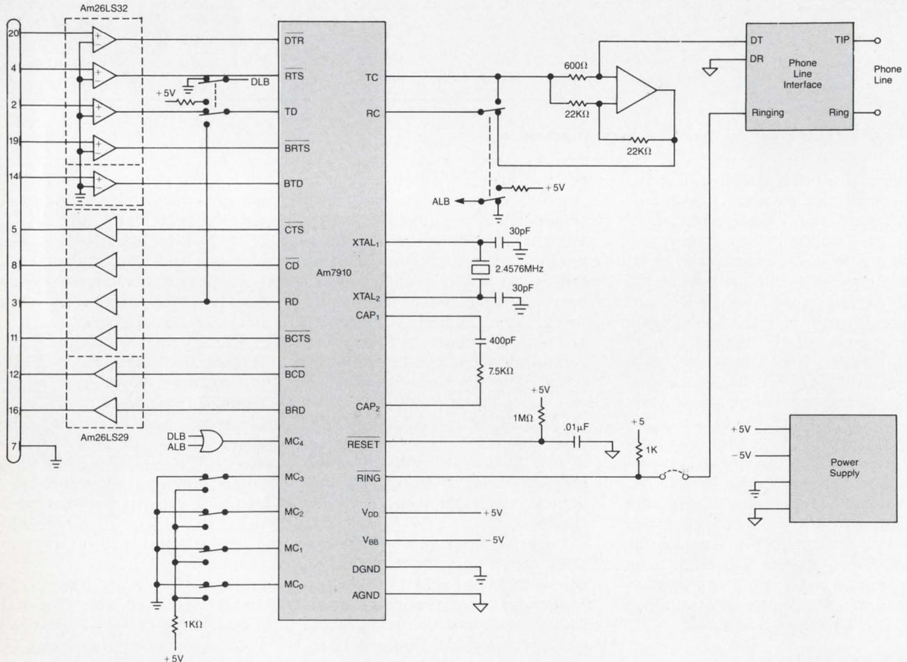
Figure 5: Am7910 FSK Modem.
