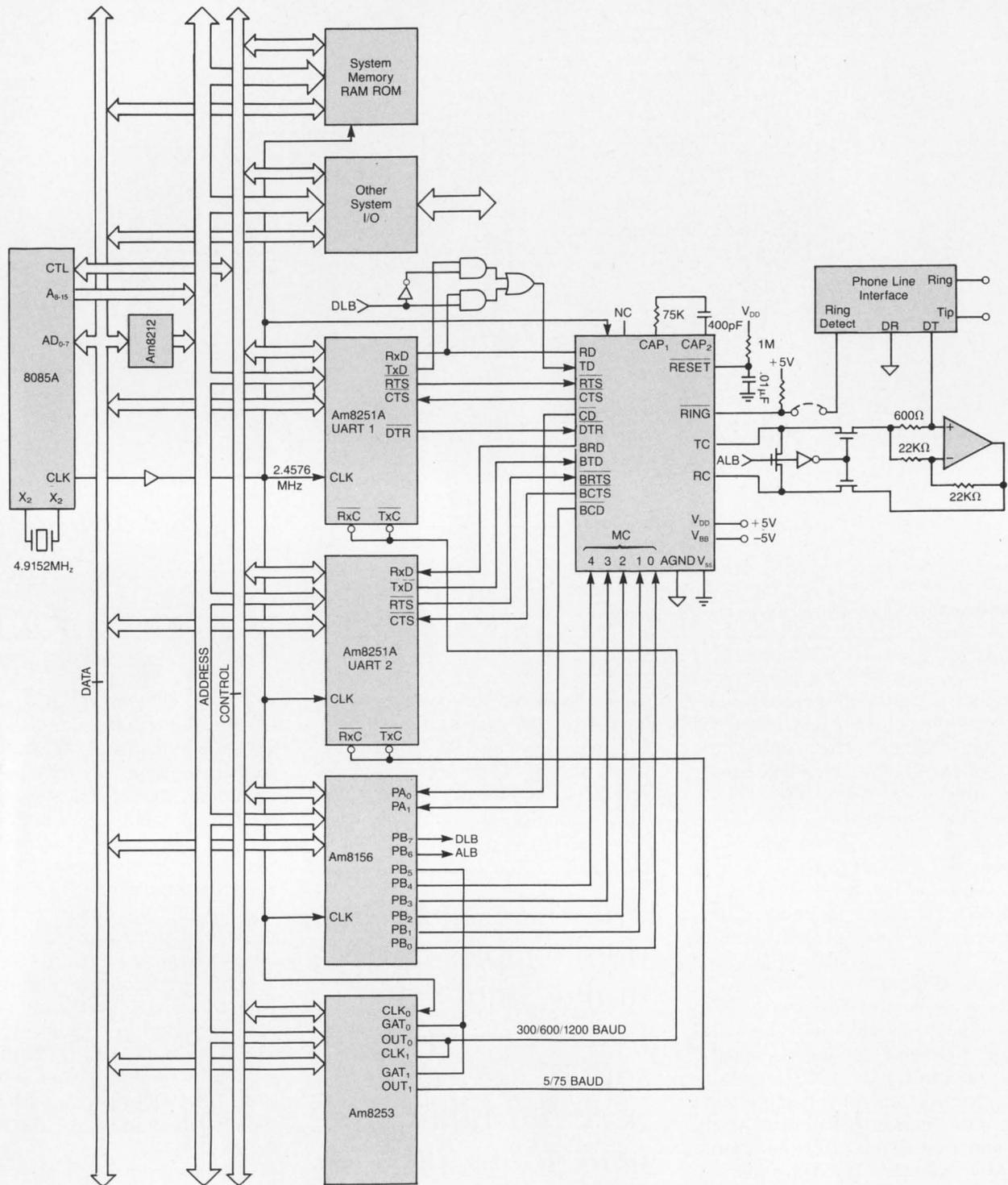
Figure 7: Am7910 in an expanded 8085 system.
