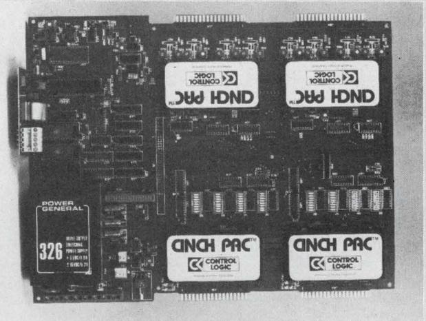
*Figure 1: Inconix Corp.'s Cinch Pac is an intelligent measurement and control system based around the MCS-51 family.*
