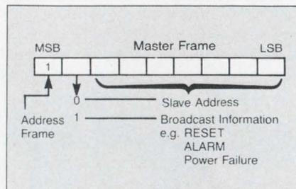
Figure 3: Network efficiency can be increased by defining software-recognized control bits in the address frame.
