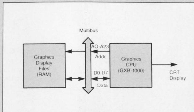
Figure 1: Display file/Graphics CPU architecture.
