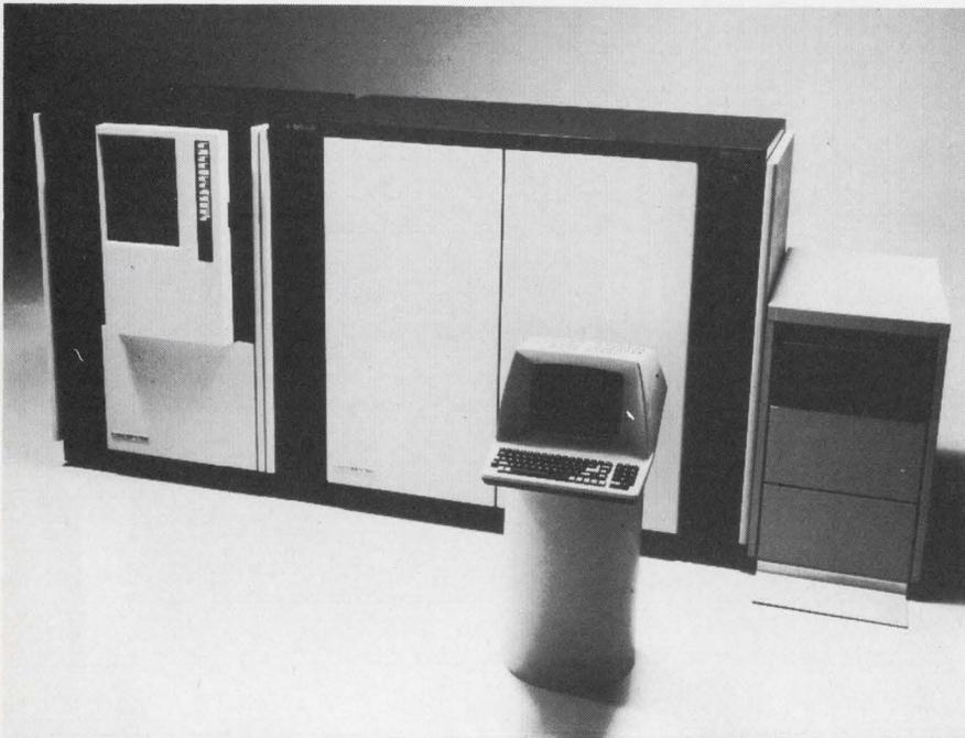
of a multiprocessor made up of 3 processors which allows placement and management of intelligence as close to the actual process as possible. An optional fourth processor, a data control unit, acts as a communications controller, handling up to 8 synchronous lines. Up to four of these data control units can be configured around a single MV/8000.
