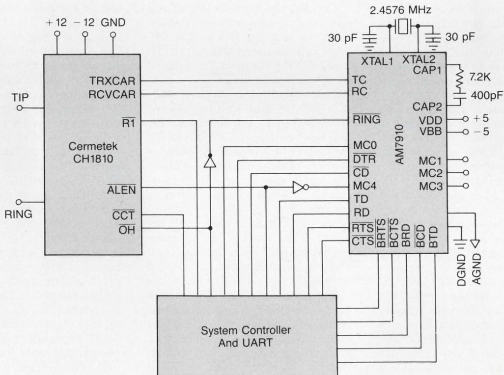
Figure 1b: AM7910 interfaced with Cermetek CH1810.
