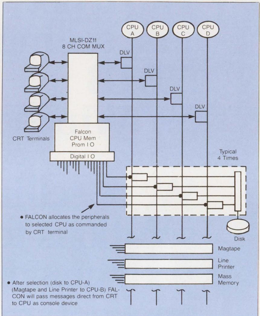
Figure 2: Transparent switch control through CRT terminals.
