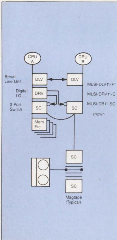
Figure 1: Program control from one CPU.
