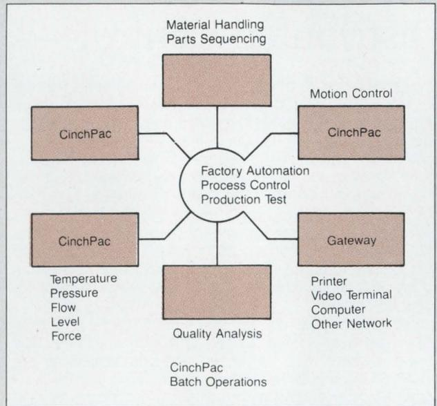
Figure 2: CinchPac with individual assignments interconnected with Cinchnet industrial network.
