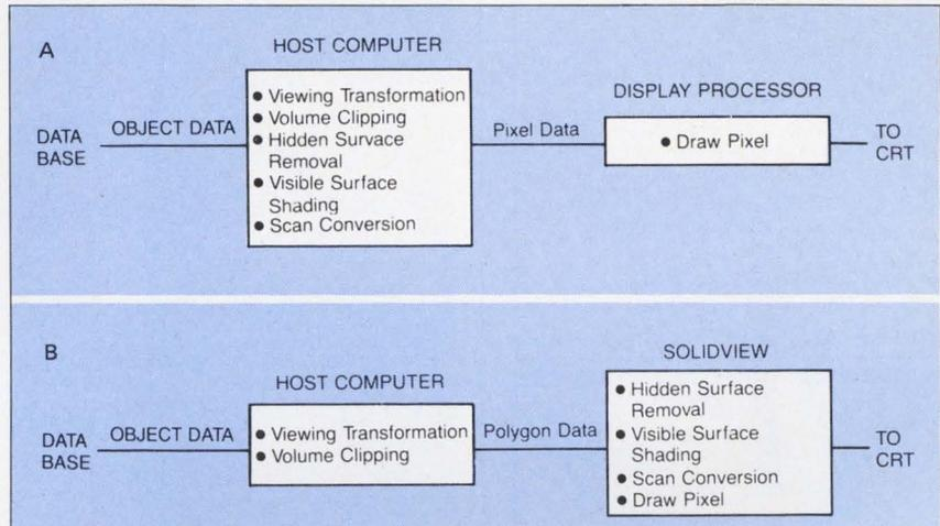
Figure 1: A) Typical solid modeling systems are host intensive, as opposed to B) SOLIDVIEW, which off-loads the host and balances the workload.
