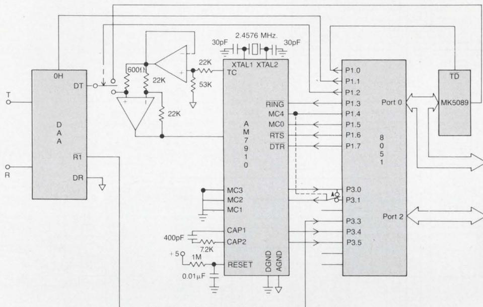
Figure 6: 8051 Single chip  $\mu$ P interfaced to Am7910
