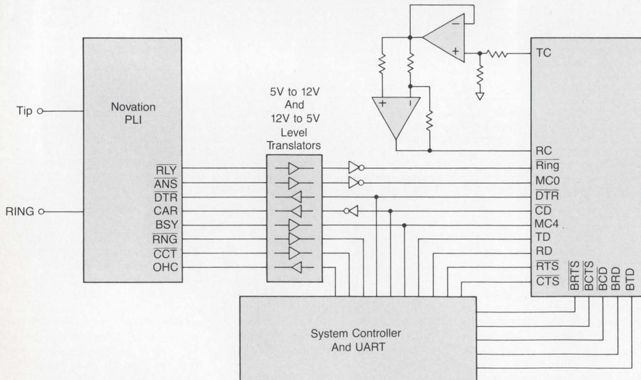
Figure 1a: Am7910 interfaced with Novation PLI
