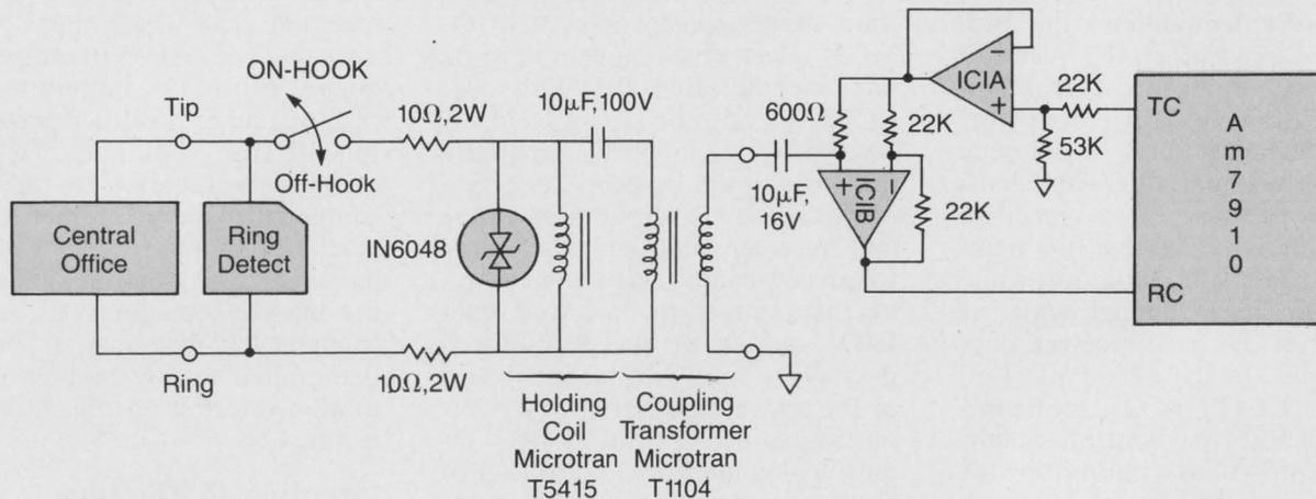
Figure 2: Am7910 Data access arrangement.
