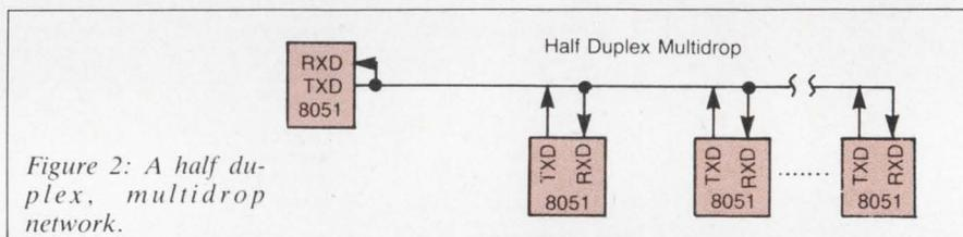
Figure 2: A half duplex, multidrop network.
