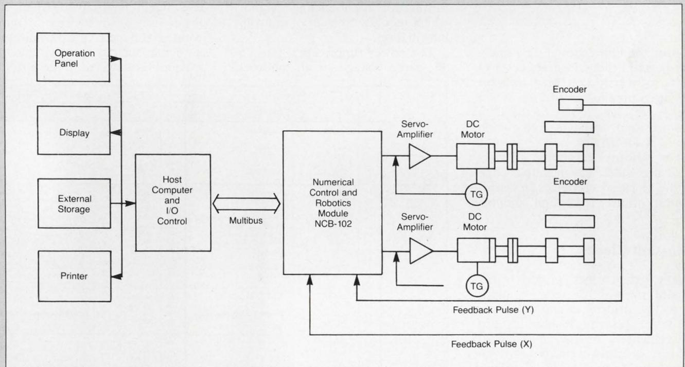
Figure 1: The NCB 102 numerical control and robotics module shown in a typical application.
