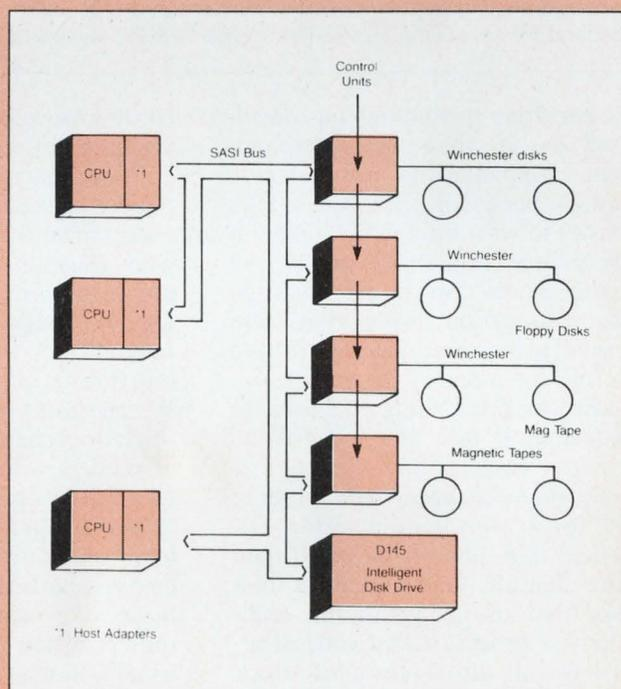
Figure 1: The SASI bus supports up to eight SASI devices, which can be any combination of host CPUs and intelligent controllers.
