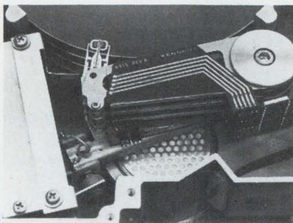
Figure 1: Kennedy's positioning system is a voice coil rotary actuator with the voice coil placed near the read/write heads (instead of behind the arm pivot).
