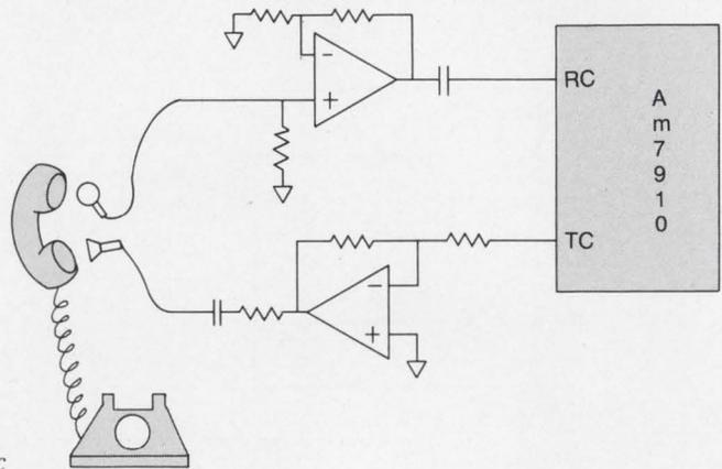
Figure 4: Acoustic Coupling Circuit.
