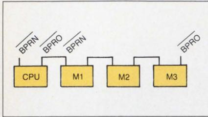
Figure 1: Priority in and out lines are used for determining priority resolution and are connected in this daisy-chained fashion. M1, master 1, is the highest priority module; M3, the lowest. Both signals are tristate with a 5 mA minimum driver current and -2 and -1.6 mA maximum receiver current, respectively (in L to R sequence above)
