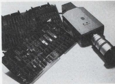
Figure 2: The IP-512 image processor and graphic controller features the unique combination of modular frame buffer (FB-512), analog processor (AP-512) and pipeline processor (ALU-512), for flexible digital image processing. Combined with a Multibus or Q-bus based computer, the IP-512 becomes a complete Image Processing system.
