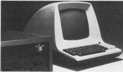
drives providing 400 Kbytes of storage capacity. Model 520T has two double-sided, double-density drives for 800 Kbytes of storage. The 1.6 Mbyte system is the Model 540T package. The conversational terminal has an 80-character  $\times$  24-line display
