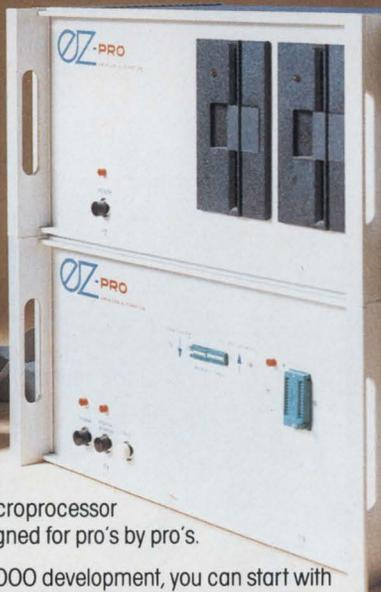
**Start Easy.** The system is modular. For a 68000 development, you can start with our Basic Development Unit (32 KB of 100 ns SRAM), the In-Circuit Emulator (totally transparent, 10 MHz, no wait states), and our 320 KB Dual Disk Unit, with your own keyboard and printer. All for a palatable \$10,195.
