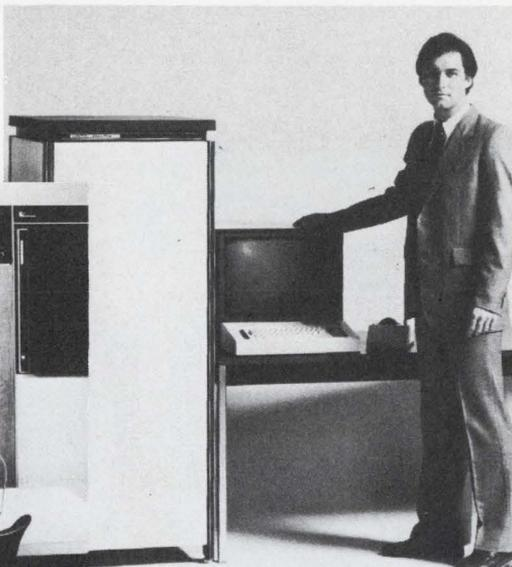
The keyboard is an 87-key detachable unit with 24 programmable function keys and auto repeat. Functions include insert and delete character and line, erase line and page, cursor addressing, 4 split screens horizontal and vertical, and self-test and diagnostics. Communications specs are: RS-232C, full or half duplex, 110 to 19,200 baud, and auxiliary port. From \$2200 to \$2750 depending on quantity.
