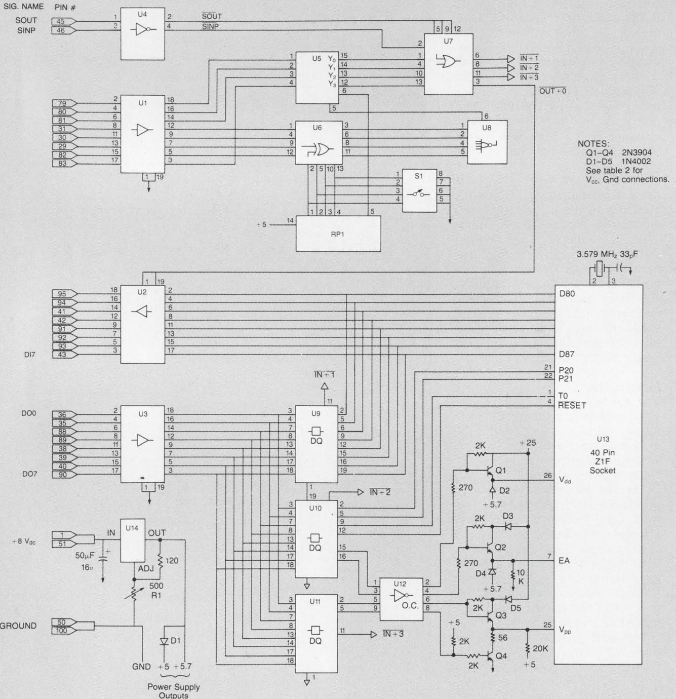
Figure 1: A schematic of the S-100 8748 programmer circuitry.
