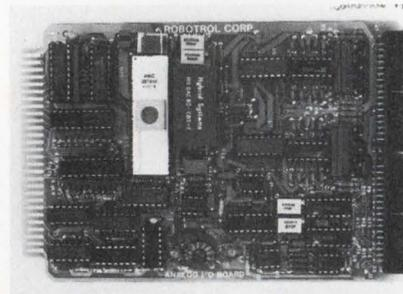
requires only 4 consecutive addresses; and vectored interrupt or polled program operation. The RSD-7728 operates with a Z80 or 8085 CPU up to 4 MHz and with a 6800 or 6809 CPU up to 2 MHz. \$360 (qty. 100). **Robotrol Corp**, 1250 Oakmead Pkwy, Suite 210, Sunnyvale, CA 94086. **Write 143**
