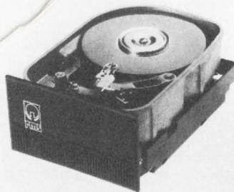
An optional Data Express-II data separator increases capacities by another 50% (9.5, 19.13, 28.5 and 38 Mbytes) and uses a faster 7.5 MHz transfer rate. Another optional data separator, Data Express I, provides system integrators with standard MFM coding and 5 MHz data rates. From \$935 to \$1485 in 100 qty; Data Express I is \$197; Data Express II is \$250. **Rotating Memory Systems Inc.**, 1701 McCarthy Blvd, Milpitas, CA 95035. **Write 133**
