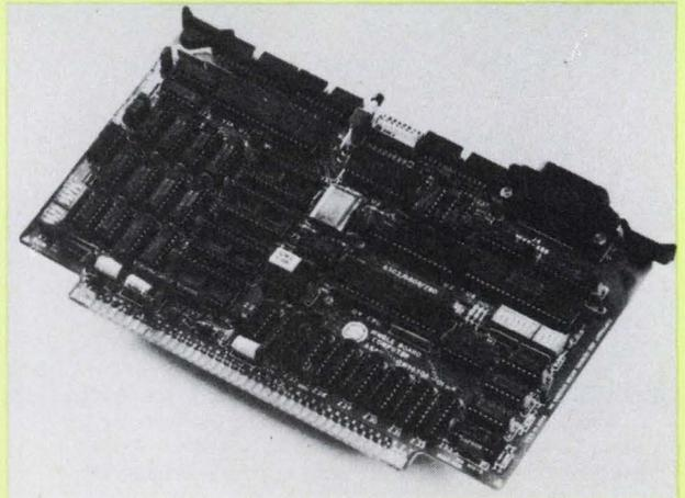
Operating systems for the 6502 (basically the System 65 operating system), 6809, and Z80 families are available. Individual software packages for IEEE-488, ACIA and printer are also available. All of the General Micro modules are burned-in for 72 hours. Each carries a full year's warranty. The 6" by 9.75" boards sell for about \$500 each with quantity discounts available.
