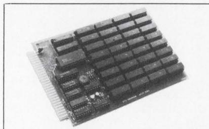
Figure 1: The NOVRAM-1 board from Acquis Data, provides 4 Kbytes of nonvolatile RAM using Xicors NOVRAM devices.
