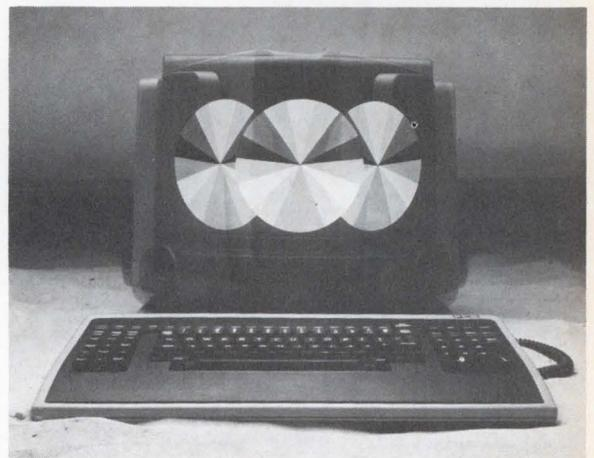
(Chicago, IL) will be introducing a desk top graphic computer family of its own (Figure 4). The 68000-based system combines high-level performance with high-resolution bit-mapped graphics and features a building block system approach based on advanced industry standards. The system uses a UNIX operating system, C and Fortran software tools, the IEEE P-796 Multibus standard and Ethernet networking capability. As a result, Cadline claims to support both tra-
