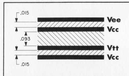
Figure 1: For systems requiring high speed ECL logic, four-layer multilayer wire wrap panels and connector backplanes are available.
