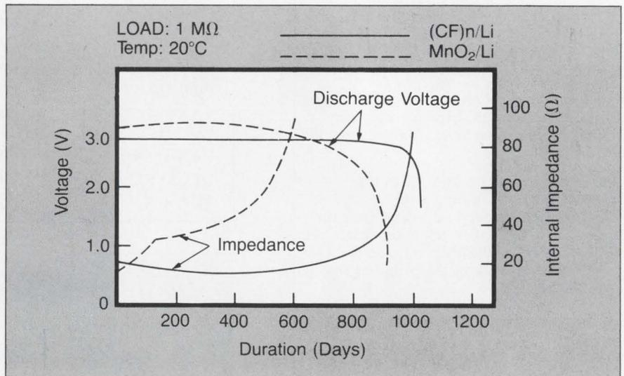
Figure 2: Graph compares characteristics of a  $Li(CF)_n$  cell with those of another solid-cathode cell using  $MnO_2$ . One reason for a flat characteristic of the monofluoride cell is that its internal resistance remains constant.
