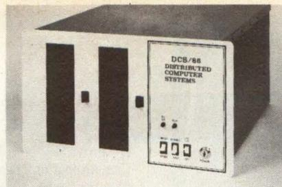
ports, 2 of which are capable of high level bit protocols such as HDLC and SDLC. One of the protocol ports is RS-232 and the other is RS 422/423 for network communications. The CPU also contains 24bits of parallel I/O
