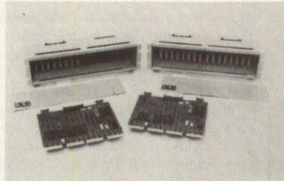
Unibus DZ11-A/DZ11-B (EIA) 8-line multiplexors and the DZ11-E (EIA) 16-line unit. Another model combines the characteristics of the DZ11-A and the DZ11-C (EIA and 20 mA current loop). They offer programmable character formats and data rates from 50 to 19.2K baud. The MLSI multiplexor modules contain a 64 character buffer with a 16-bit SILO counter which allows minimal processor intervention. From \$1350 to \$2800. **MDB Systems Inc.**, 1995 N. Batavia St., Orange, CA 92665.
