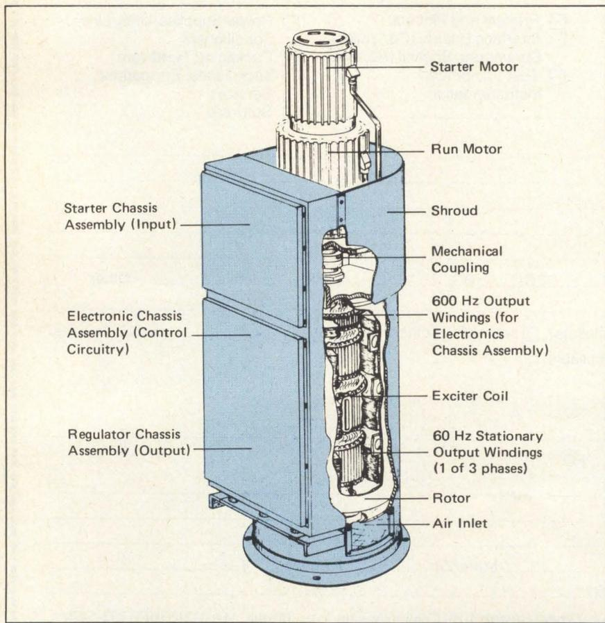
Figure 1: This variable-speed, constant-frequency (VSCF) generator uses an exciter coil that prints magnetic poles on a magnetic rotor fly wheel, producing even-frequency power, despite input power spikes, dips, and outages of 10 secs or more.
