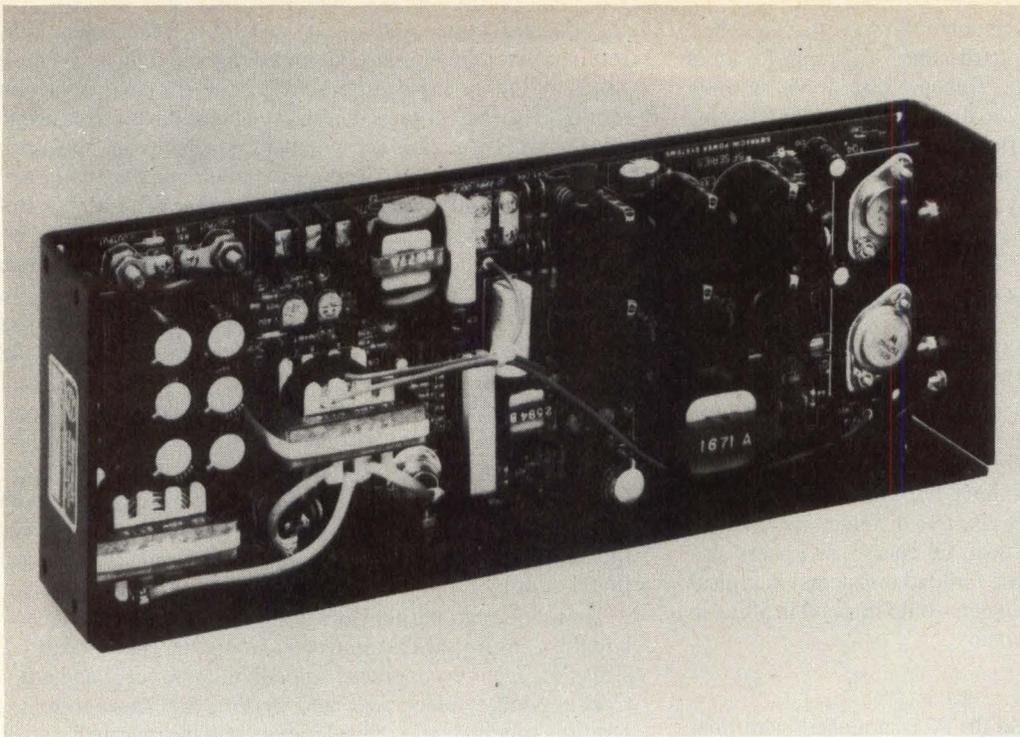
**Figure 2: Single and multiple output switchers are available in different models, each with its own voltage and current ratings. To reduce cross-regulation, as with Sierracin/Power Systems' switchers, auxiliary outputs are preregulated by the switching section, then postregulated by linear regulators.**
