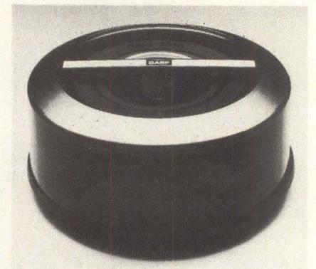
drives. It has 10 recording disks, 19 recording surfaces, plus top and bottom protective disks. A servo surface is prerecorded to provide precise control data for seeking, position sensing, and clocking. Track density is 384 tpi; bit density is 6,038 bpi. \$1,100. **BASF Systems Corp.**, Crosby Drive, Bedford, MA 01730.
