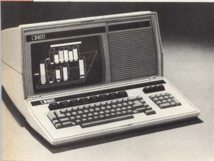
amber. Fully compatible with DEC VT 100. RS 232 or 20 mA interface. Keyboard baud rate 50 to 19,200.
