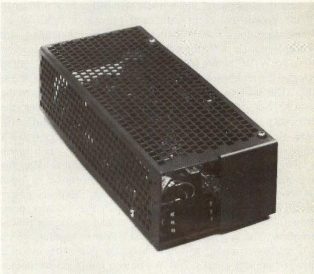
**Figure 1:** With 115 Vac or 230 Vac input at 47 to 440 Hz, Standard Logic's SWS 150 Series is designed for either domestic or European applications. It has good regulation on all outputs. Features include single phase input, 75% efficiency, low parts count, remote sense and remote shutdown capability.
