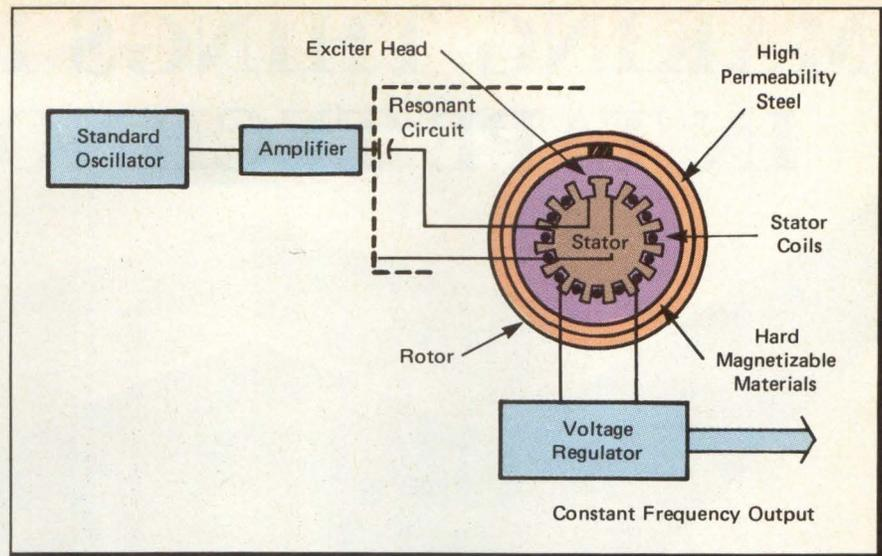
**Figure 2:** A standard oscillator regulates PoweRotor's exciter head, so that it prints poles on the spinning magnetic rotor drum at a constant rate. The 800-lb rotor, which may run on any power source, can speed up or slow down, but the stator coils will still see the same number of poles per second, keeping frequency accurate to 0.025%.
