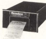
World's smallest complete 20 column alphanumeric panel mount printer. Has RS232C and 20 mA loop interface, is microprocessor controlled, has internal self test program and includes all drive circuits and AC power supply.
