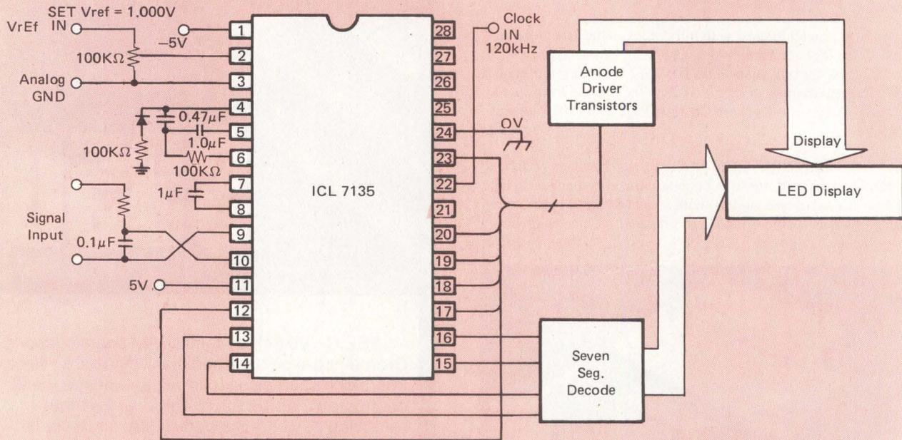
ICL 7135 one chip  $\pm 4\frac{1}{2}$  digit CMOS A/D converter drives LED display.
