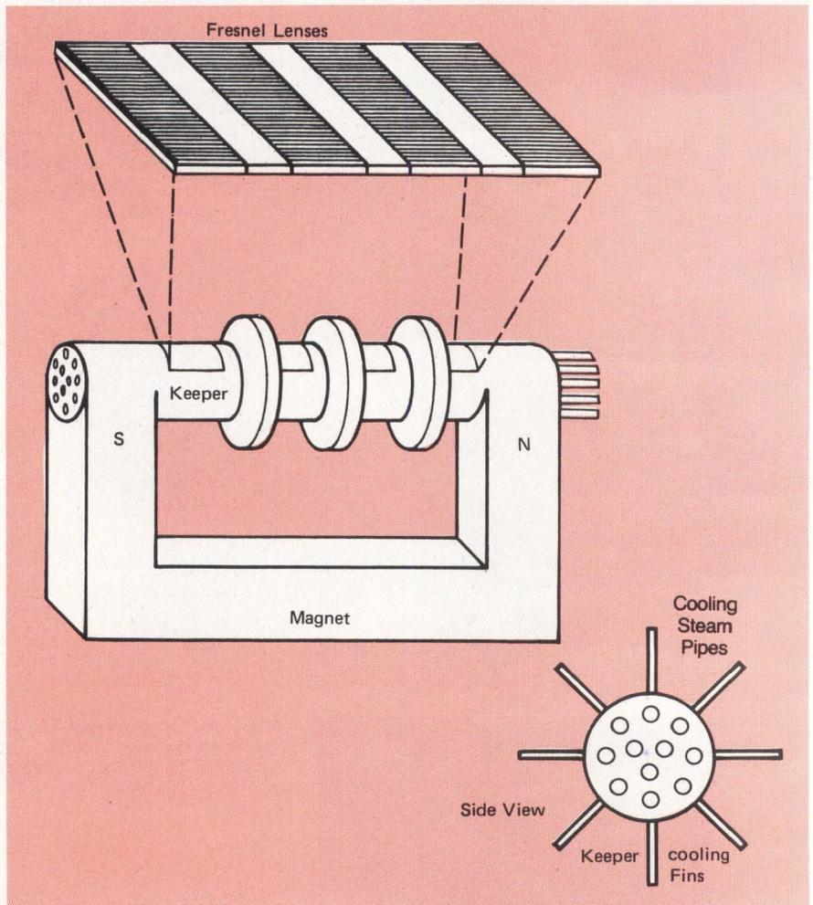
**Faraday Solar Generator focuses rays to heat soft iron keeper, causing magnetic domain disalignment and rapid outward flux line movement, which cuts coils. Next, steam burst through keeper pipes lowers keeper temperature, causing domain realignment and flux collapse, inducing a negative counter emf pulse. A mechanical or electrosensitive shutter for the Fresnel lenses is not mandatory.**
