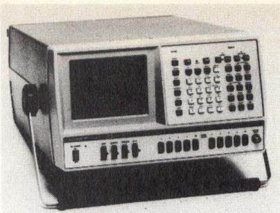
system with an interactive keyboard and display. It is compatible with the IEE-488 GPIB so it can be used in fully automated
