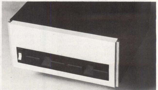
stepping rate 10 times faster than previous mini-floppy systems, is both small and low cost, and provides 1.8 MB of disk storage. **General Robotics Corp.** 57 N. Main Street, Hartford, WI 53027. **Circle 181**
