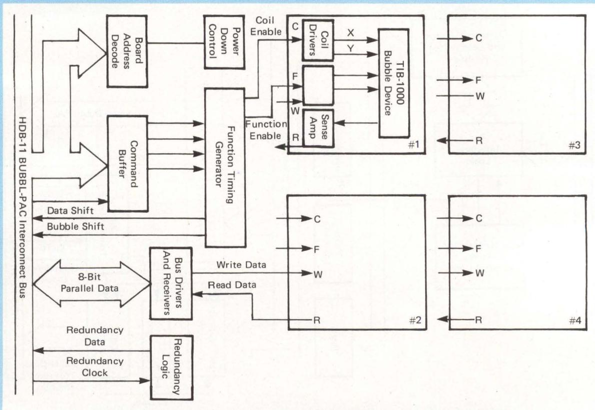
Figure BB: HDB-11 Bubbl-Pac Block Diagram
