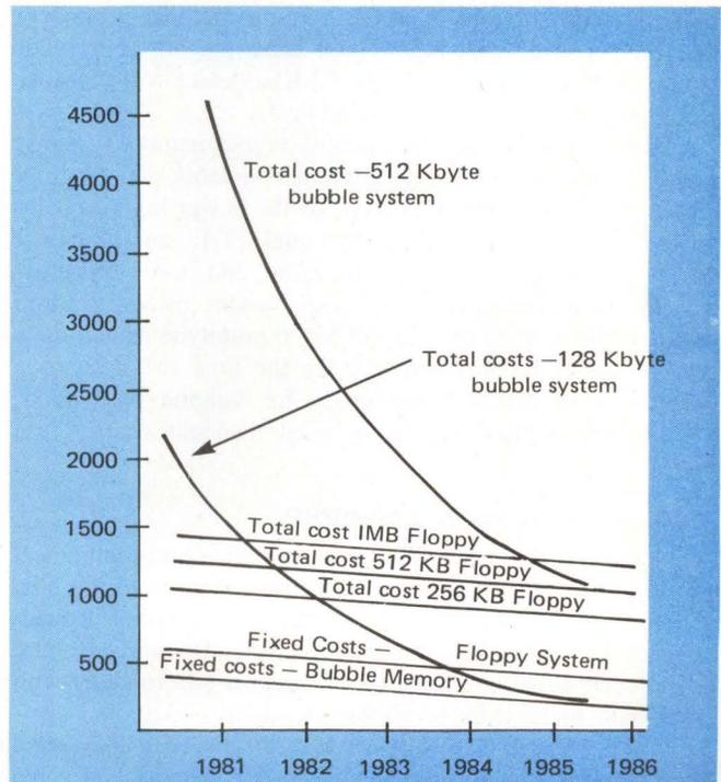
Figure 2: Price comparison for bubble memory system vs floppy disk considering total storage capacity
