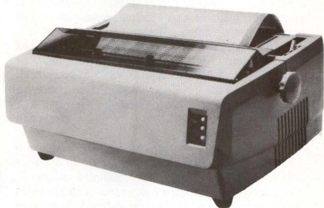
produce letter-quality printing on 3 copies with either 136 or 163 columns. Compatible with sheet feeders, handles forms up to 15" wide, includes self-test, programmable VFU and front panel indicator lamps for paper, select and power status. **C. Itoh Electronics Inc**, 5301 Beethoven St, Los Angeles, CA 90066. **Circle 241**
