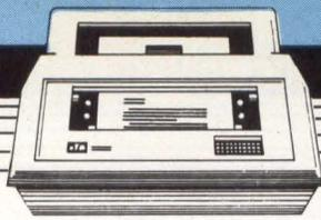
**Impact Line Belt Printer.** The Quiet 300 features a 300 lpm print speed and switchable serial/parallel interface. It includes up to 9600 baud rate, 64 or 96 character ASCII, tractor paper feed and 1K memory optional to 4K. Interfaces include RS-232C, 20 mA, Centronics parallel, DEC LA-180. **Local Data**, 2701 Toledo St, Torrance, CA 90503. **Circle 243**
