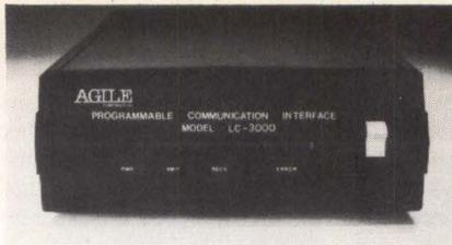
standalone  $\mu$ P-controlled protocol translator and line speed converter. It is plug compatible with the 20mA MTS 3000 HP current loop and offers HP modified bisync compatibility. LC-3000 also includes a 4000-byte receive buffer, a 256-byte trans-
