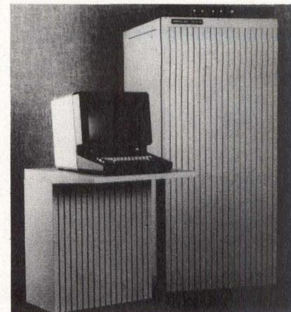
to 340ns. Reliability features include hardware error logger, ECC memory, power fail/automatic restart, processor self test, and the capability for remote diagnostics. Model 3230 is \$46,789 (qty 15) for a processor with 512 kB MOS memory, a Model 550 system console, real-time clock, cache memory, and battery back-up. **Perkin-Elmer**, Computer Systems Div, 2 Crescent Place, Oceanport, NJ 07757.
