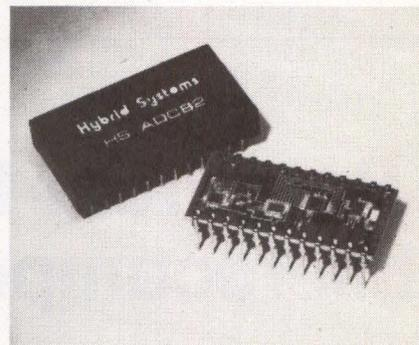
ature and improving stability; and, the power supply voltage range has been widened to include operation at  $\pm 12V$  supplies. HS ADC82 is an 8-bit ADC which converts in  $2.8\mu\text{Secs}$ . Packaged in a 24 pin DIP; \$69 (1 - 9), \$48 (100). **Hybrid Systems Corp**, 22 Linnell Circle, Billerica, MA 01821. **Circle 193**
