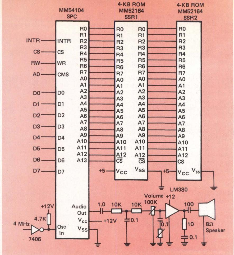
Figure 2: Microprocessor circuit for exercising the Speech Synthesizer.
