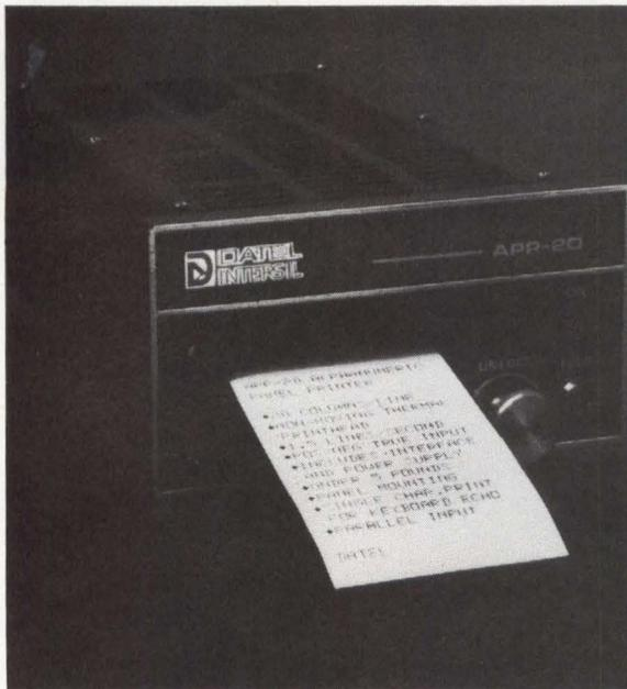
Features inverted or extra-height character printing, single character and keyboard echo printing. Accommodates 2.31" wide thermal paper at 20 col/line. The APP-20-2 is a serial input version which can accept RS-232C or 4-20 mA serial data inputs. It also includes a one line internal buffer. Both measure approx. 4"W x 3"H x 9"D. A 48 column version is also available. **Datel-Intersil**, 11 Cabot Blvd, Mansfield, MA 02048. **Circle 230**
