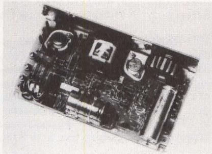
porates the Univerter design, a feed-forward, pulse width modulated inverter using only one switch transistor. It requires fewer parts, for a higher efficiency, longer MTBF and improved reliability. **Adtech Power**, 1621 South Sinclair, Anaheim, CA 92806. **Circle 129**
