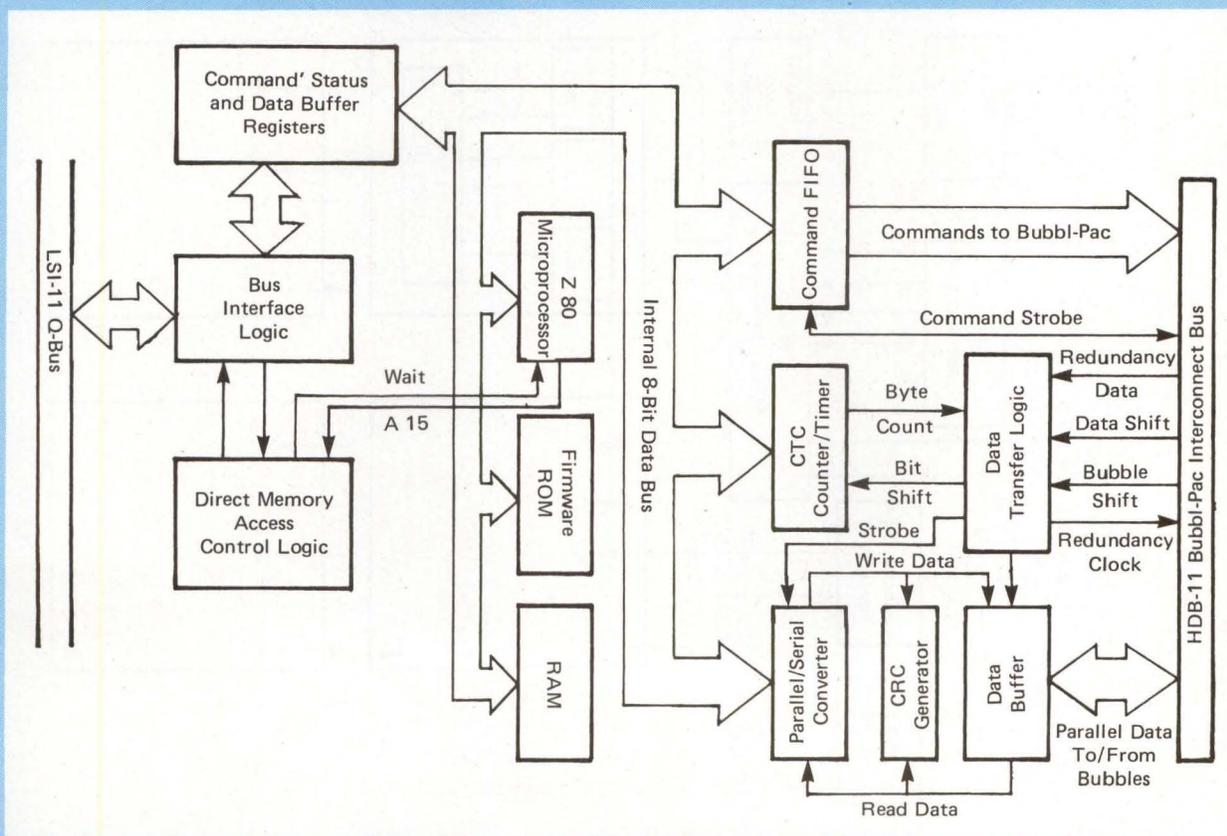
Figure B: Typical block-replicate device-schematic
