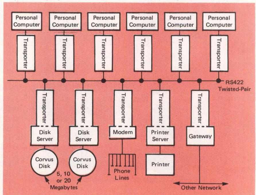
storage and printers and two to 64 computers; it is easily expandable as needs grow and simple to install (screwdrivers and pliers).
