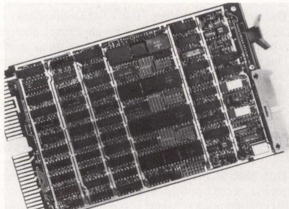
parallel daisywheel printers. The MSI 11 series connects the LSI-11/Q-Bus to 1, 2 or 4 serial lines and printers with serial interfaces. The MSI 11-P connects the LSI-11/Q-Bus to 2 or 3 serial lines and a parallel line printer. Compatible with DEC RT-11 and RSX-11 software. **Andromeda Systems, Inc.**, 9000 Eton Ave, Canoga Park, CA 91304. **Circle 259**
