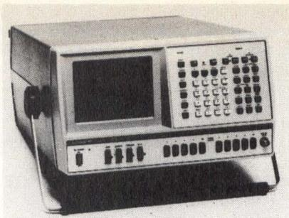
system with an interactive keyboard and display. It is compatible with the IEE-488 GPIB so it can be used in fully automated
