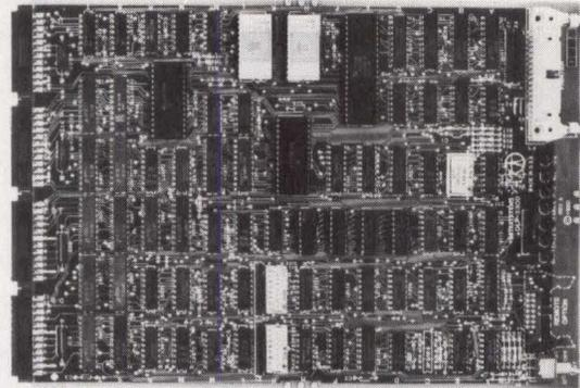
features: self-test which verifies controller, cable and printer operations and assists in printer system troubleshooting; all cables are interchangeable with other Datasystem controllers; all addressing and interface options are DIP switch selectable with no trace cutting or jumpering required; all are software transparent. **Datsystems Corp**, a Wespercorp Subsidiary, 8716 Production Ave, San Diego, CA 92121. **Circle 270**
