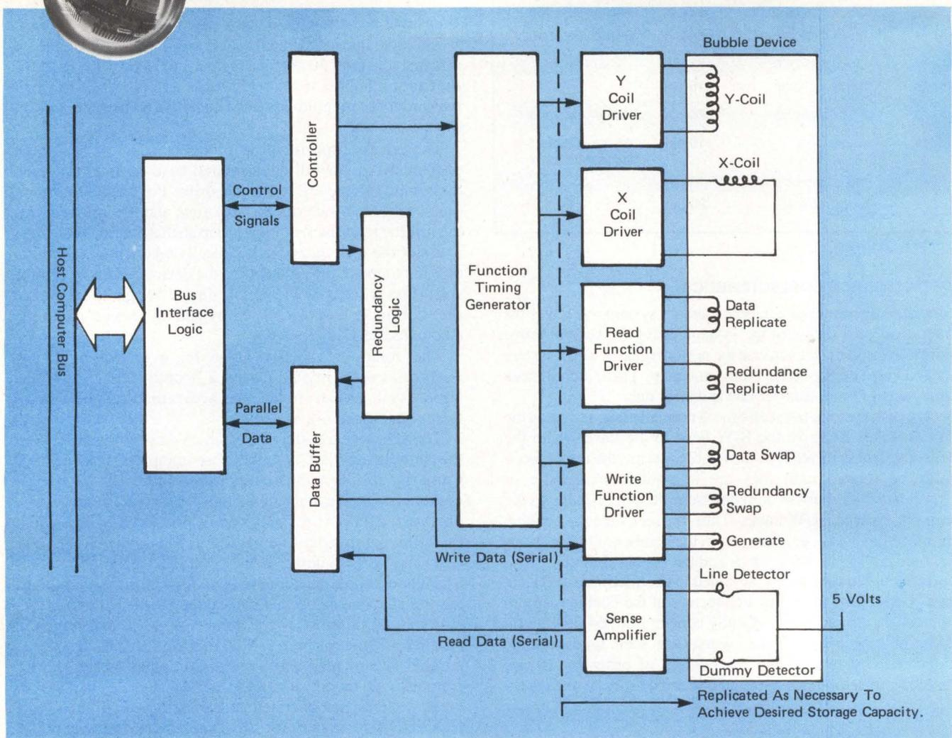
Figure 5: Typical block diagram for bubble-memory mass-storage system.
