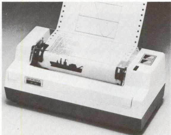
sets, 80 columns with 12 cpi, adjustable tractor feed, 3 copy reproduction, Centronics parallel interface. Optional interfaces include RS-232C, serial TTL, 20 mA current loop, IEEE 488, plus interfaces for most small computers. Print speed is 30 cps in a 5x7 dot matrix. Designed for the OEM and the personal and small business markets. **Axiom Corp**, 1014 Griswold Ave, San Fernando, CA 91340. **Circle 219**
