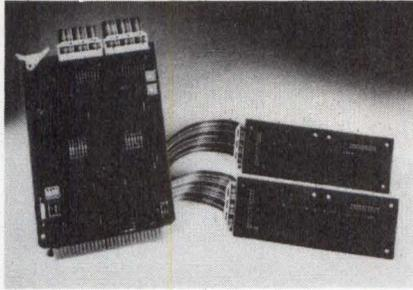
remote display up to 6' away. The 7911/HDC operates as write only memory and occupies 16 I/O mapped address locations. A decimal only version, the 7911/DDC, has special symbol displays and individual digit blanking. A LED support board, the 7911/HDA, consists of six .5" LED displays that are directly compatible with either the HDC or DDC. The Hex Display Controller is from \$190 to \$133 (100). **Matrix Corp.**, 1639 Green St., Raleigh, NC 27603. **Circle 148**
