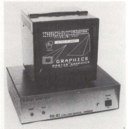
high level commands from a host computer and displays text and graphics on a standard 525 line TV monitor. Includes point to point draw, circles, reverse video, variable size ASCII characters, selective erase, and rectangular fill. \$1,450. **Raster Graphics**, Box 23334, Tigard, OR 97223. **Circle 184**
