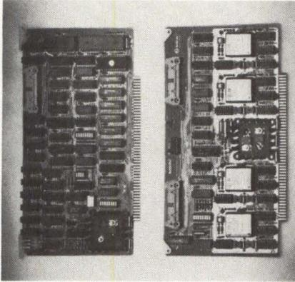
handles bubble-device formatting, error-checking and control. The MBB-100 contains 46 kB of bubble-memory mass storage. Access time is less than 4 ms average, 7.27 ms max. The MBC-100 controller is \$361; the MBB-100 is \$772 (100 ea. prices). **Bubbl-tec**, 6800 Sierra Court, Dublin, CA 94566. **Circle 242**
