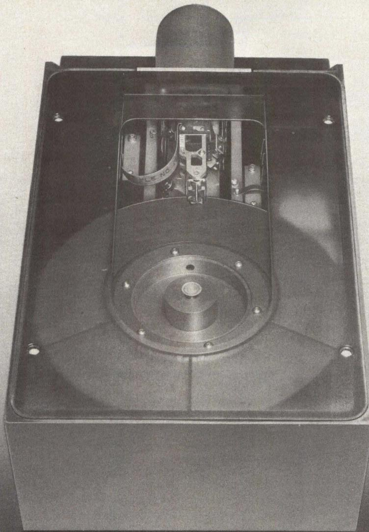
**Proven Reliability.** BASF, because of its experience in both magnetic media and drives, is highly qualified to develop drives using reliable 3350 Winchester technology. BASF 6170 drives have a 10,000 hour MTBF and require no scheduled maintenance or operator intervention.
