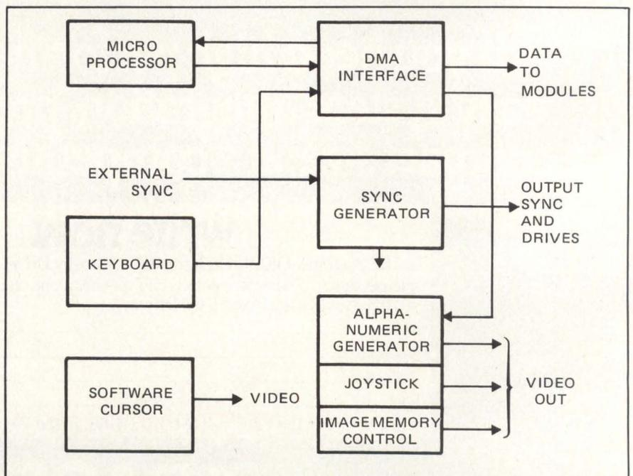
Figure 2: Core Subsystem contains the IDEX real-time bus switcher.
