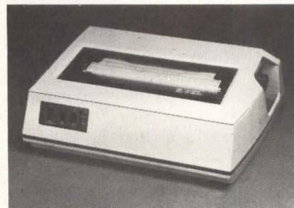
acters, 7 x 7 dot matrix with upper and lower case characters, serial RS232 communications interface, a monitor mode where all characters received by the printer, including control characters, are printed, and escape code sequences that allow for control of printer functions. Operation of the printer may be controlled locally or via the host processor. The P1600 is \$2395. **Beehive International**, 4910 Amelia Earhart Dr. Salt Lake City, UT 84125.
