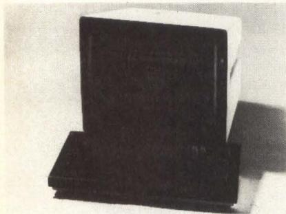
The slave printer interface is standard. The 95-key detached keyboard has separate numeric pad. It also includes a 20-key function keypad, with erase and print keys. The Model DG-Compat is \$1600; OEM and qty discounts available. **Ann Arbor Terminals, Inc.**, 6175 Jackson Road, Ann Arbor, MI 48103. **Circle 160**
