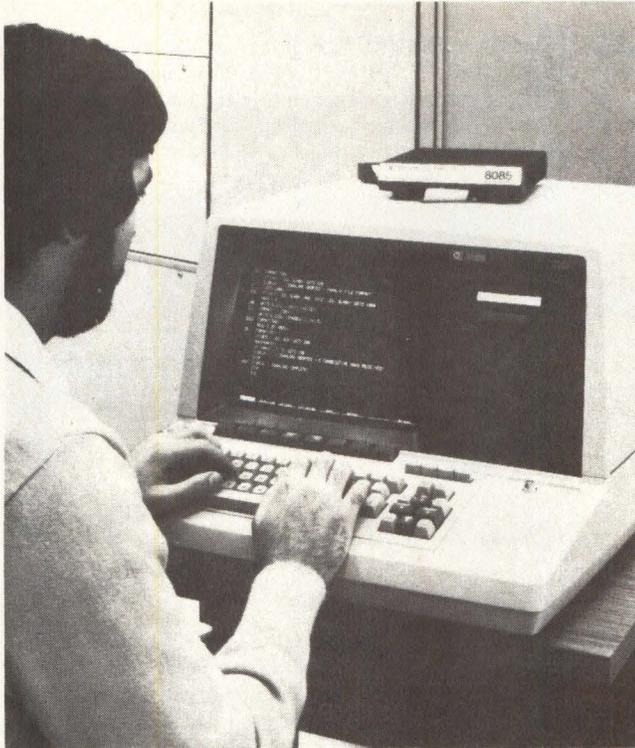
selected  $\mu$ P. Each contains a host processor with 64 kB of host memory, I/O control, and display control. The host and emulation systems have separate buses and memories. Model 64005S Emulation Terminal System is \$14,400 to \$22,600. **Hewlett-Packard Co.**, 1507 Page Mill Rd., Palo Alto, CA 94304. **Circle 216**
