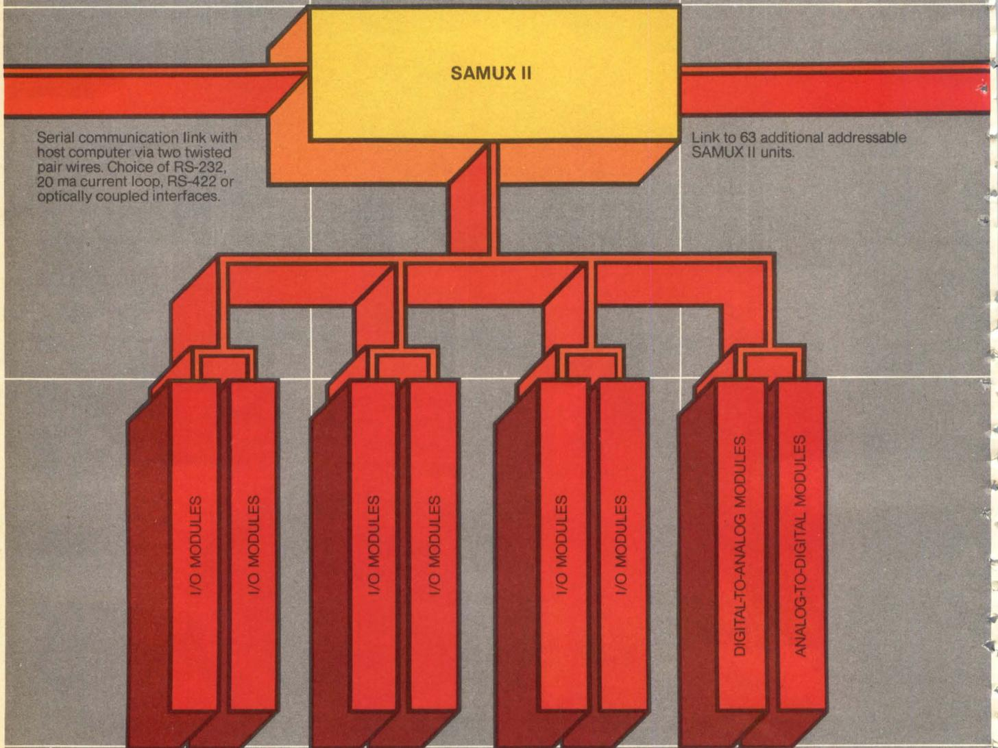
Serial communication link with host computer via two twisted pair wires. Choice of RS-232, 20 ma current loop, RS-422 or optically coupled interfaces.
