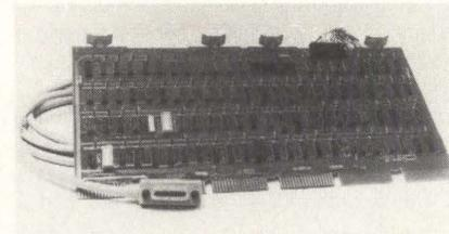
single or multiple Controller environment. The GPIB11-2/VX provides transfer rates of up to 500 kB/sec for tri-state operation and up to 250 kB/sec for open collector operation. A 4 meter cable with a GPIB connector on the outboard end allows connection of 14 instruments on a single interface. \$2495, including software and cable. **National Instruments**, 8900 Shoal Creek Blvd, Austin, TX 78758
