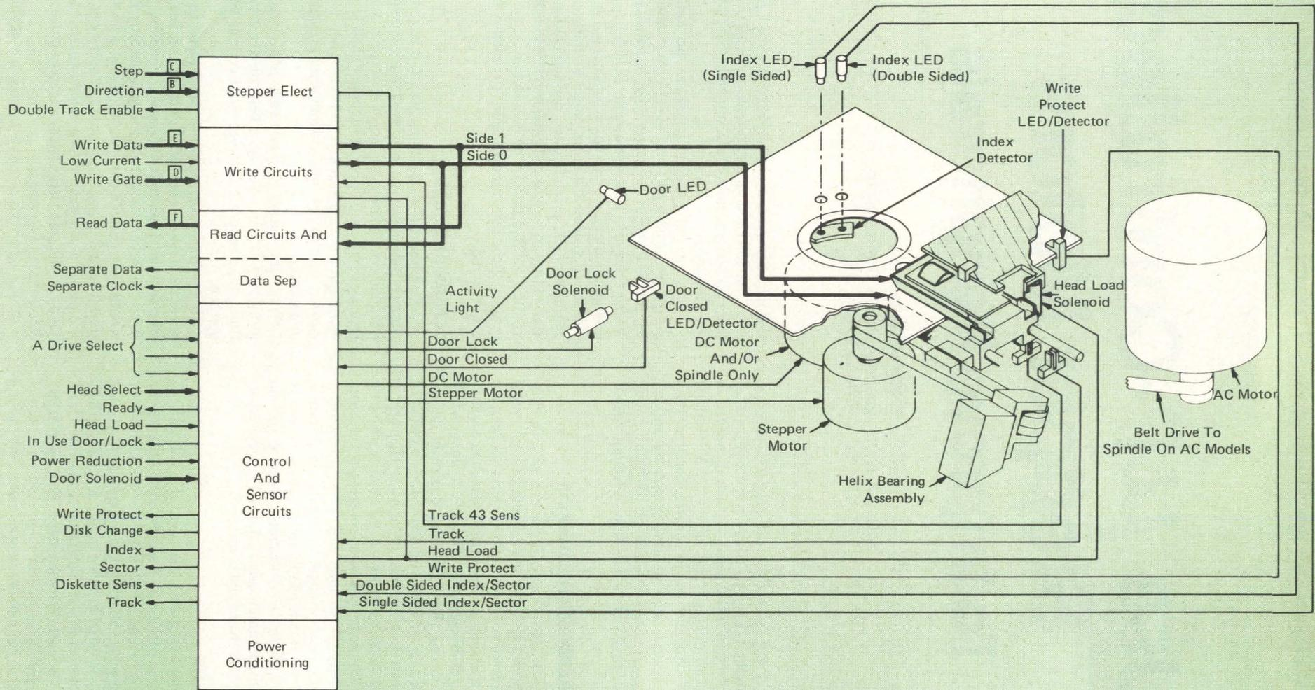
Flexible disk drives, such as MFE's 700 and 500 Series, provide single-sided operation (where maximum capacity is not required) and are just one peripheral that uses  $\mu$ P-controlled stepper motors.
