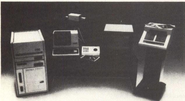
joystick controls, multiple cursor generation, additional image function memories and a hard copy color printer. All models in the GMR 260 Series are complete systems with a 16-bit parallel, TTL-compatible, bi-directional interface. Plug-compatible, DMA parallel interfaces are available. **Grinnell Systems**, 2159 Bering Dr., San Jose, CA 95131. **Circle 228**
