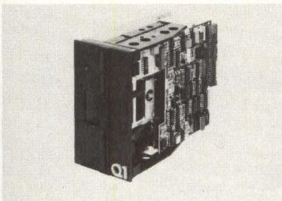
Microlite  $\mu$ C system. It is mounted within the console of the Microlite system, which is a desk-top, stand-alone, multi-function  $\mu$ C. A standard Winchester ferrite head is used, and data is recorded on the disks at 7500 bpi. The drive includes two motor assemblies (stepper and spindle), a head assembly with 4 Winchester heads, and a disk assembly consisting of two disks. **Q1 Corp.**, 125 Ricefield Lane, Hauppauge, NY 11787. **Circle 180**
