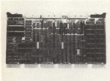
alternative that is ideal for VAX systems and works with equal effectiveness in other UNIBUS systems including PDP11, System 10 and System 20. The single hex-width board plugs into any standard hex SPC backplane slot and is diagnostic compatible with the DEC DH. Each 16-line multiplexer stands alone and runs independently. The user can install as many individual backplane-resident units as needed. **Able Computer**, 1751 Langley Ave, Irvine, CA. **Circle 127**
