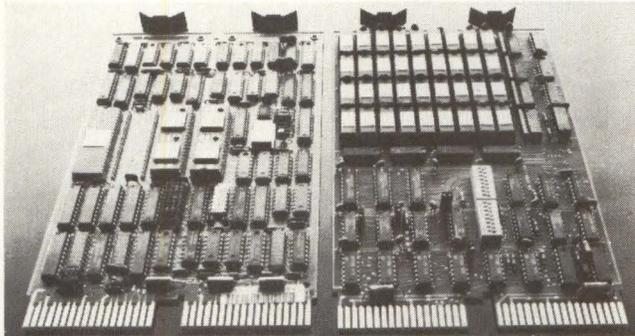
64K dynamic RAM with an access time of 240 ns and cycle time of 400 ns. Power requirement is 1.2A from a 5V supply with battery back-up operation available. The CI-1123 is \$1925 for a 128K x 9 option; \$2550 for the 256K x 9 option. **Chrislin Industries, Inc.**, 31312 Via Colinas #102, Westlake Village, CA 91361. **Circle 194**
