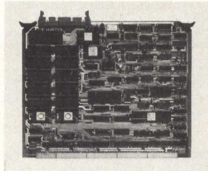
RAM. It may be used stand alone or as a master or slave in a multi-processor environment. Its two-channel serial I/O chip is capable of serial communications up to 500 kilobaud. I/O with other modules in the backplane is memory mapped. The 1868+A accepts both the 9511 arithmetic processor unit or the 9512 floating point processor unit. The module also provides direct memory access to the system's main memory. **Xycom, Inc**, 750 North Maple Rd, Saline, MI 48176. **Circle 202**
