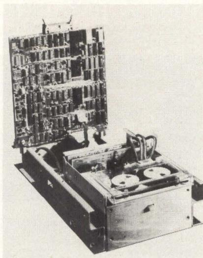
10 times before a new cartridge must be recorded. Model 6450 cartridge tape system incorporates a 6400-bpi, 30 ips cartridge drive and a  $\mu$ P-based formatter in a single compact package. With a 600' cartridge, the 6450 has an unformatted capacity of 23MB; 17.3MB with a 450' cartridge, 11.5MB with a 300' cartridge. Model 6450 is \$1520 ea./100. **Kennedy Co**, 1600 Shamrock Ave., Monrovia, CA 91016. **Circle 146**
