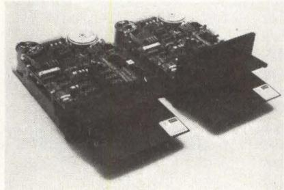
ical drive. With dimensions of 2.1" x 5.75" x 7.5", these units occupy 1/3 less space than other available drives. For full compatibility, they are also offered with an optional "industry-standard"-sized (3.75" high) front panel, allowing mechanical interchangeability in existing systems. Optional software-controllable door interlock and sensors and connectors, permit system customization and versatility. **BASF Systems Corp**, Crosby Dr, Bedford, MA 01730.
