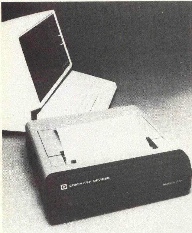
96 character upper and lower case ASCII code with underscore, remote terminal reset, and user controls for paperfeed, on-line/off-line, reset and self-test. The standard Model 1201 is \$1,385 (\$1,094/100). **Computer Devices, Inc.**, 25 North Ave., Burlington, MA 01803. **Circle 133**
