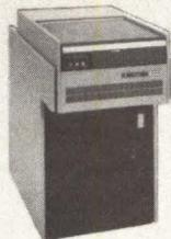
Plessey's PM-DS02D disc subsystem consists of the PM-DC1102 controller and one 67 Mbyte PM-DD11/80 SMD drive that has a proven history of reliability and data integrity. The PM-DS02D subsystem provides complete software and media compatibility with DEC's RH11/RM02 subsystem. The PM-DC1102, in this configuration, can directly support four 67 Mbyte disc drives for a total system capacity of 268 Mbytes. Disc pack files created on either the PM-DS02D or the DEC RM02 can be used interchangeably.
