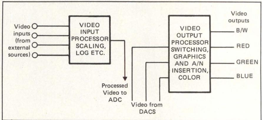
Figure 1: Analog Processor handles live incoming video.
