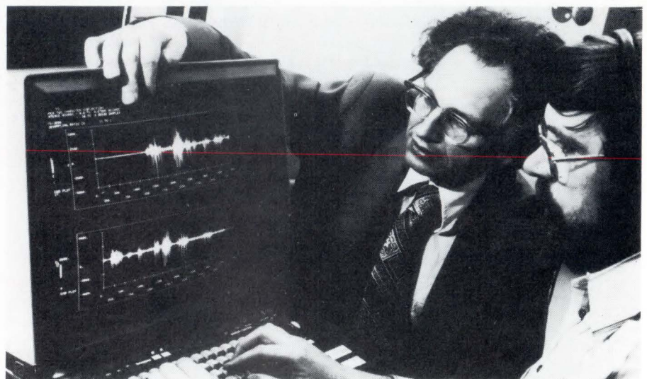
IBM Research scientists have used a computer to transcribe ordinary speech, composed of sentences drawn from a 1,000-word vocabulary and read at a normal speaking pace, into printed form with an accuracy of 91%.
