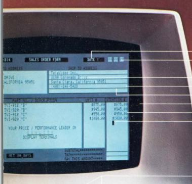
Reverse video Blinking/blank fields Upper/lower case char. Protected fields Underlining Non-glare screen 12 x 10 char. res. Blinking cursor
