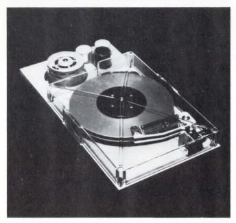
side-by-side in a standard 18" rack. Track-to-track time is 12 msec. Average head movement time is 50 msec, with a 100-msec worst-case maximum. A 3600-rpm disk rotation gives an average latency time of 83 msec. Delivery is three months ARO. Kennedy Co., 1600 S. Shamrock Ave., Monrovia, CA 91001. Circle 255
