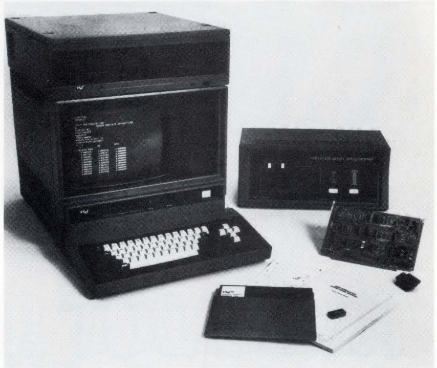
The designer can quickly transfer 2920 programs to the 2920 device via the Intellec \mu C development system and its Universal PROM Programmer by using the SP20 EPROM programming personality board and adapter socket.
