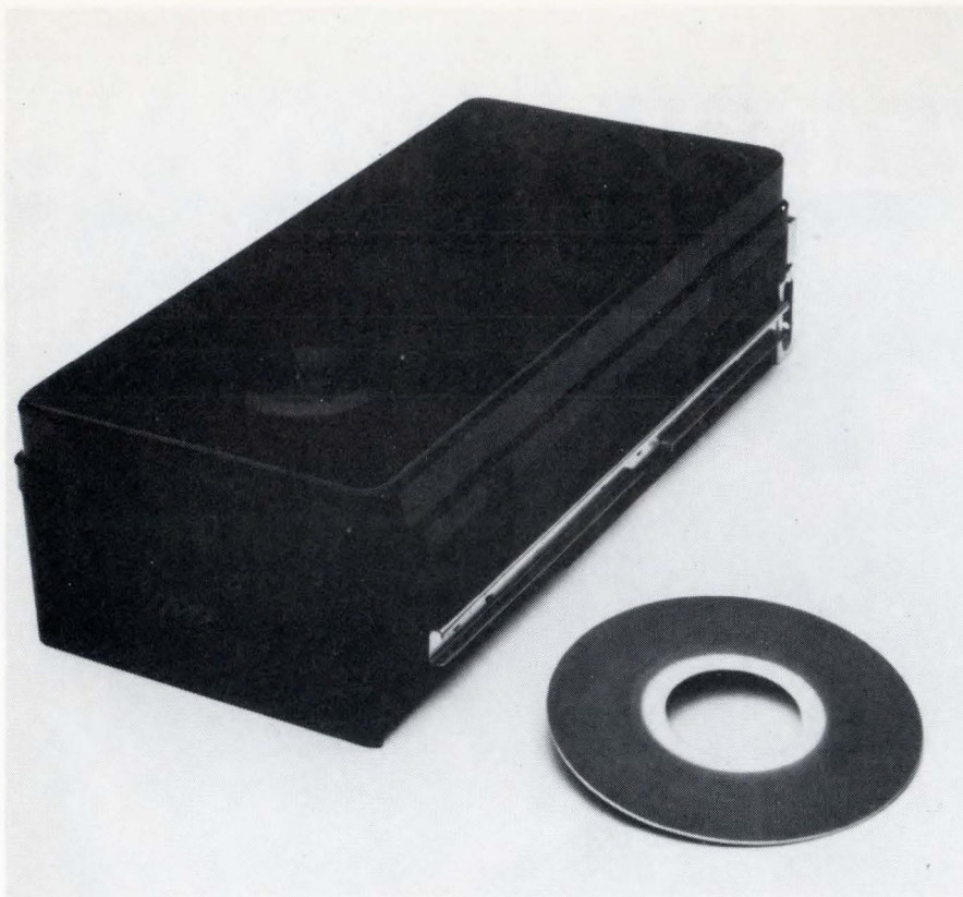
Model 7710 hard disk storage system from International Memories used two 200 mm disks and Winchester-type read/write heads positioned by a linear voice coil actuator that uses a closed loop, track-following servo system.
