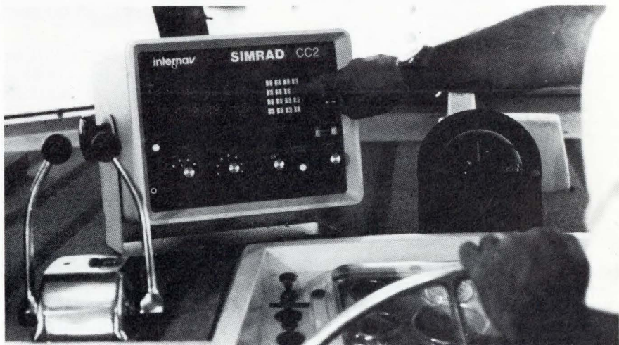
Fig 3 Internav Simrad CC-2 navigation computer includes LORAN receiver. (Courtesy of Simrad Inc., Armonk, NY).
