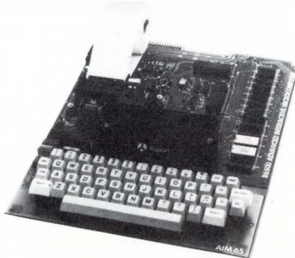
Fig 4 Rockwell AIM-65 \mu C contains a 20-character alphanumeric display and a 20-character thermal printer.
