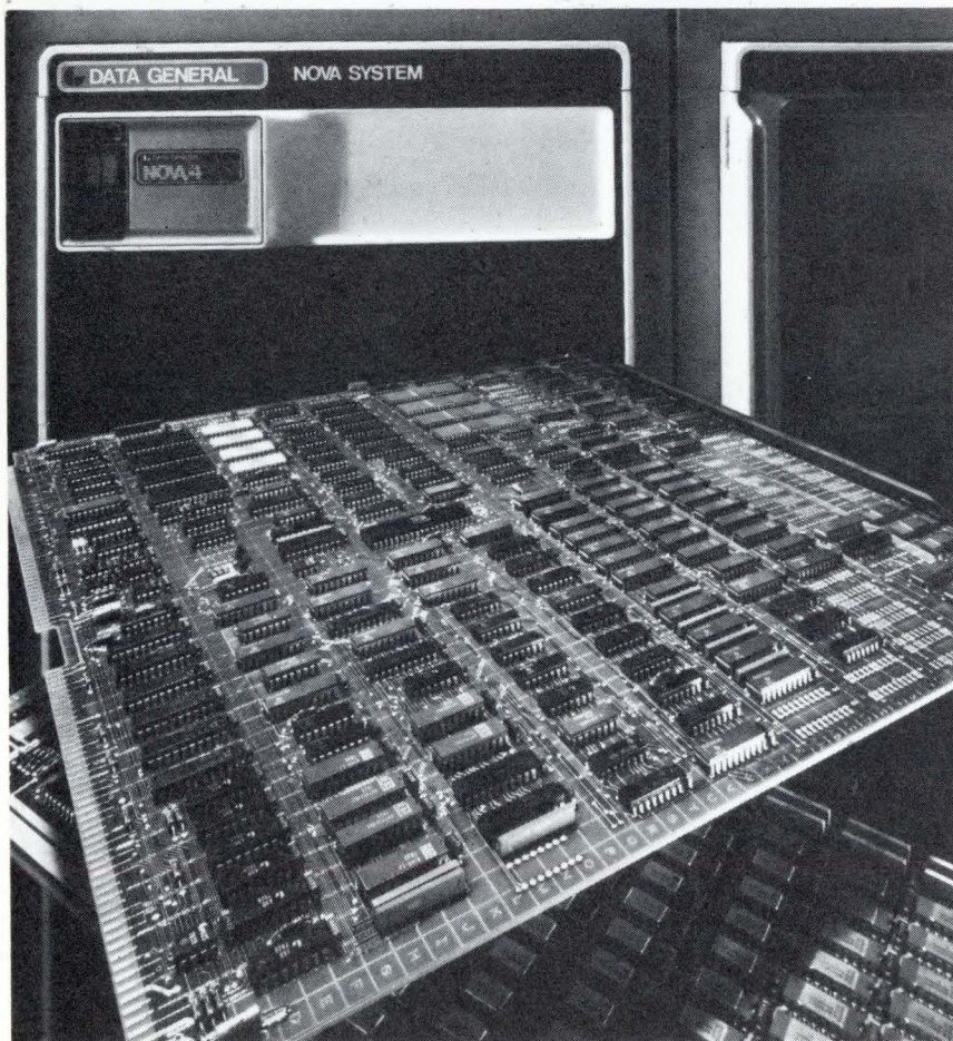
The two-board design of Data General's NOVA 4/X computer shown above incorporates CPU, MMPU, async interface, real-time clock, automatic program load, and power fail/auto restart on the CPU board, an up to 256 Kbytes on a single memory board.
