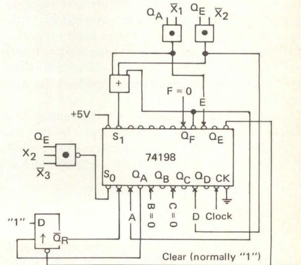
Fig 3b Sample flow diagram and state machine representing typical example of implementing — in a simple and practical way using MSI shift registers — digital sequencers for processes of relative complexity. See the sample problem in the text for equations for the above sequencer.
