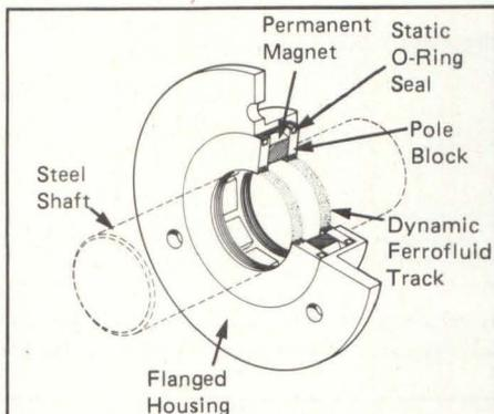
**Fig 1** Aluminum casing houses two magnetic field focusing structures separated by a ring magnet. The 0.006 -- 0.007 inch diametral gap between the drive spindle and the focus structure is filled with ferromagnetic fluid. In operation, at speeds up to 6000 rpm, liquid "O" ring Ex-seal keeps helium atmosphere free of contaminants.
