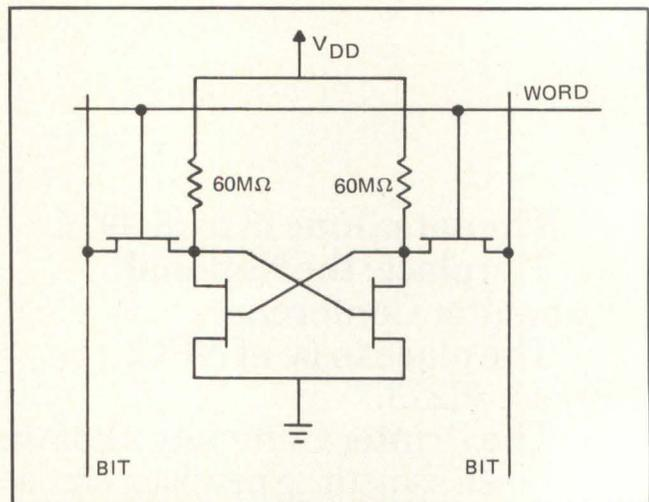
Fig 1 Static memory cell uses four transistors for the basic flip-flop and access ports. Two ion-implanted resistors serve as flip-flop loads. Depositing the resistors on top of the MOS transistors not only reduces the number of diffusions to one, but decreases the cell size considerably.
