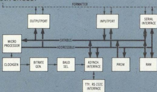
The Tandberg controller/interface is contained on one p.c. board which mounts inside the Recorder. Power is internal from the TDC 3000 built-in power supply. Two interface connectors are provided so that the Recorder can be connected both to a local I/O terminal (such as the Tandberg TDV 2100 Series CRT terminals) and a modem for remote operation.
