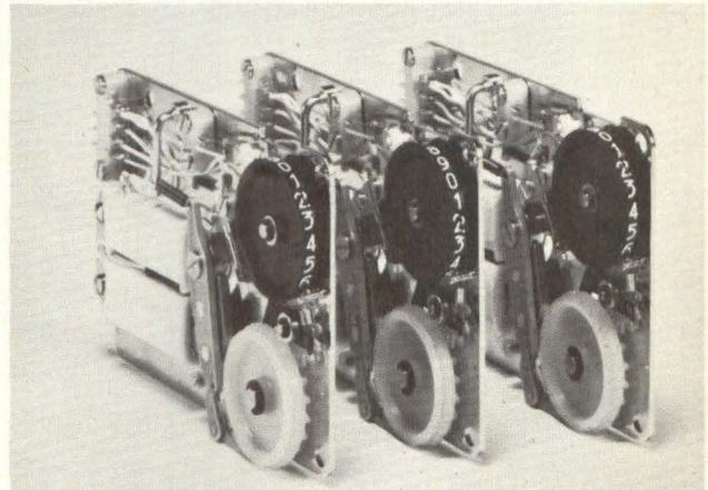
Fig 2 Wheel print mechanism has alphabetic or numeric symbols (up to 20 per wheel) arranged around each wheel's circumference. These printers are generally limited to numeric data applications and other uses requiring less than lps output.
