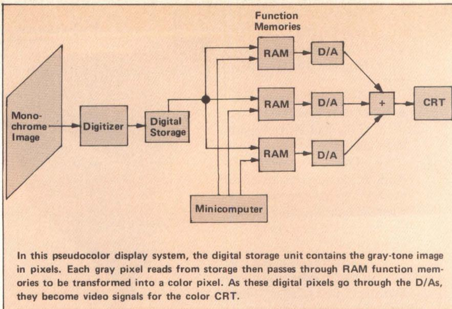
provided by the CT scanner in an 8-million bit solid state memory called refresh storage. The system then retrieves image data from this storage and processes the information through two independent, sequential processors — a function and a pseudocolor processor — before it sends it to a high resolution CRT display. Equipped with separate memories, function and pseudocolor processors perform analysis and enhancement algorithms on the refresh
