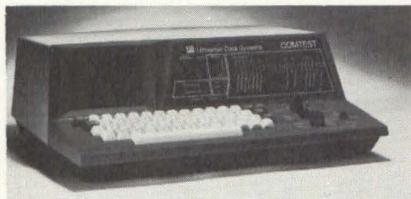
based unit from Universal Data Systems may be used in full or half duplex mode to monitor the entire system or can emulate either the CPU or various terminal devices. A 16-line, 512 character CRT display allows the dialog to be viewed at the RS232 interface. The unit has programmable search, trap, and display capability for any contiguous data string up to 16 characters. Universal Data Systems, 4900 Bradford Dr., Huntsville, AL 35805. (205) 837-8100. **Circle 216**
