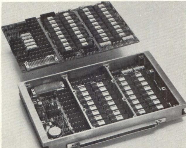
**Fig 2** Partially disassembled view shows the 9 x 4 semiconductor array and the regulator section. Timing and control electronics are packaged in the standard DIPs mounted on both surfaces.  $V_{DD}$  vs.  $V_{SX}$  shmoo plot of assembly at various interface temperatures indicates a substantial operational voltage margin for the SEMS 12 memory.
