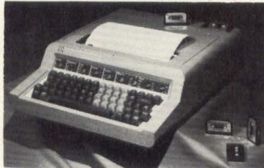
ceive capability; tape-to-tape memory, memory-to-tape, or either tape- or memory-to-line transmission. Unit features 1200 Baud transmission rates from tape, memory or keyboard to line; three-mode, operator selected keyboard including upper/lower case typewriter, TTY, APL, or integral 16 key numeric cluster; 35 character per second printing speed, fully buffered. It is compatible with all minicomputers and central processors
