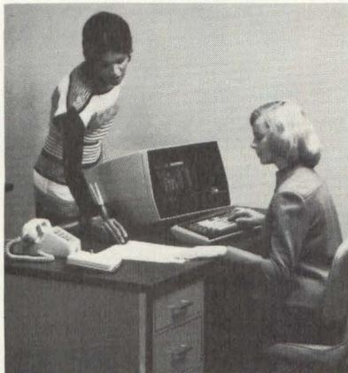
full transaction processing. Mohawk Data Sciences is initially offering two versions of its Series 21, for data entry and application processing. Basic configuration consists of an operator station with 1920 character CRT, keyboard and a processor with
