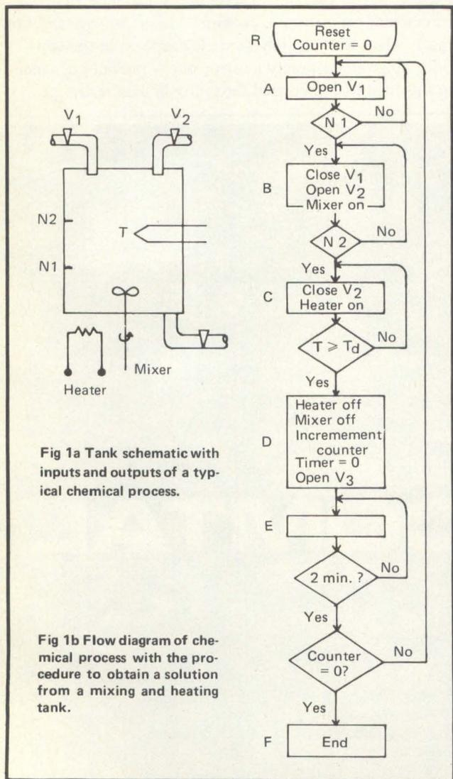
as well. We desire to repeat this process  $n$ -times, and so use a counter module- $n$ .
