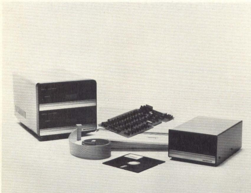
Family of integrated floppy disk systems use 5¼-inch disks and offer capacities ranging from 143 to 630 kilobytes at the price of conventional 5¼-inch disks. All four models of the MetaFloppy family are plug-compatible with most popular microcomputers.
