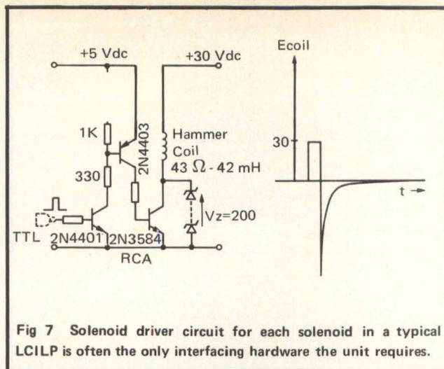
Fig 7 Solenoid driver circuit for each solenoid in a typical LCILP is often the only interfacing hardware the unit requires.
