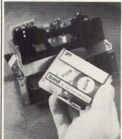
Cartridge drive using the new cartridge, in applications which require a compact unit. It stores in excess of 100,000 bytes, recording at full width, and can be battery operated. 3M Co., Mincom Div., 3M Center, Bldg. 224-BW, St. Paul, MN 55101. (612) 733-4518. **Circle 203**
