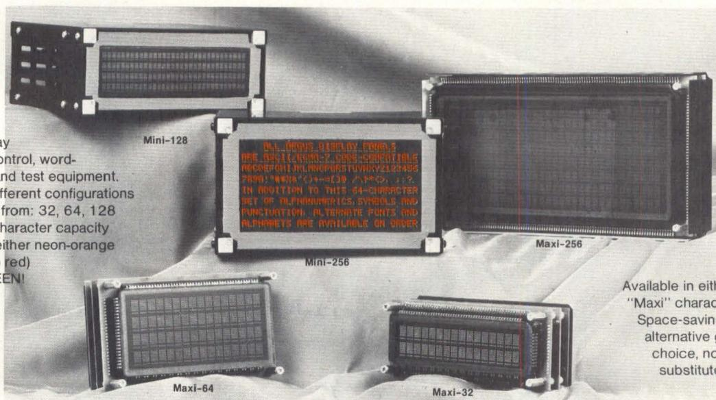
The ideal display for process control, word-processing and test equipment. Fourteen different configurations to choose from: 32, 64, 128 or 256-character capacity panels in either neon-orange (filterable to red) or NEW GREEN!
