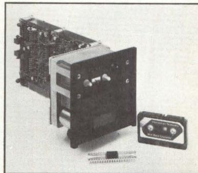
for considerations. Its small size, less than 17 cubic inches, makes the Mini-Raycorder suitable for portable terminals, desktop calculators and portable test equipment. Minimal power requirements, less than 1.5 watts at 5 volts, make it suitable for battery operation. Raymond Engineering Inc., Middletown, CT 06457, (203) 632-1000 **Circle 246**
