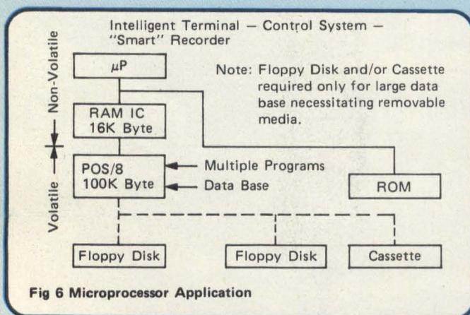
Fig 6 Microprocessor Application
