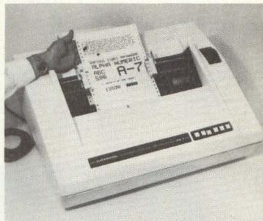
printed on either carbon or carbonless/stock, from 4-7/8" wide to standard printout size, by Dataroyal IPS-7. Print head travels with no wasted motion in this microprocessor controlled bi-directional unit to the next actual printing location. Dataroyal Inc., 235 Main Dunstable Rd., Nashua, NH 03061. (603) 883-4157. **Circle 227**
