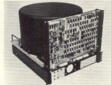
electronics for reading, writing, track selection and timing generation. The non-contact fixed head assembly can access data in an average of 8.5 milliseconds. Digital Development Corp., 8615 Balboa Ave., San Diego, CA 92123, (714) 278-9920. Circle 256
