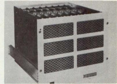
Dataram's interface is microprocessor controlled with access time ranging from 750 nanoseconds to 2.0 microseconds, depending on the system. The FHD-compatible systems have parity generate-and-check, built in off-line test capability, 0°C to 55°C operation, and operational fault indication. Dataram Corp., Princeton-Hightstown Rd., Cranbury, NJ 08512. (609) 799-0071. **Circle 202**
