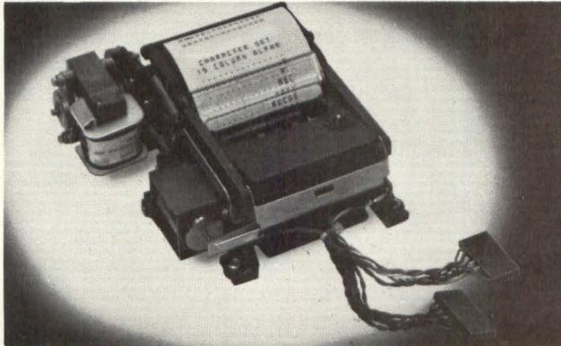
Fig 1(a) Typical solid-drum low cost impact line printer uses a line matrix to form characters by striking an inked ribbon when the desired matrix element faces the hammer. Printing occurs "on the fly," at about 3 lps. (b) Commercially available low-cost impact printer outputs 15-column lines in two colors.
