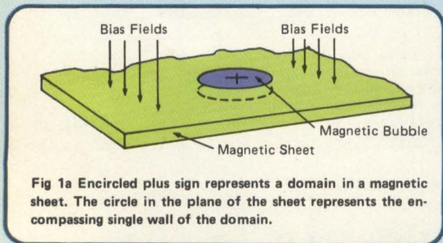
Fig 1a Encircled plus sign represents a domain in a magnetic sheet. The circle in the plane of the sheet represents the encompassing single wall of the domain.
