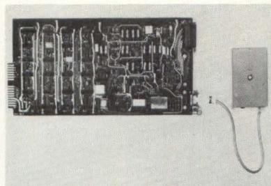
registered and is a direct replacement for the Bell system model 113B. Recent FCC rulings permit the incorporation of the data access arrangement function as an integral part of the modem if tested under FCC rules. Model VA317S enables direct electrical connection of the modem to the telephone network without externally provided telephone company data access arrangement. Unit has analog and digital loopback as well as
