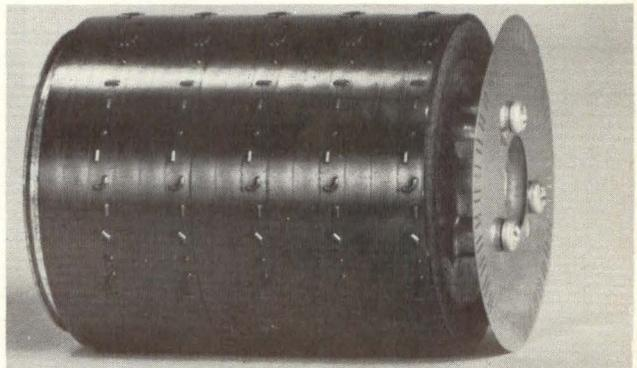
Fig 3 Solid-drum printers can output full alphanumeric data (54-character ASCII) by arranging elements of a line (bar) matrix in circumferential rows. The small drum diameter permits high-speed (1.6 lps) and fast start-up (less than 0.5 sec).
