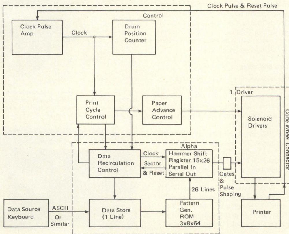
Fig 5 Simple logic is required to interface an LCILP with a data source. Patterns are generated in a ROM that can form part of the internal ROM of a microprocessor.
