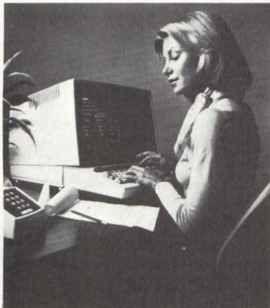
allows users with distributed operating facilities to perform data entry, data processing, file management and data communications functions, concurrently, at any local or remote site.
