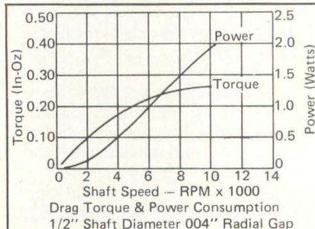
Fig 2 Combination of EX-seals and Helium atmosphere help reduce drag to conserve on energy needs for portable equipment.
