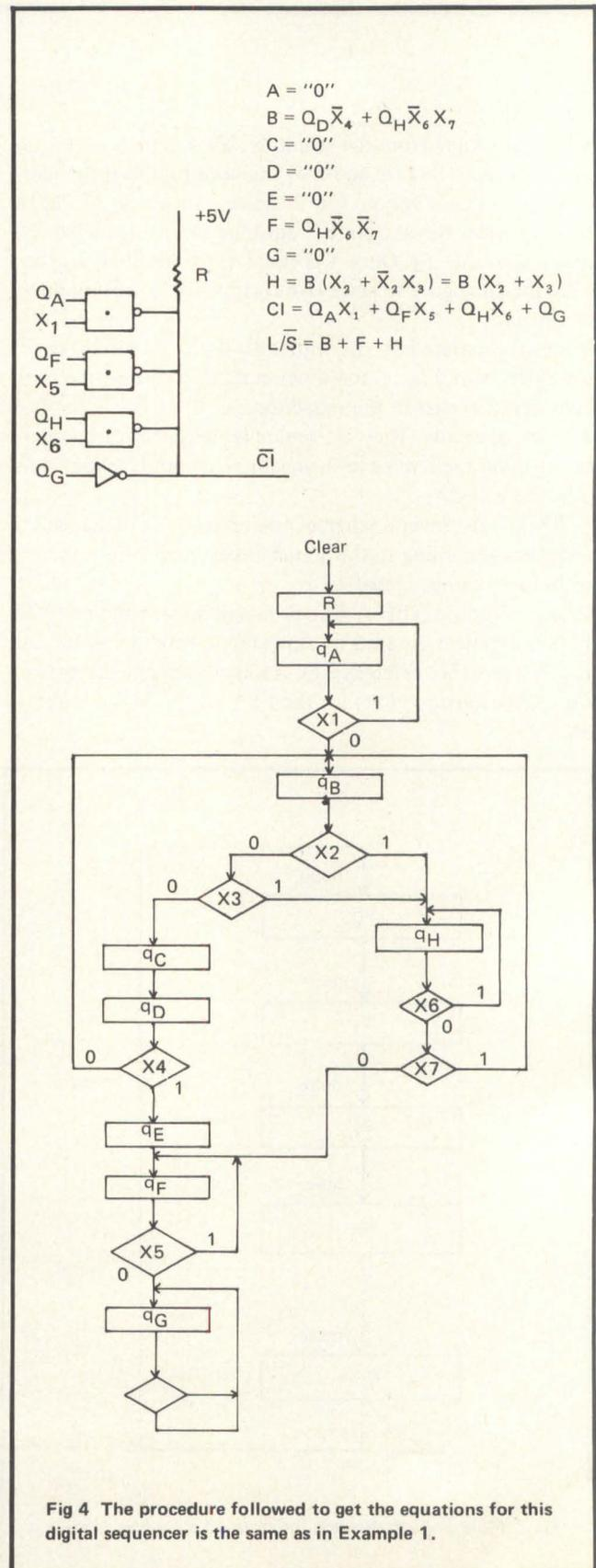
Fig 4 The procedure followed to get the equations for this digital sequencer is the same as in Example 1.
