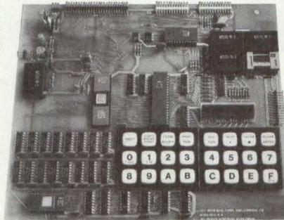
lines, 5 heavy duty relays, and Teletype and audio cassette interfaces. Plus, a 24 pad hexadecimal keyboard and a 9-digit LED hex display. All on one board.
