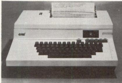
impact dot matrix printer with 5 level code, up to 30 char/sec. speed, paper tape punch and reader and an electronic editable memory of up to 8000 characters. Model B208L, an electronic KSR impact dot matrix printer with 8 level code, up to 30
