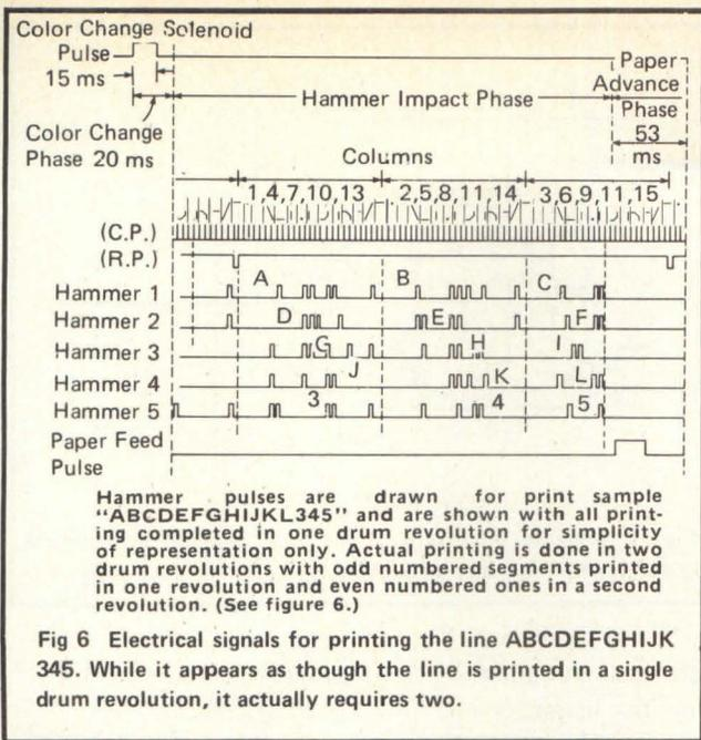
Fig 6 Electrical signals for printing the line ABCDEFGHIJK 345. While it appears as though the line is printed in a single drum revolution, it actually requires two.
