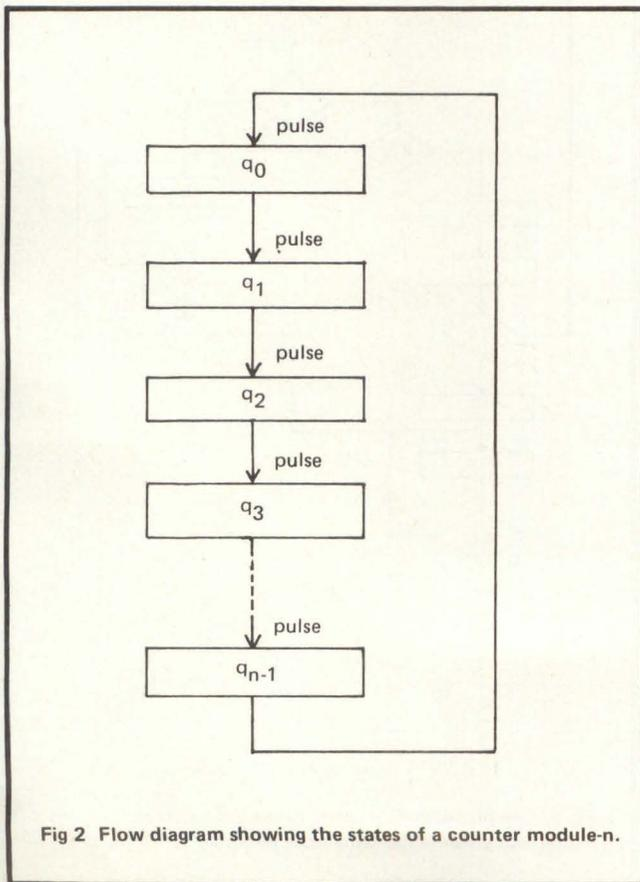
Fig 2 Flow diagram showing the states of a counter module-n.
