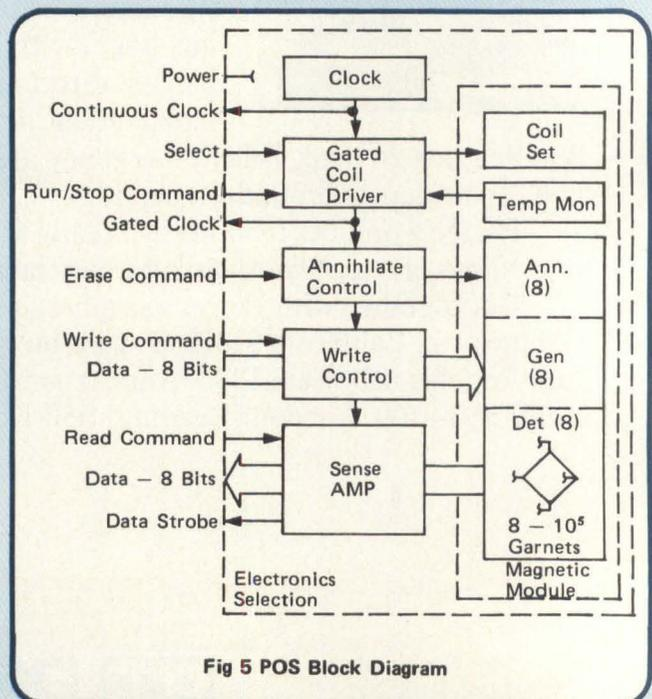
Fig 5 POS Block Diagram
