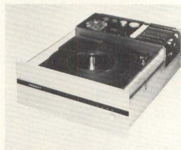
formatted capacities ranging from 14 megabytes in the single-disk version up to 70 megabytes in the three disk model. Each surface has two 350-track/inch cylinders with a recording density of 6000 bits/inch. A sealed enclosure eliminates expensive filters and blowers, yet allows operation in locations previously considered unsuitable for disk drives. Kennedy Co., 540 W. Woodbury Rd., Altadena, CA 91001, (213)798-0953.
