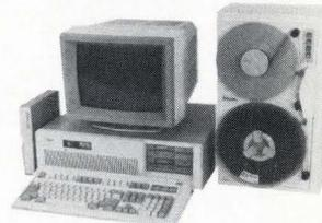
Now you can exchange data files between your IBM PC and any mainframe or mini-computer using IBM compatible 1600 or 6250 BPI 9-Track tape. System can also be used for disk backup. Transfer rate is up to 4 magabytes per minute on PCs and compatibles. Subsystems include 7" or 10½" streaming tape drive, tape coupler card and DOS compatible software. For more information, call us today!
