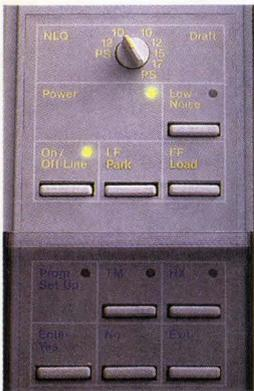
*The B-line control panel offers instant selection of print quality, font pitch, low-noise printing, etc. Set-up parameters are also controlled from the panel, thereby making the printers very easy to install.*
