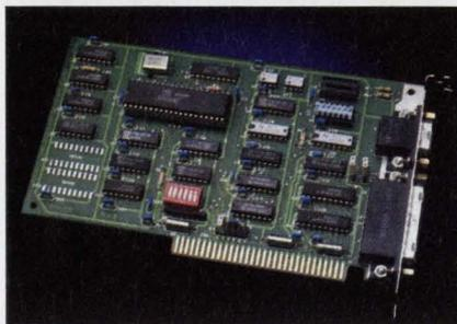
sessions, one of which can be an IBM 3287 printer emulation. ClusterNet connects to the host through an external synchronous modem, at up to 9,600bps, using either leased or switched telephone lines. It consists of a high-speed RS422 serial link and a communication protocol that supports data transmission at 19.2Kbps. ClusterNet also emulates IBM 3777 Remote Job Entry (RJE) functions to send batch jobs to the host, and to receive output directly from the host.
