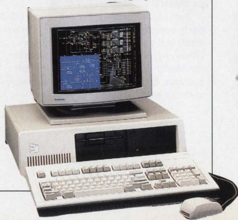
tions, which leaves the PC processor open for the application. The coprocessor has two memory banks. One is the display memory, the other is 1MB of general purpose RAM. It emulates IBM PC EGA and CGA boards, allowing compatibility with existing graphics software.
