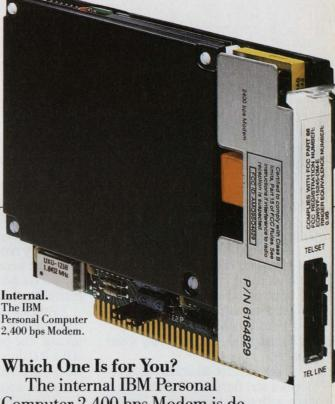
The internal IBM Personal Computer 2,400 bps Modem is designed to occupy a half slot in the IBM PC, XT, AT and 3270 PC.
