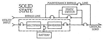
to 600 KVA. Six or more modules can be paralleled to increase ratings to 3600 KVA and beyond, building in fail-safe redundancy.
