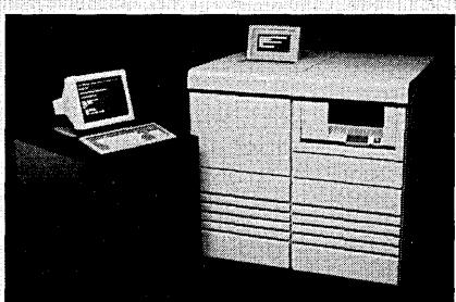
ing up to 224 users, the H 1200 utilizes 100K ECL (emitter coupled logic) and gate array circuits. The H 1200 software is compatible with the rest of the H Series. Prices for the HCX-7 start at \$225,000. The H 1200 starts at \$249,000. HARRIS CORP., Computer Systems Division, Fort Lauderdale, Fla.
