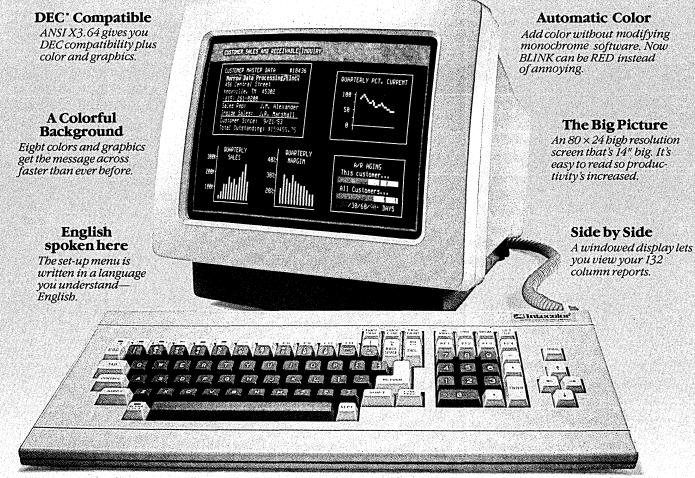
**A Custom Fit** Designed according to European standards, there's a low-profile keyboard and one-touch tilt display.
