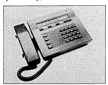
computers and data terminals can be connected via RS232C ports directly into a desktop Telenova 1 station set. The station set has a two-line, 40-character LCD display that guides users through the system and highlights only those services that are useful at a given time. A help button is built into the system with an on-line instruction manual.
