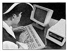
membrane panel is mounted over the face of the crt display. The membrane can sense input position with a resolution of 1 mm.
