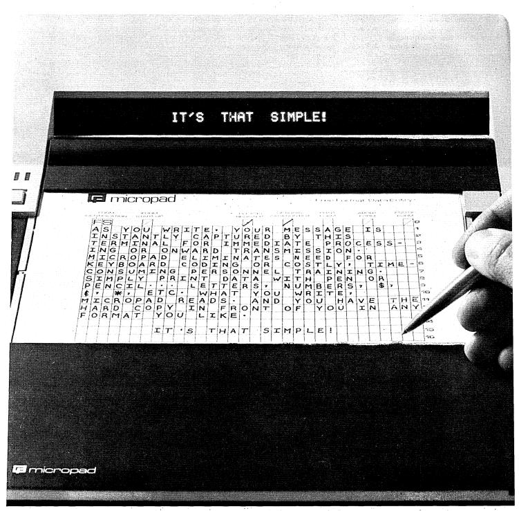
Brokers, bankers, accountants—from a factory foreman entering work in process to the chairman of the board accessing financial data—anyone can become a computer user with Micropad. Immediate feedback and data recall are provided in the integral display. Corrections are simple—just write over the character to be changed.
