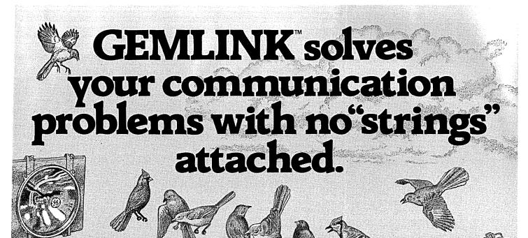
No leased wires. No modems. Or cables. That's the beauty of GEMLINK, a line-of-sight system with an effective range of up to 2.5 miles. It's an inexpensive solution to your data transmission problems that works.
