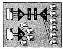
The Switch Mux allows a user to contend for any host port in either the local or remote location. Rotary group selection, speed conversion and unbalanced configurations are also standard. Costs savings are realized by reducing the number of computer ports and the size of the multiplexer configuration.
