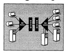
Using the advantages of statistical multiplexing, these facilities can be located thousands of miles apart.
