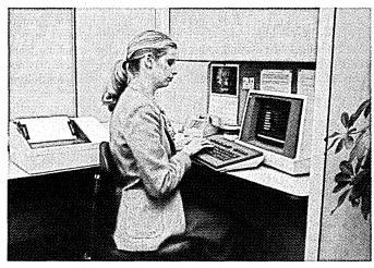
Compact 6410 matrix printers, that print at a constant 90 LPM, are available with either tractor or friction feed. The 7900 CRTs, with models that operate in block, page or character mode, are also available with either fixed or detachable keyboards.
