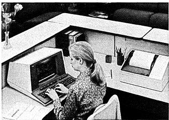
7900 display terminals weigh less than 25 lbs. Their versatile keyboards and non-glare green displays assure easy use and readability. 6425 non-impact printers silently produce hard copy at a steady 240 LPM and can print up to 99 copies under software control.
