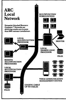
ARC networks enable workstations, processors, printers, and files to be linked together so that all resources are available to all users. Shared access brings significant economies while uniting all members of an organization with a high-speed artery for information exchange.
