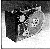
compatible with the Minifloppy line, allowing both rigid and floppy drives to interface via the same control lines. The other interfacing choice is said to be compatible with other 5.25 inch Winchesters already on the market.
