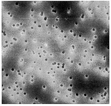
Proof positive: debris generation test with sleeves of TYVEK shows no particles on microporous filter, above. While on filter below, paper reveals considerable abrasive debris.
