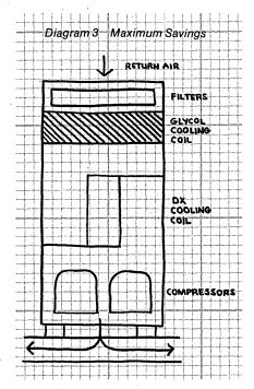
EDPAC equipment or as a retrofit to existing systems. In ten years it can save \$100,000 in a typical 3,000 sq. ft. computer room.\*
