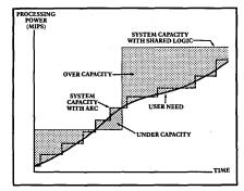
With conventional computers you can only add processing power in large, expensive steps. With ARC, you can add power in small increments, closely matching capacity to user needs.
