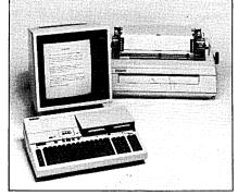
The unit also can be had with a 40 character LCD in place of the full-page display. The software-based system boots itself from diskette at power-up. With a 55cps letter quality printer and dual disk drives, the unit's pricing starts around \$9,000.
