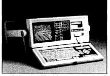
used to store and load test programs as well as capture data traffic frome the line under test.
