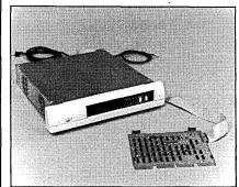
up the bandwidth, and Sytek is back with its System 40, offering higher-speed (1Mbps) channels. Intended primarily to link computers to other computers, the initial System 40 offerings interface to the Unibus used in DEC's 32-bit VAX line and the PDP-11. Standard Network Adapter Units will be compatible with Intel's Multibus.
